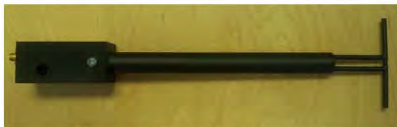
Figure 1 – MVG COMOSAR Validation Dipole
