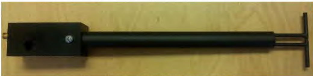
Figure 1 – MVG COMOSAR Validation Dipole
