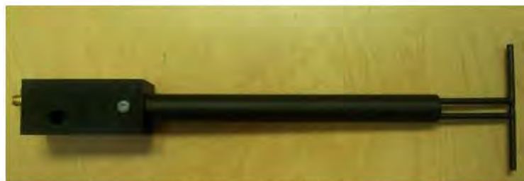
Figure 1 – MVG COMOSAR Validation Dipole
