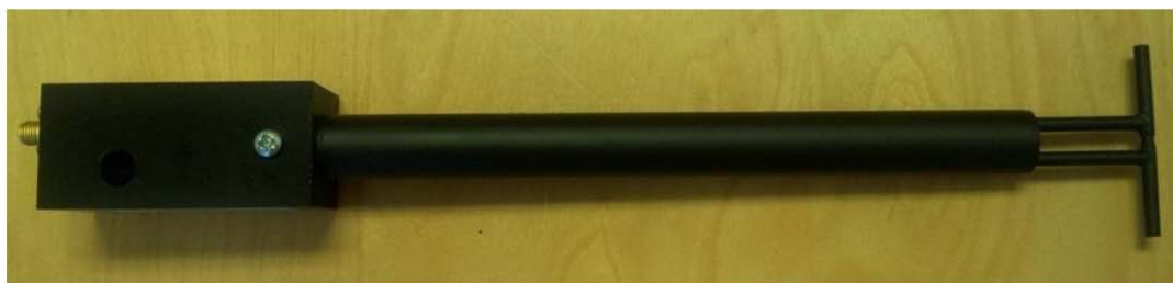
Figure 1 – MVG COMOSAR Validation Dipole
