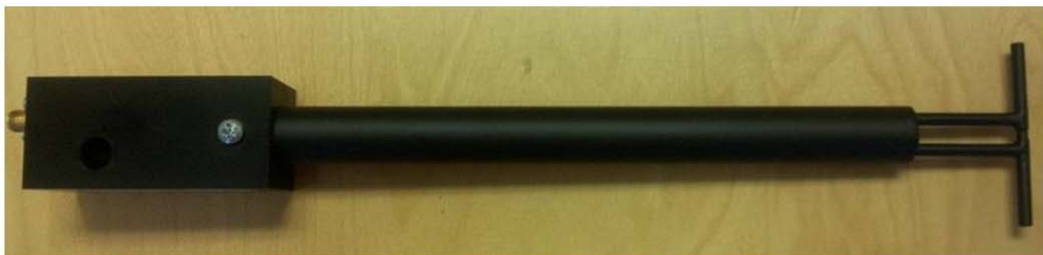
Figure 1 – MVG COMOSAR Validation Dipole
