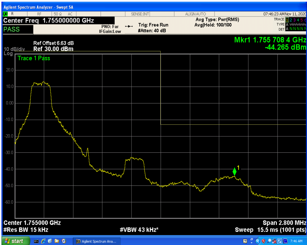
LTE Band4 QAM16 BW=1.4MHz Channel=20393 RB Size=1 Position=#Max
