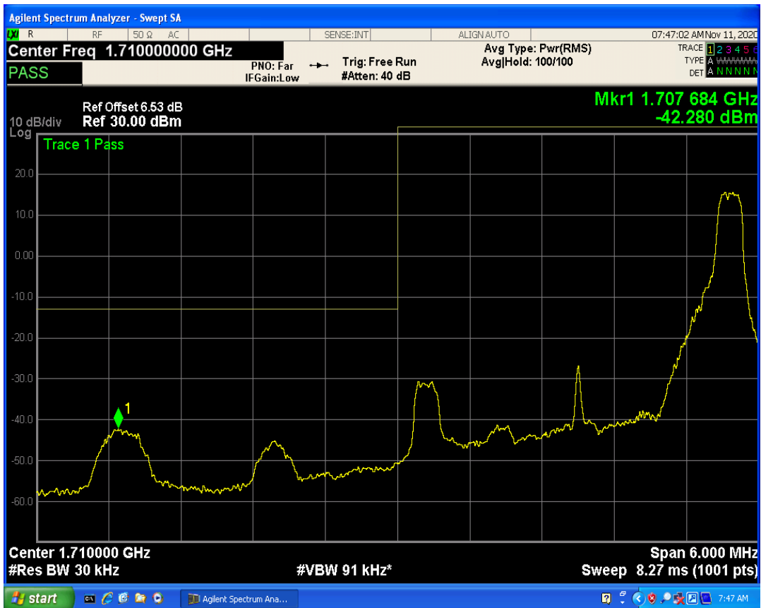
LTE Band4 QAM16 BW=3MHz Channel=19965 RB Size=15 Position=#0
