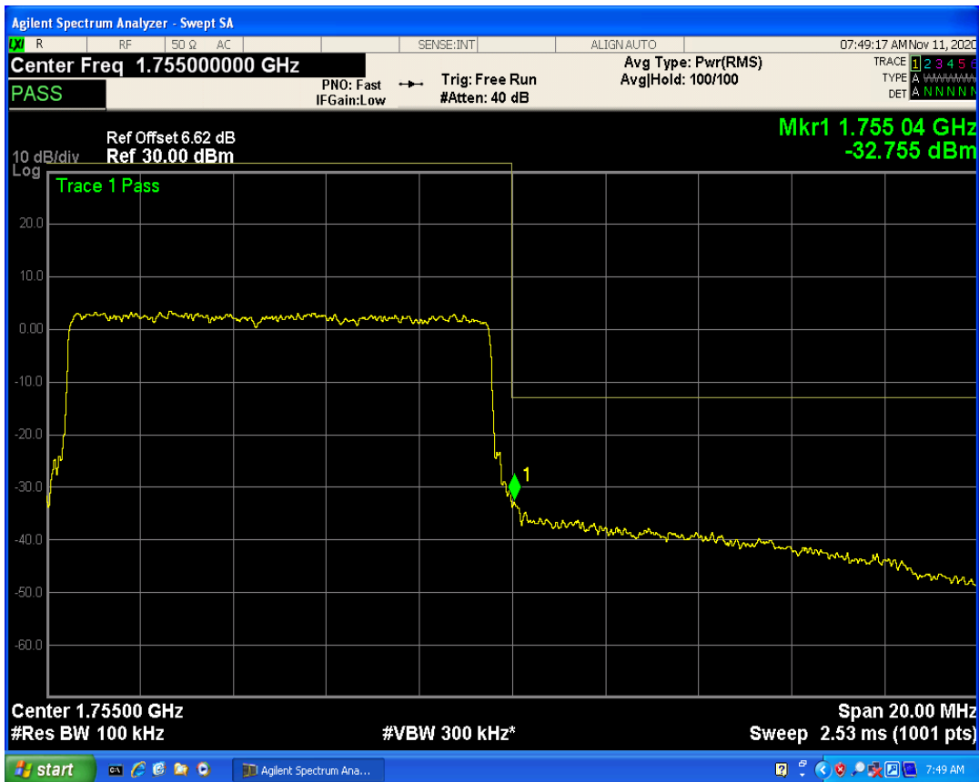
LTE Band4 QPSK BW=15MHz Channel=20025 RB Size=1 Position=#Max
