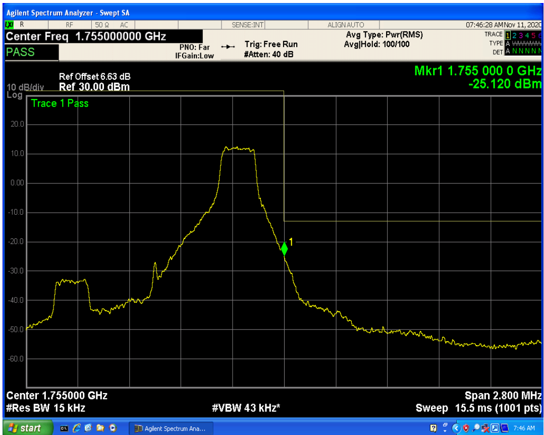
LTE Band4 QAM16 BW=1.4MHz Channel=20393 RB Size=6 Position=#0
