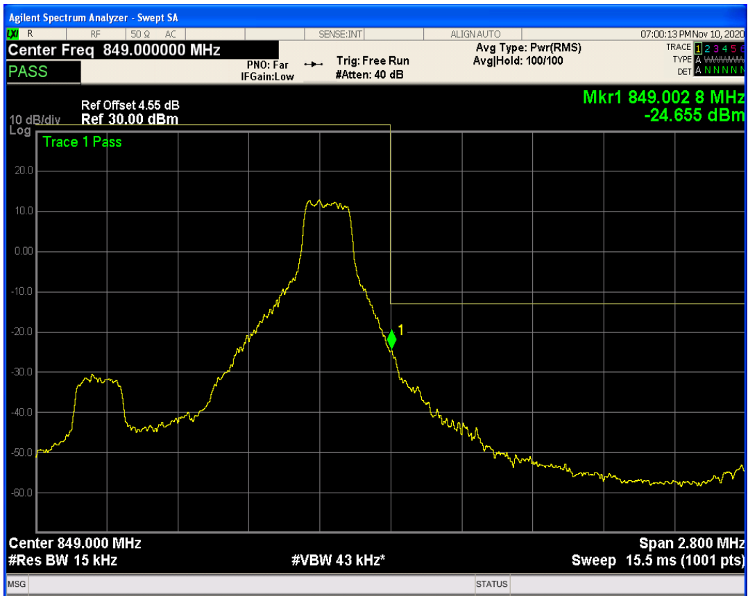
LTE Band5 QAM16 BW=1.4MHz Channel=20643 RB Size=6 Position=#0
