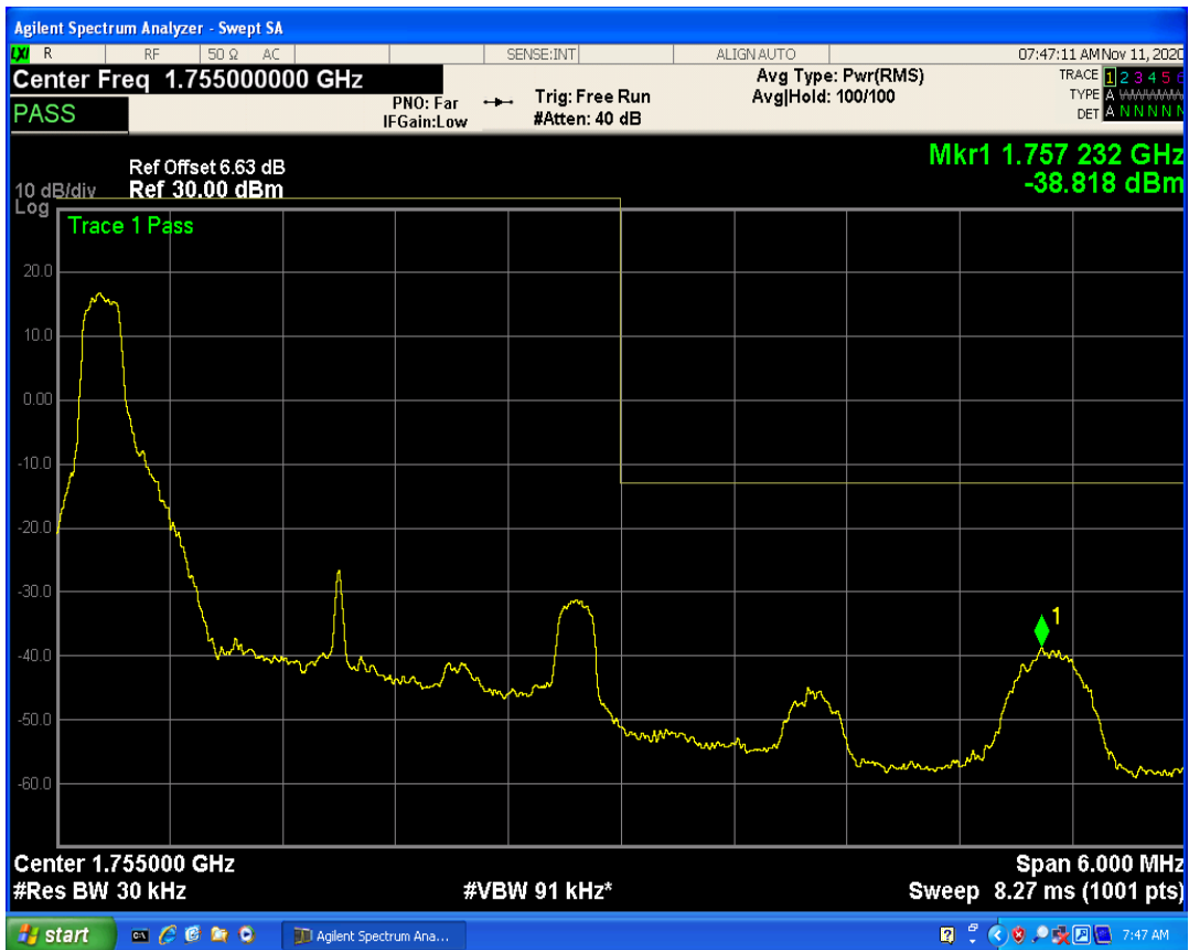
LTE Band4 QPSK BW=3MHz Channel=20385 RB Size=1 Position=#Max
