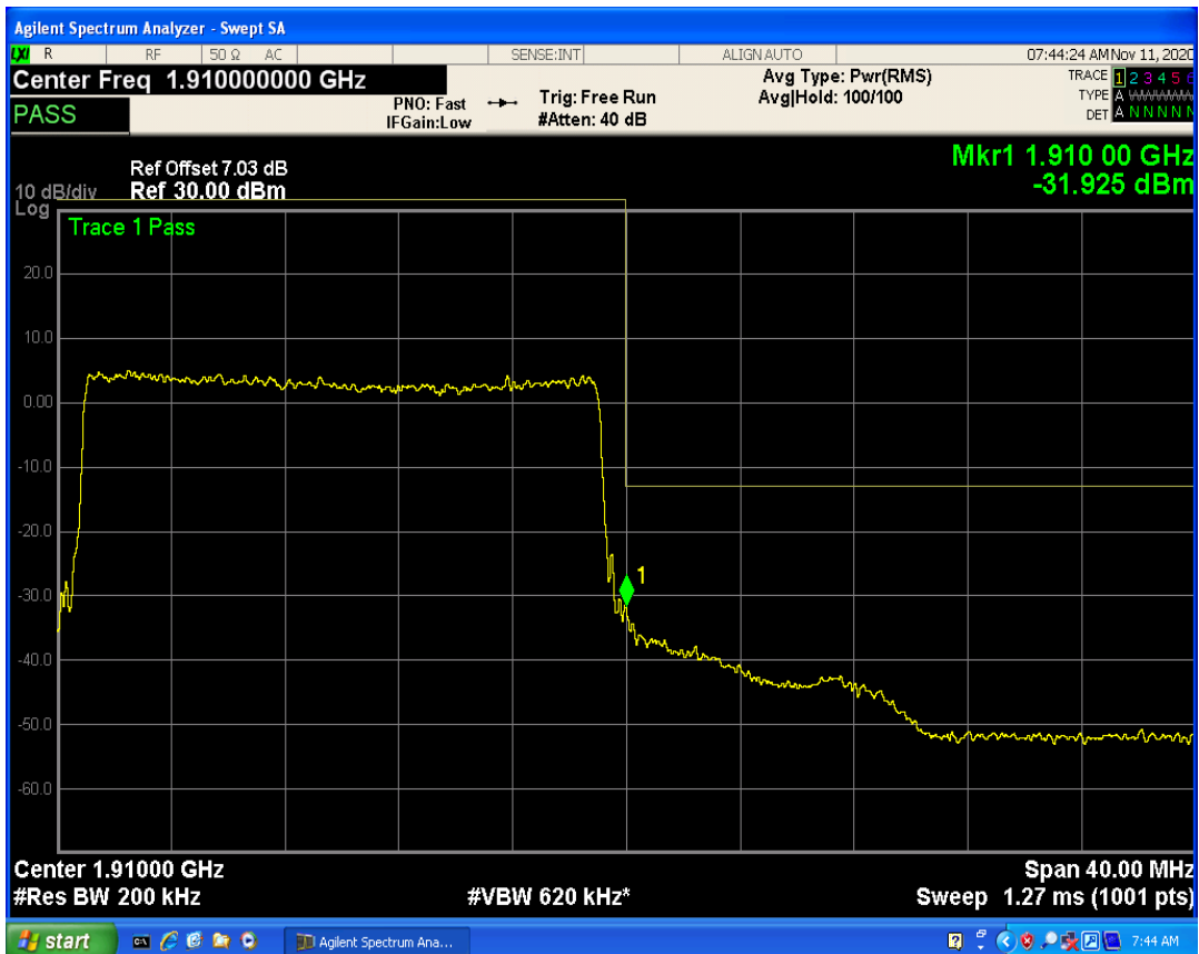
LTE Band2 QAM16 BW=20MHz Channel=19100 RB Size=1 Position=#Max
