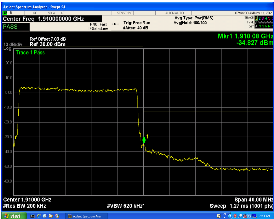
LTE Band4 QPSK BW=1.4MHz Channel=19957 RB Size=1 Position=#0
