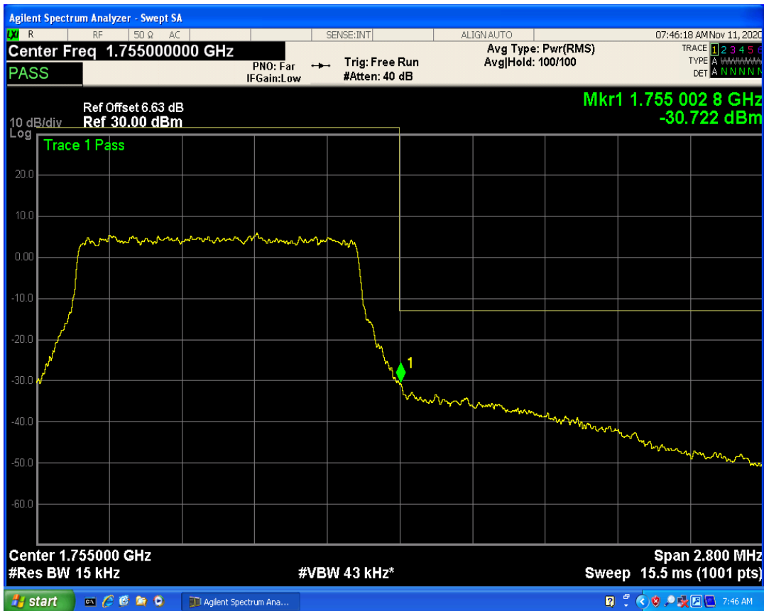
LTE Band4 QAM16 BW=1.4MHz Channel=20393 RB Size=1 Position=#0
