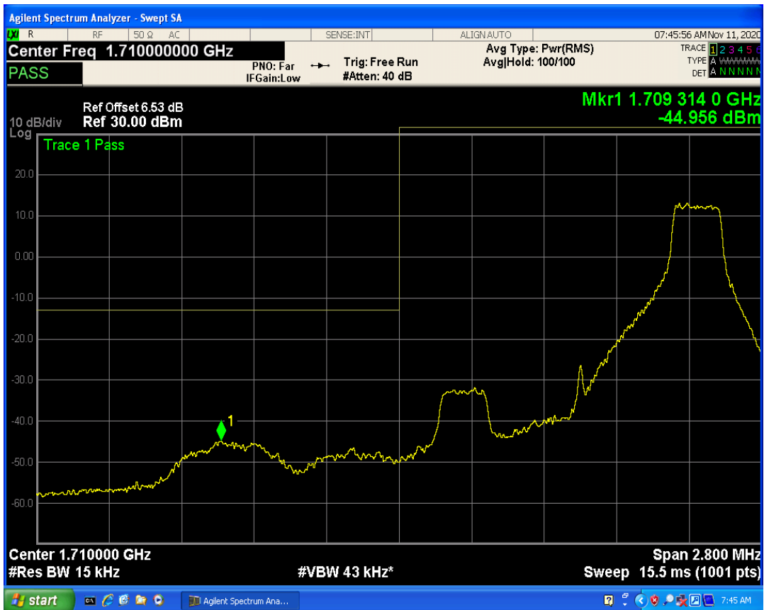
LTE Band4 QPSK BW=1.4MHz Channel=20393 RB Size=1 Position=#0
