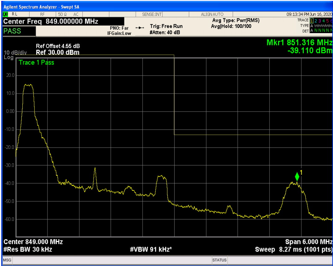
LTE Band5 QAM16 BW=3MHz Channel=20635 RB Size=1 Position=#Max
