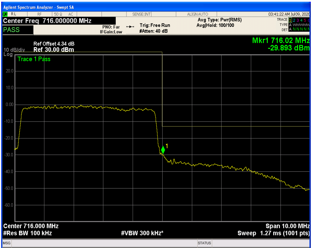
LTE Band17 QAM16 BW=5MHz Channel=23825 RB Size=1 Position=#Max
