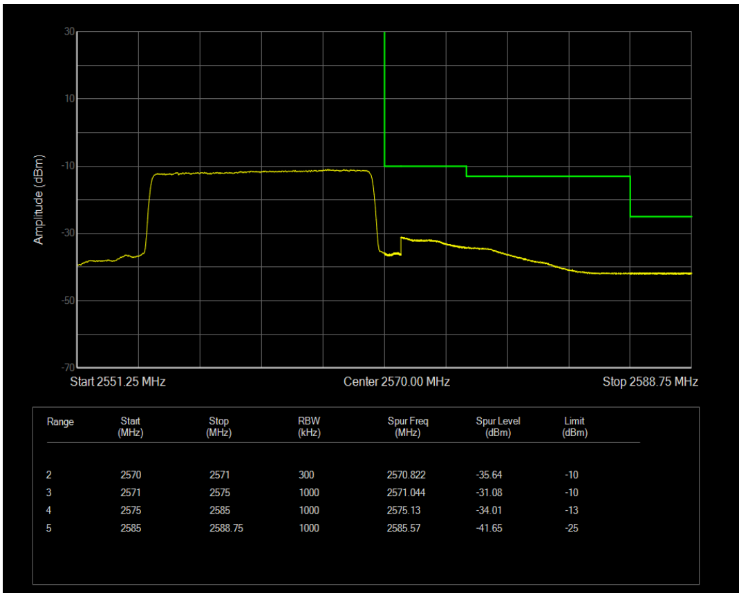
LTE Band7 QAM16 BW=15MHz Channel=21375 RB Size=1 Position=#0
