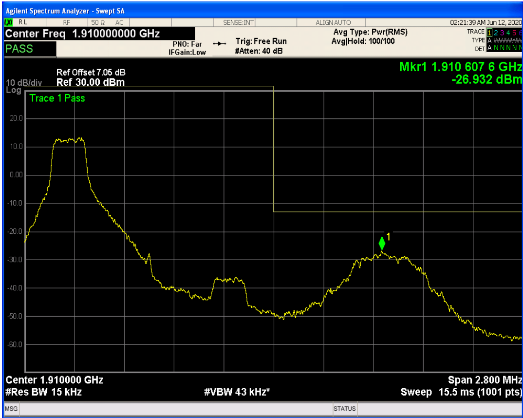
LTE Band2 QAM16 BW=1.4MHz Channel=19193 RB Size=1 Position=#Max
