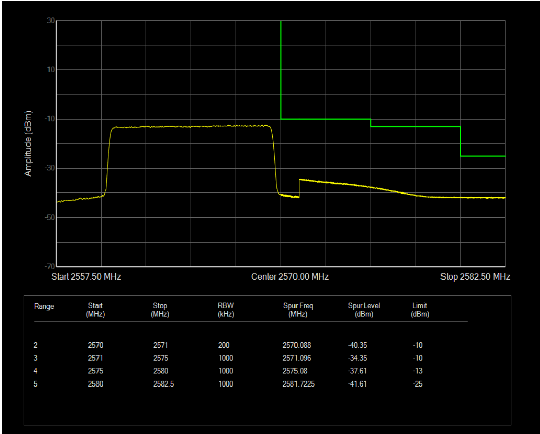
LTE Band7 QPSK BW=15MHz Channel=20825 RB Size=1 Position=#0
