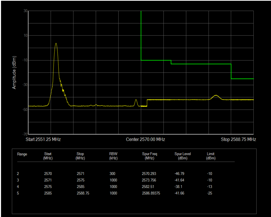
LTE Band7 QPSK BW=15MHz Channel=21375 RB Size=1 Position=#Max
