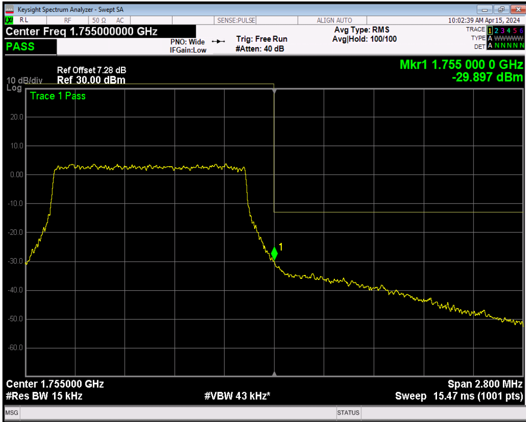
Band4 QPSK BW=3MHz Channel=19965 RB Size=1 Position=#0
