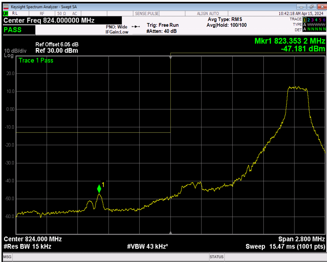
Band5 16QAM BW=1.4MHz Channel=20407 RB Size=6 Position=#0
