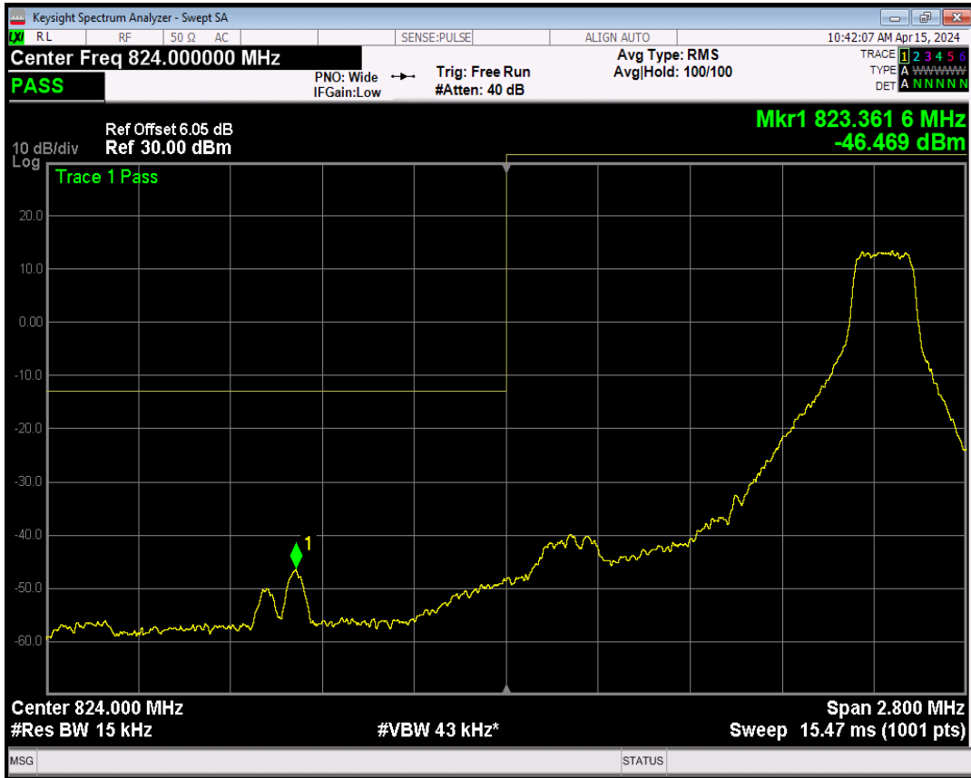
Band5 QPSK BW=1.4MHz Channel=20407 RB Size=6 Position=#0
