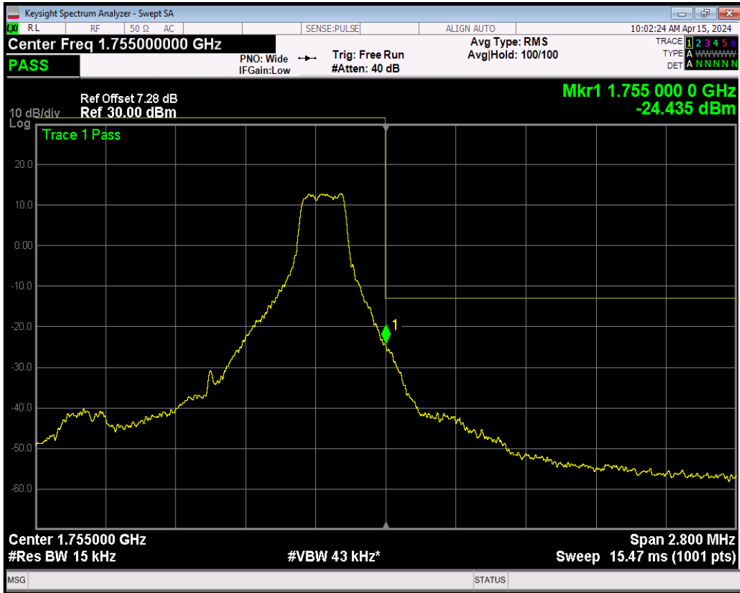
Band4 QPSK BW=1.4MHz Channel=20393 RB Size=6 Position=#0
