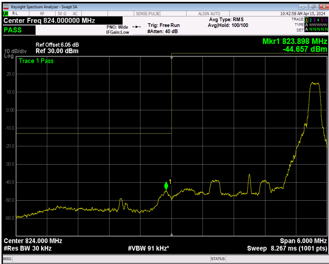
Band5 QPSK BW=3MHz Channel=20635 RB Size=1 Position=#0
