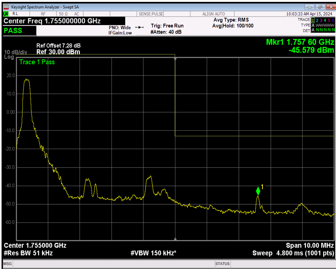
Band4 QPSK BW=5MHz Channel=20375 RB Size=1 Position=#Max
