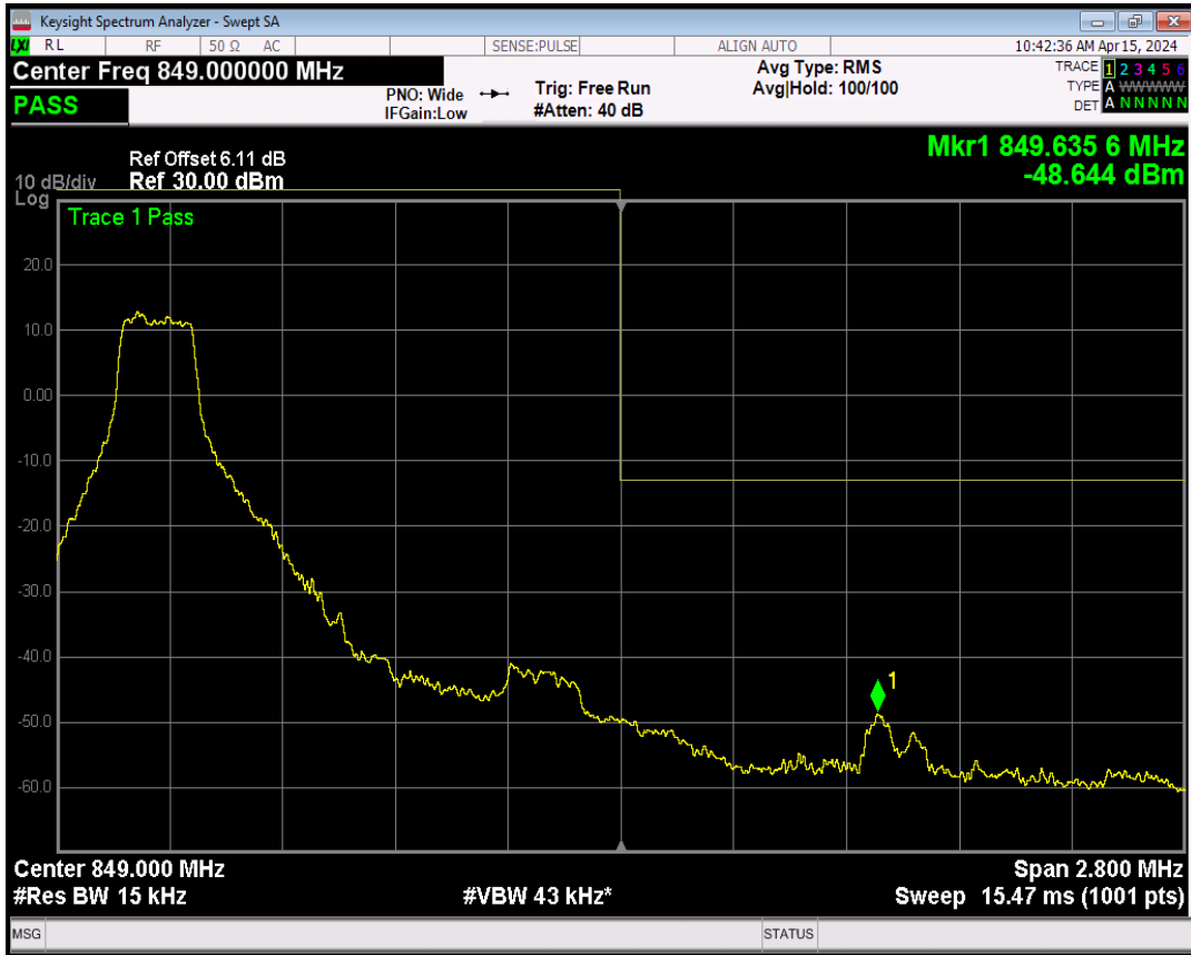
Band5 16QAM BW=1.4MHz Channel=20643 RB Size=1 Position=#Max
