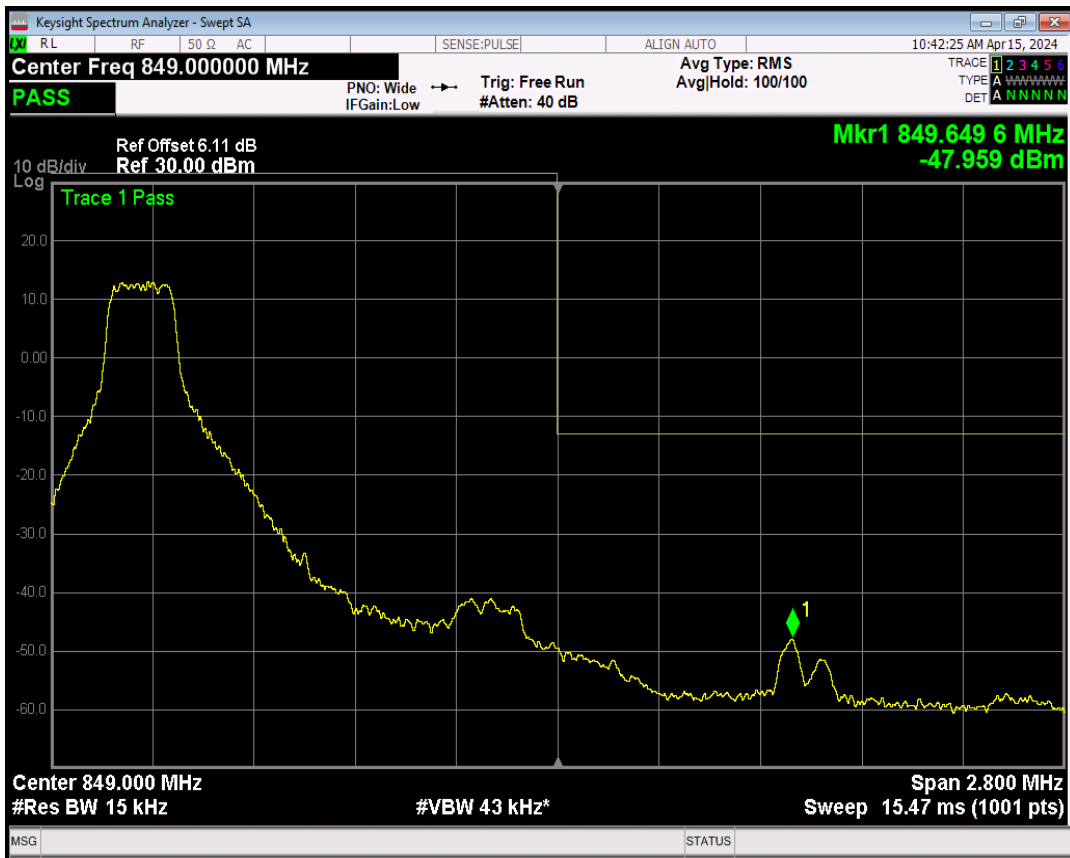
Band5 QPSK BW=1.4MHz Channel=20643 RB Size=1 Position=#Max
