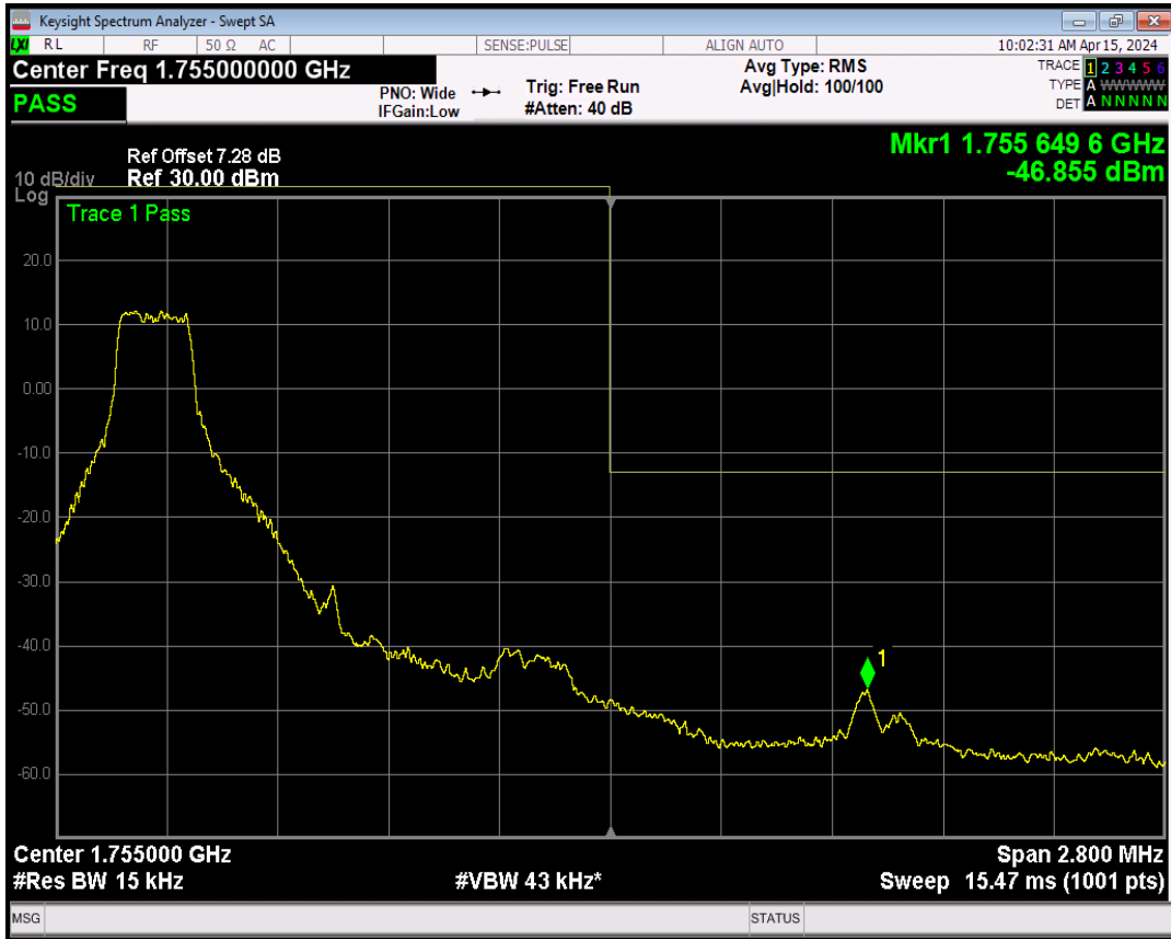
Band4 16QAM BW=1.4MHz Channel=20393 RB Size=1 Position=#Max
