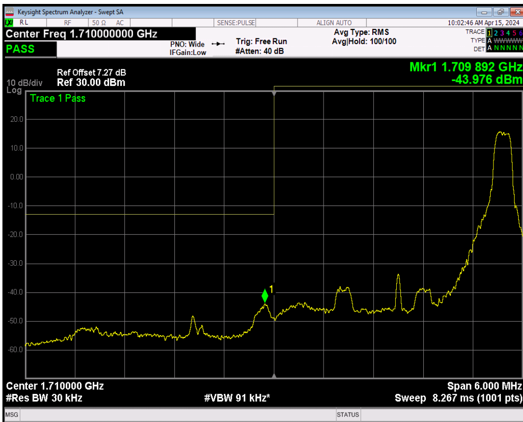
Band4 QPSK BW=3MHz Channel=19965 RB Size=15 Position=#0
