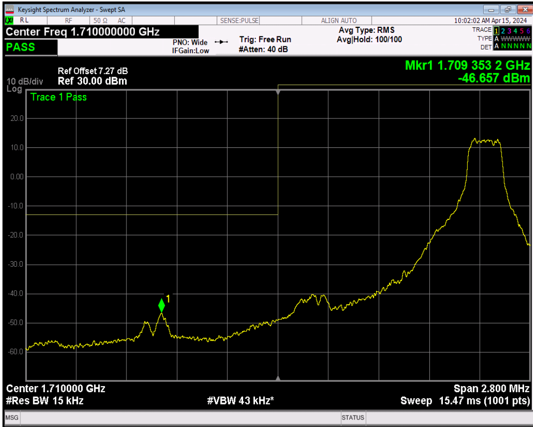
Band4 QPSK BW=1.4MHz Channel=19957 RB Size=6 Position=#0
