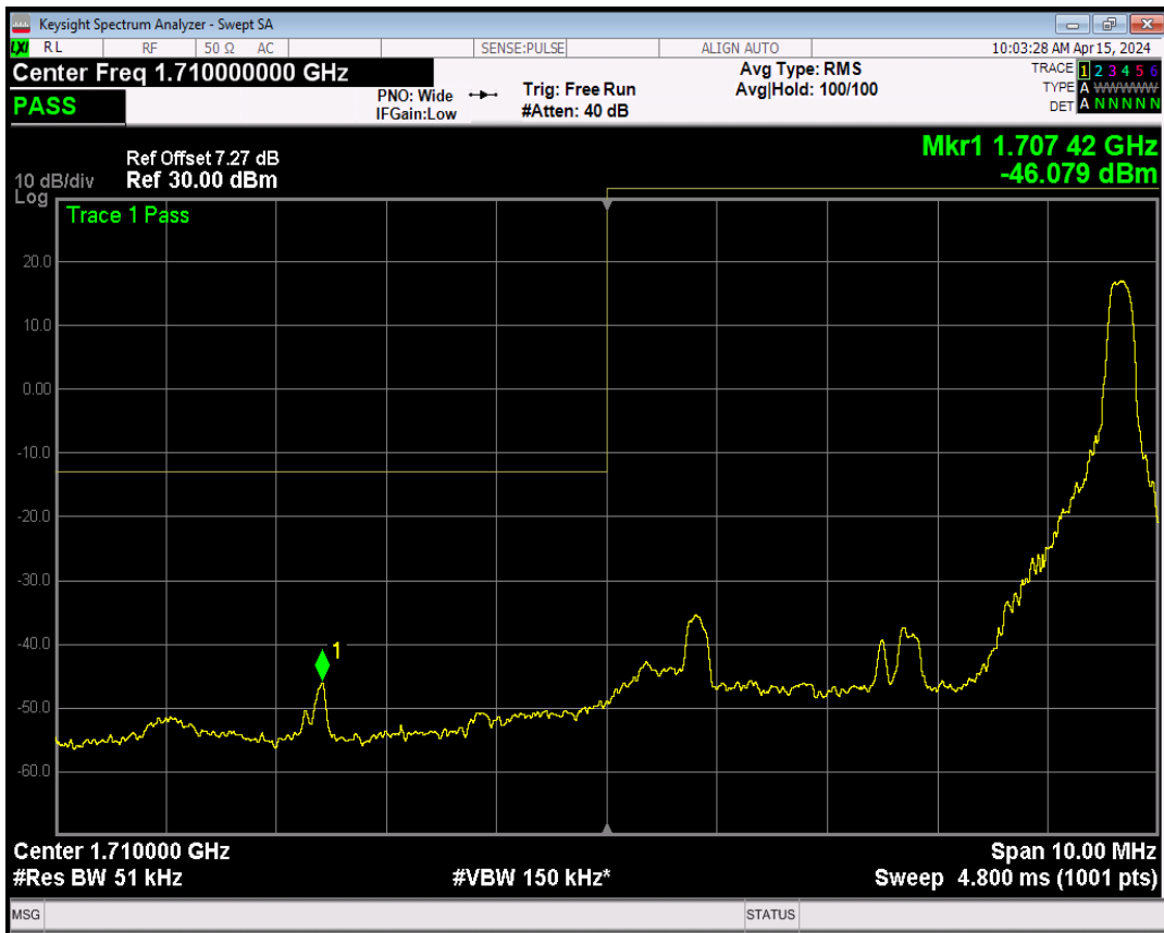
Band4 16QAM BW=5MHz Channel=19975 RB Size=25 Position=#0
