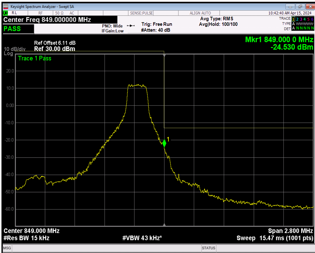
Band5 16QAM BW=1.4MHz Channel=20643 RB Size=6 Position=#0
