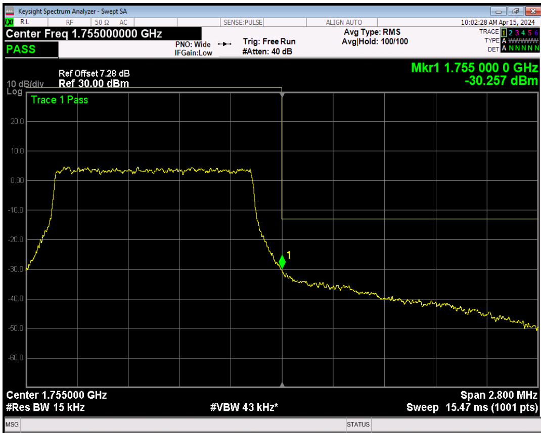
Band4 16QAM BW=1.4MHz Channel=20393 RB Size=1 Position=#0
