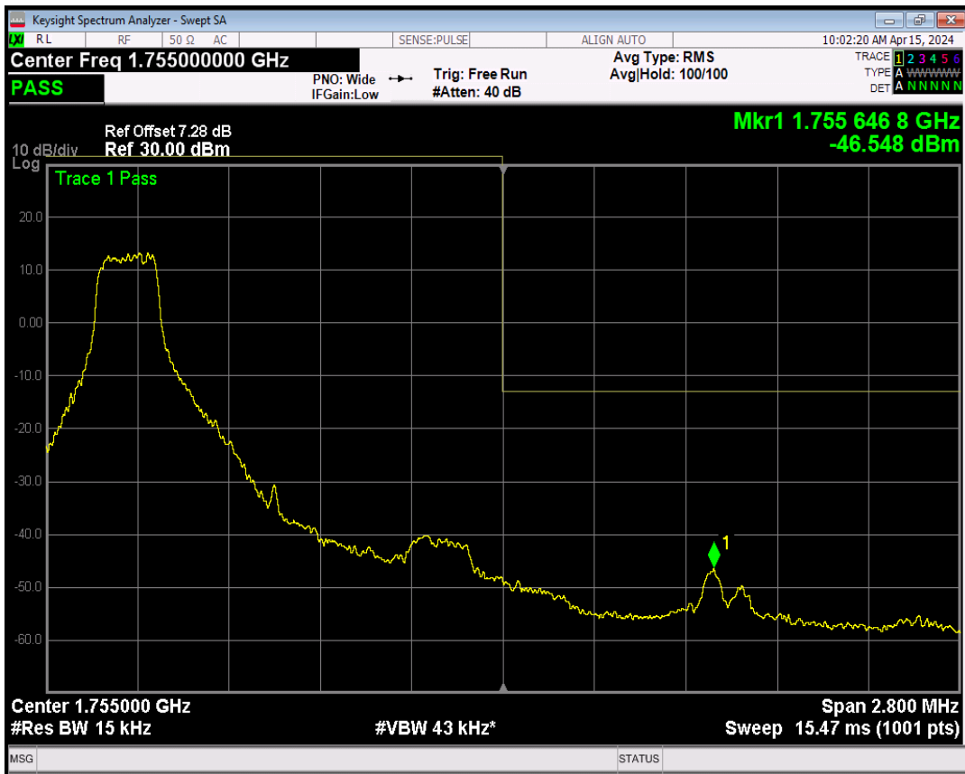
Band4 QPSK BW=1.4MHz Channel=20393 RB Size=1 Position=#Max
