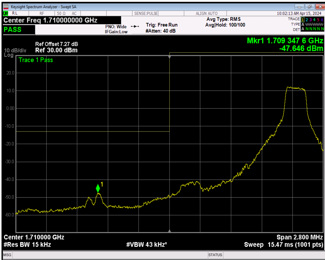
Band4 16QAM BW=1.4MHz Channel=19957 RB Size=6 Position=#0
