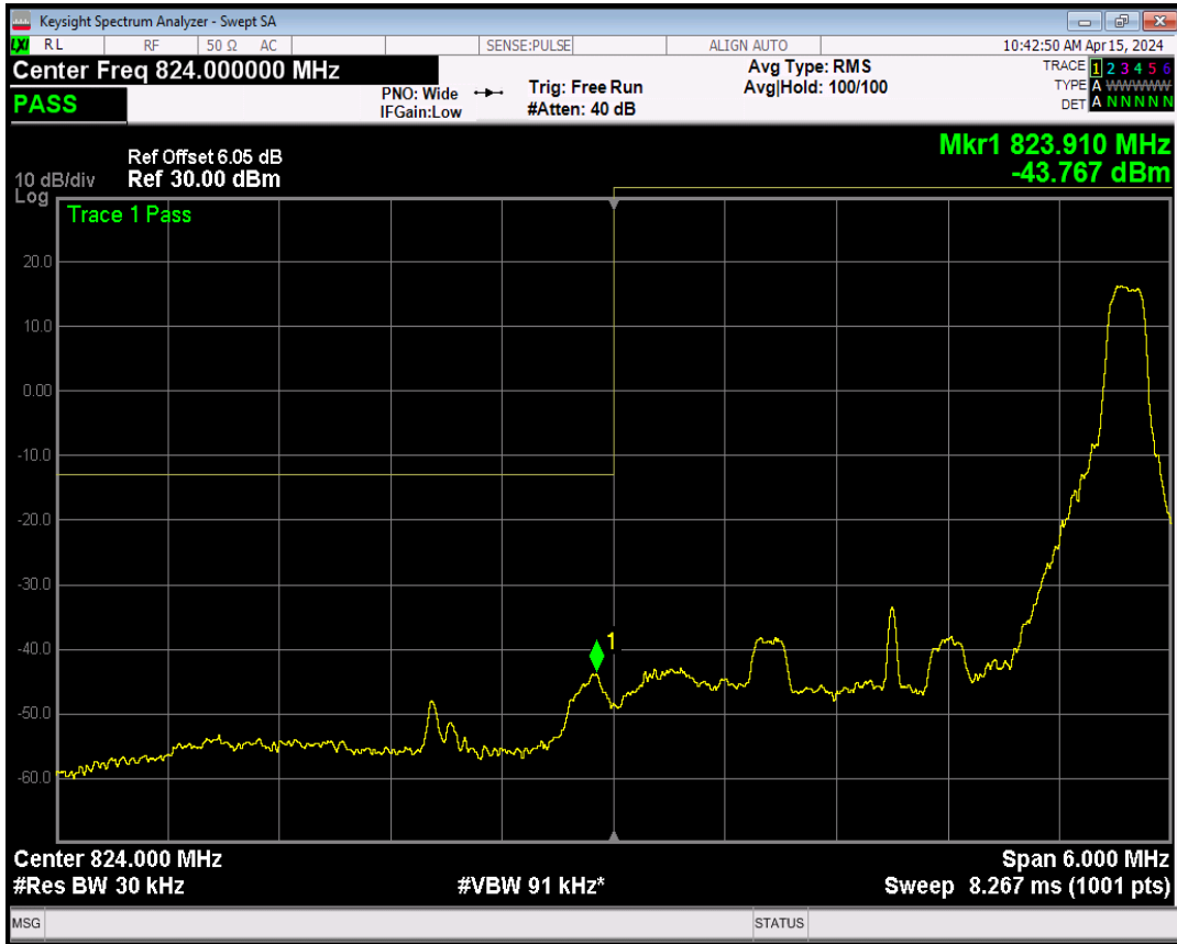
Band5 QPSK BW=3MHz Channel=20415 RB Size=15 Position=#0
