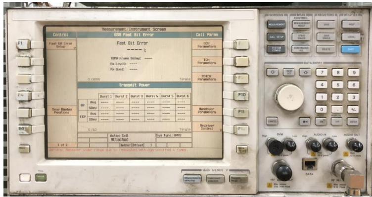
Agilent 8960 (2G/3GTest Equipment)
