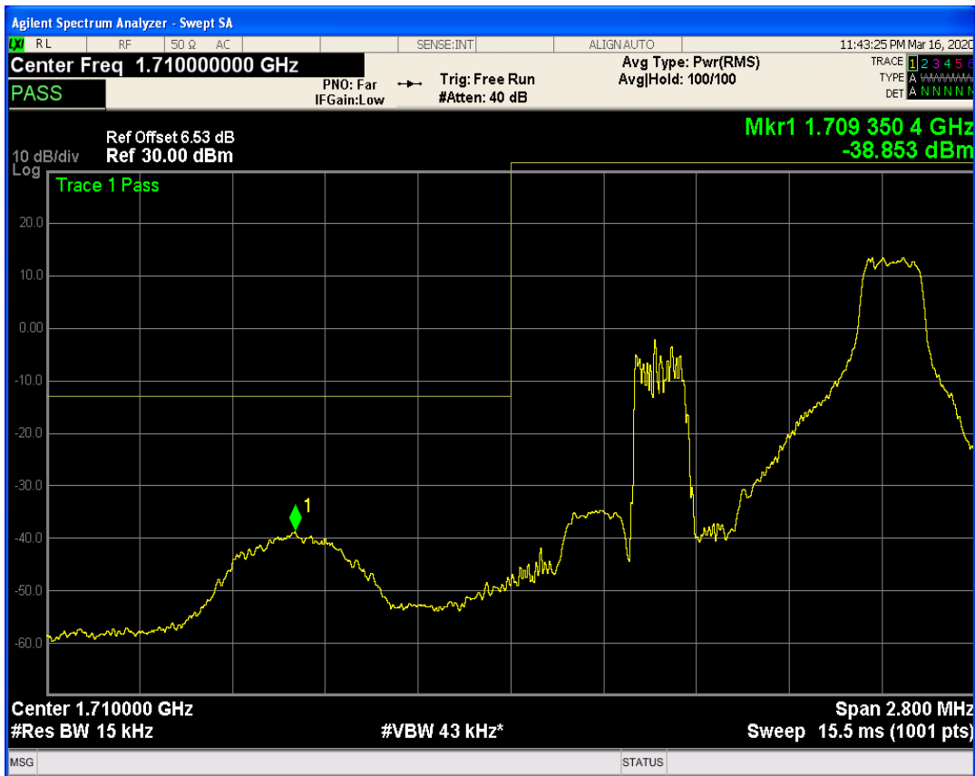
LTE Band4 QPSK BW=1.4MHz Channel=19957 RB Size=6 Position=#0
