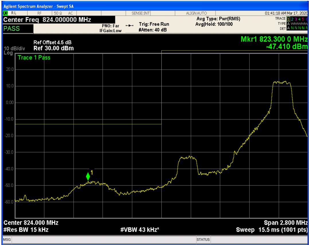
LTE Band5 QPSK BW=1.4MHz Channel=20643 RB Size=1 Position=#0
