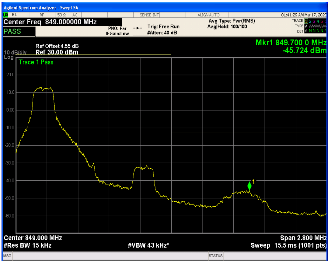
LTE Band5 QPSK BW=1.4MHz Channel=20643 RB Size=1 Position=#Max
