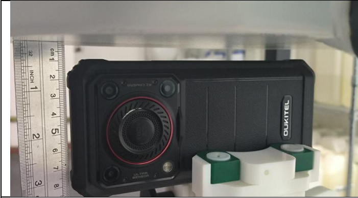
Top Side (Separation distance of 10mm)
