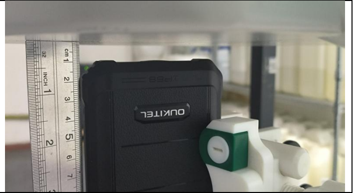
Bottom Side (Separation distance of 10mm)
