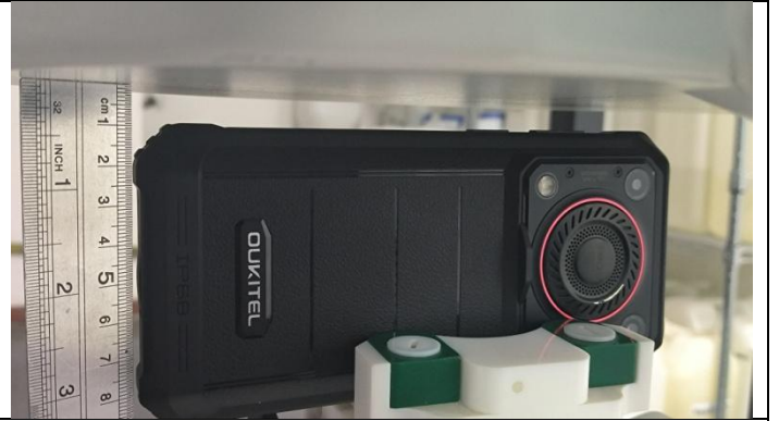
Bottom Side (Separation distance of 10mm)
