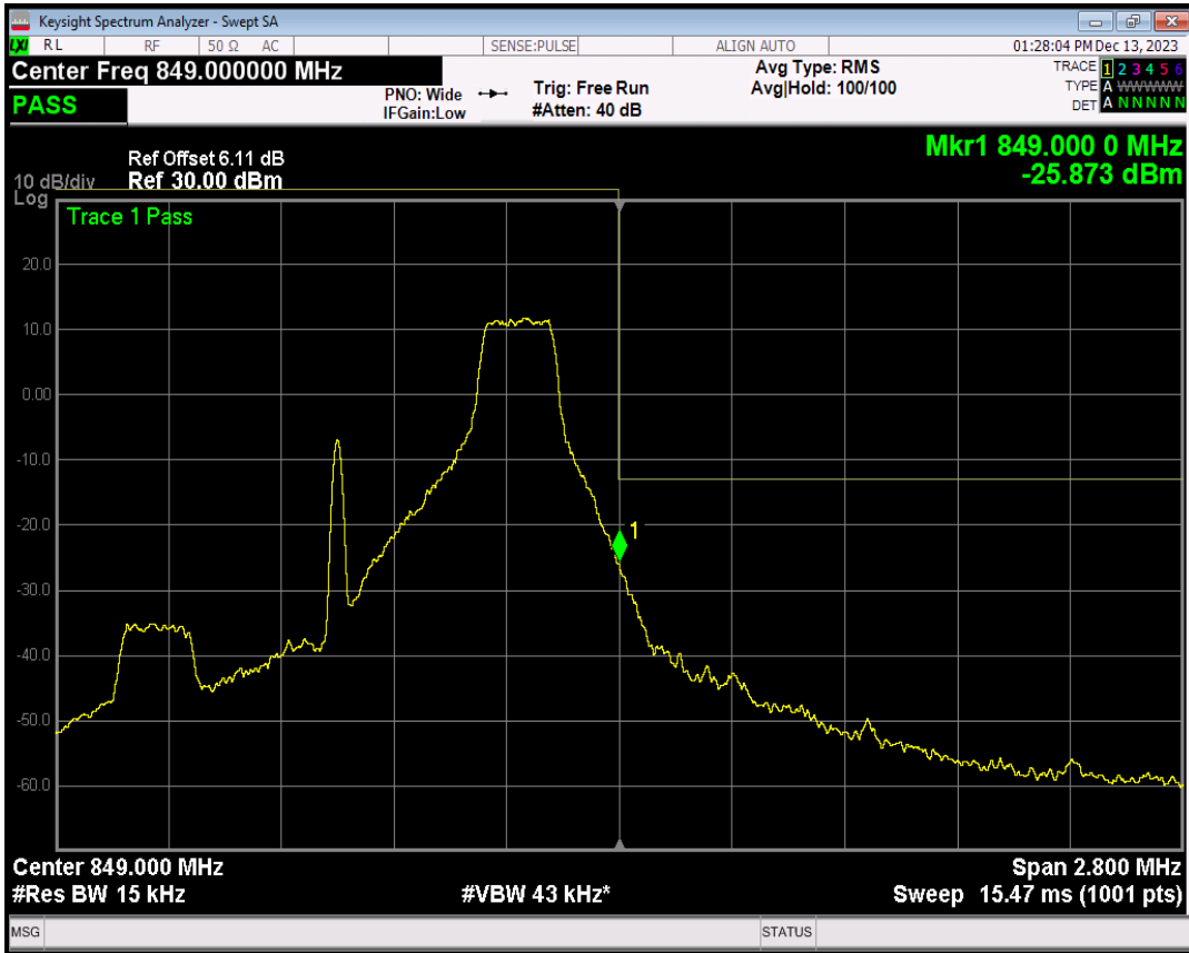
Band5 QPSK BW=1.4MHz Channel=20643 RB Size=6 Position=#0
