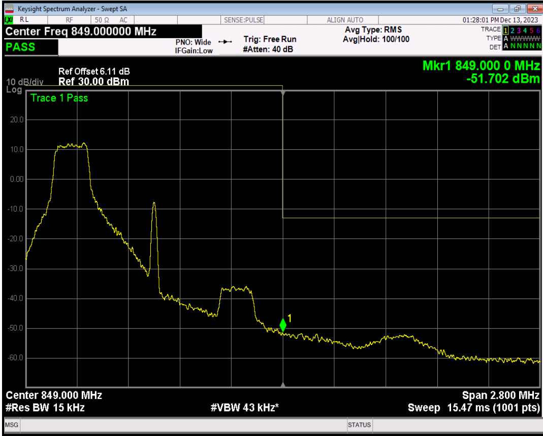
Band5 QPSK BW=1.4MHz Channel=20643 RB Size=1 Position=#Max
