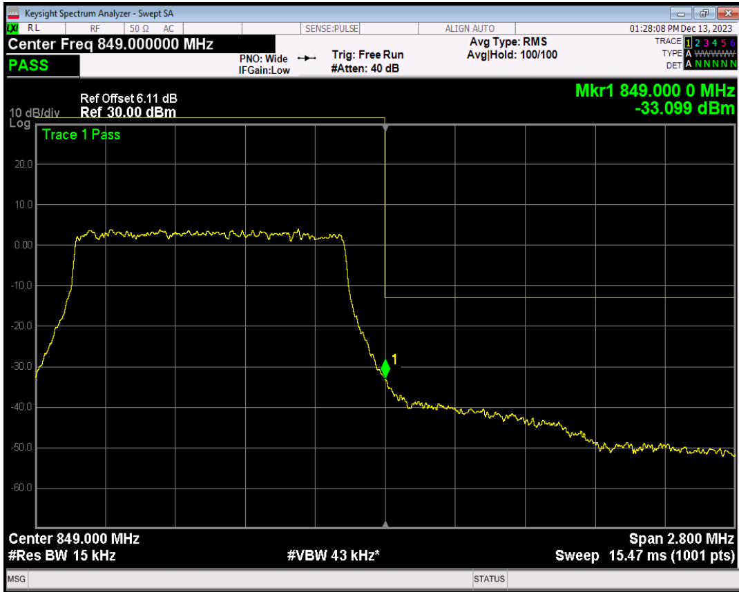
Band5 QPSK BW=10MHz Channel=20450 RB Size=1 Position=#0
