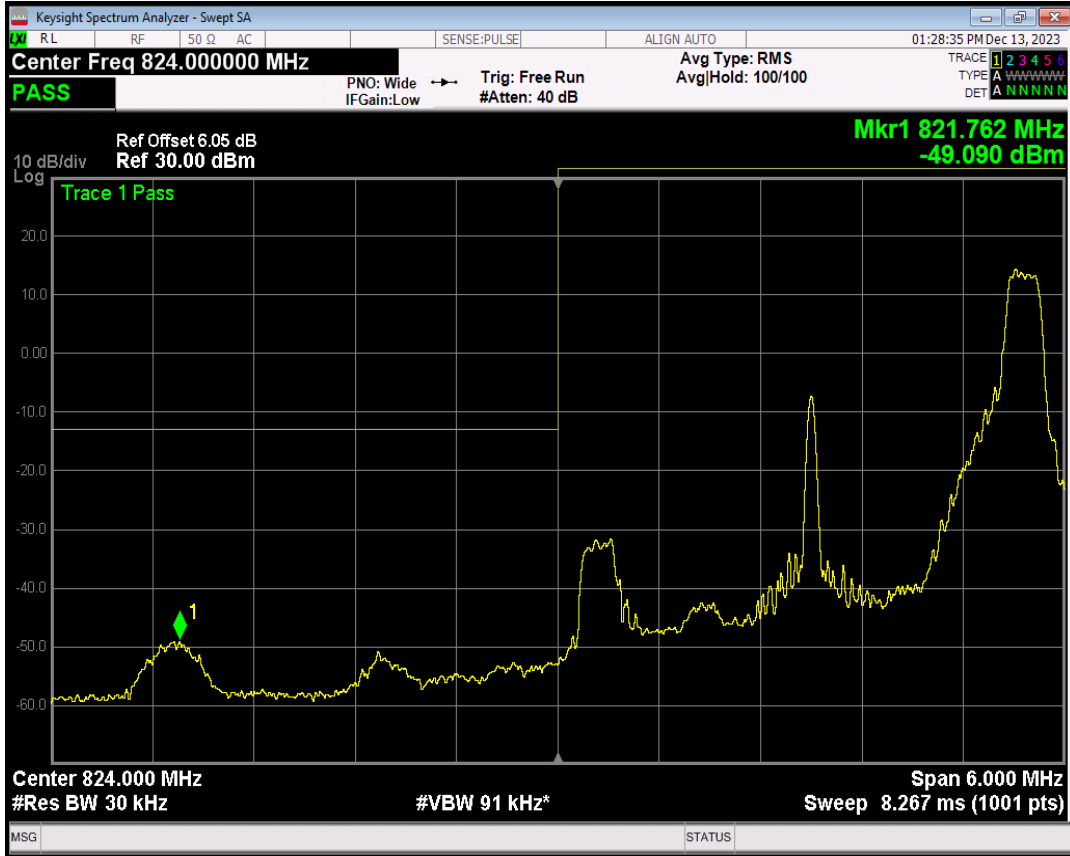
Band5 16QAM BW=3MHz Channel=20415 RB Size=15 Position=#0
