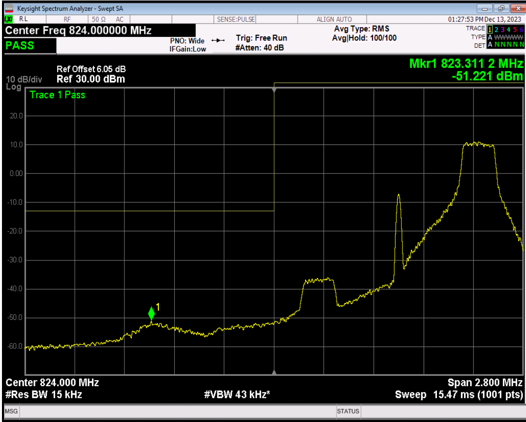
Band5 16QAM BW=1.4MHz Channel=20407 RB Size=6 Position=#0
