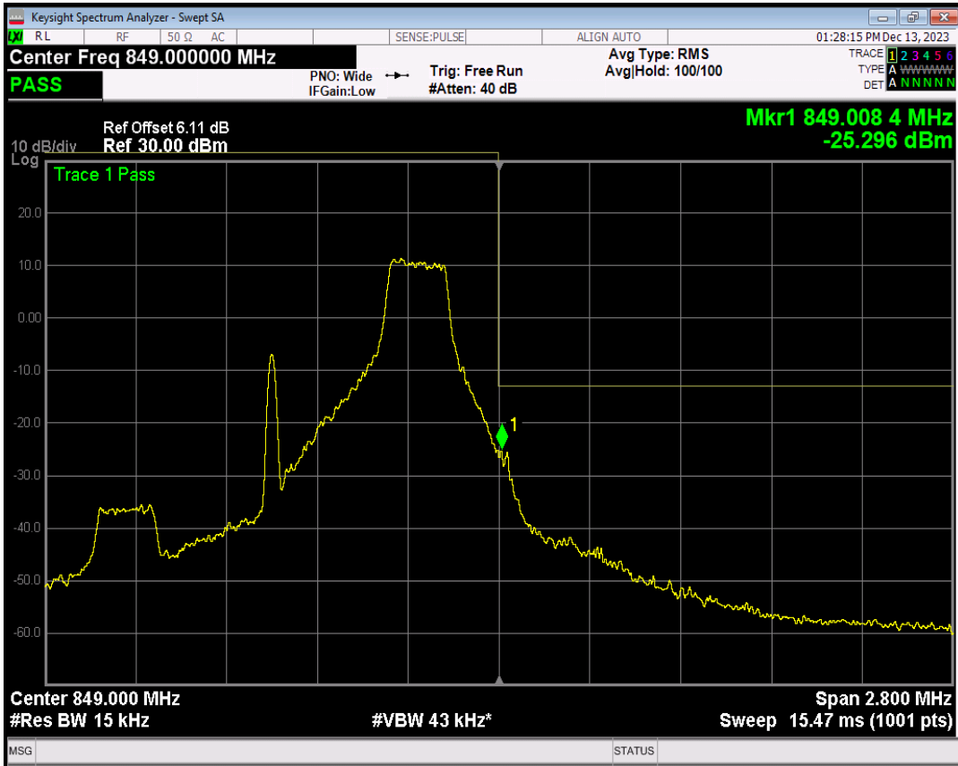
Band5 16QAM BW=1.4MHz Channel=20643 RB Size=6 Position=#0
