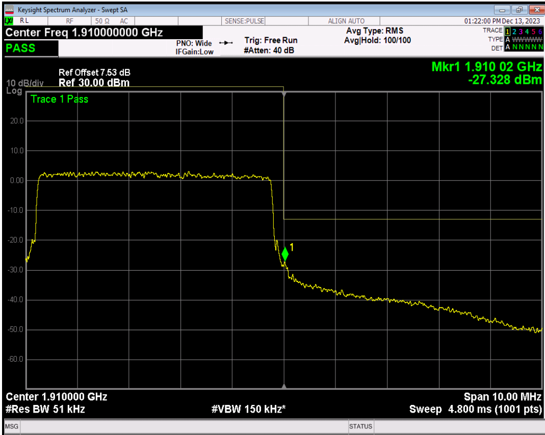
Band2 16QAM BW=5MHz Channel=19175 RB Size=1 Position=#0
