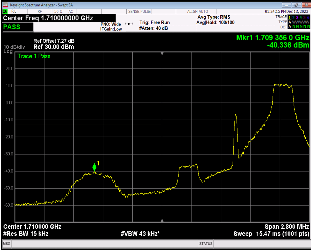
Band4 16QAM BW=1.4MHz Channel=19957 RB Size=6 Position=#0
