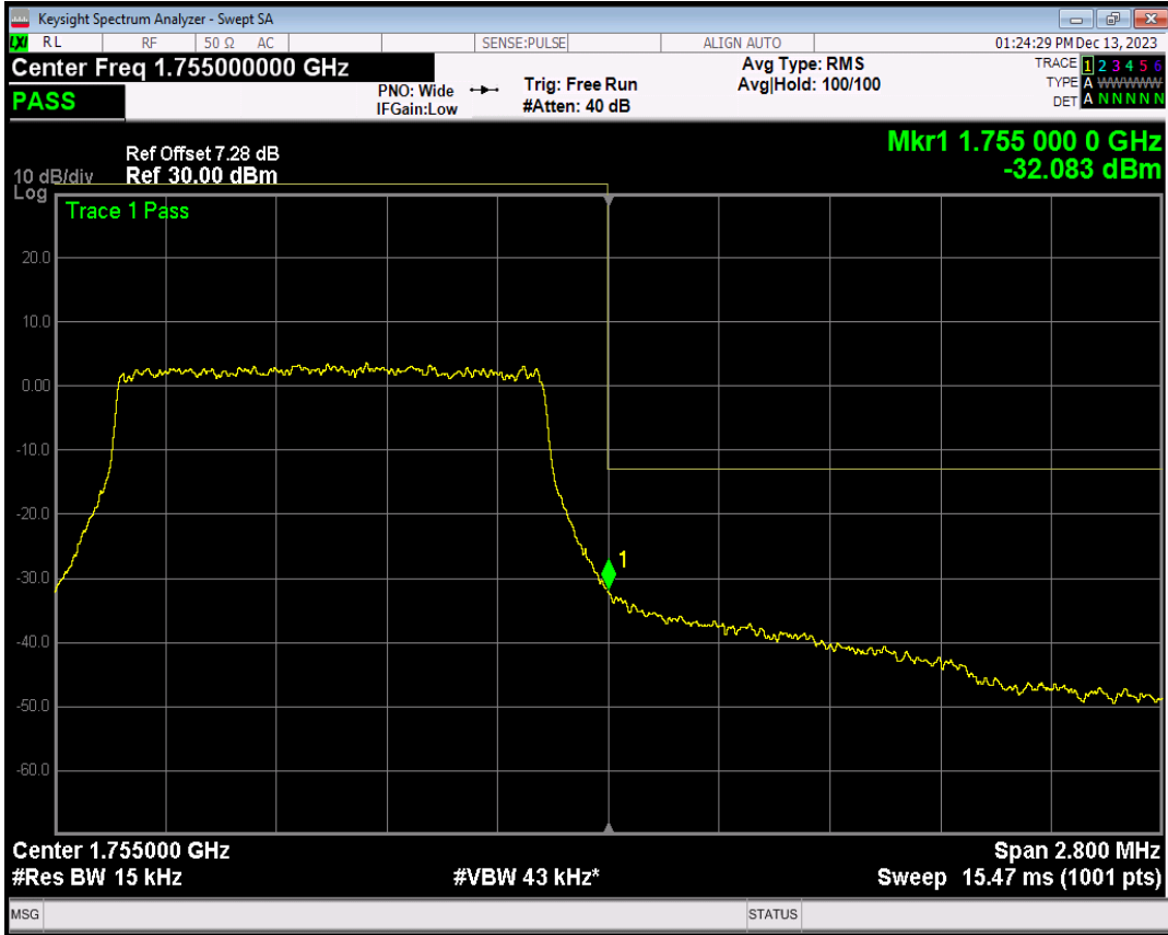
Band4 QPSK BW=10MHz Channel=20000 RB Size=1 Position=#0
