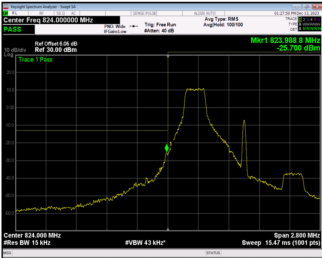
Band5 16QAM BW=1.4MHz Channel=20407 RB Size=1 Position=#Max
