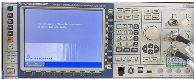
CMW 500 (2G/3G/4G Test Equipment)
