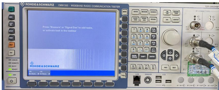
CMW 500 (2G/3G/4G Test Equipment)
