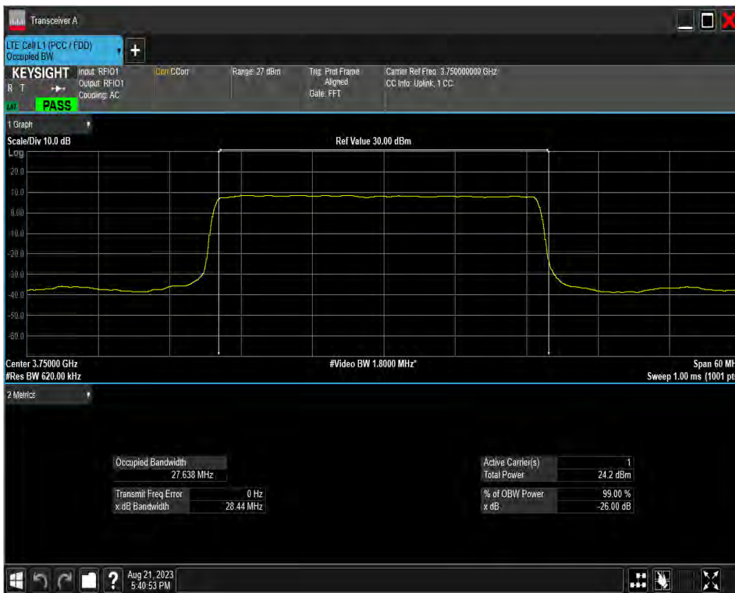
n78(3700-3800) SCS=30kHz DFT BPSK BW=30MHz Channel=652332 RB=75@0
