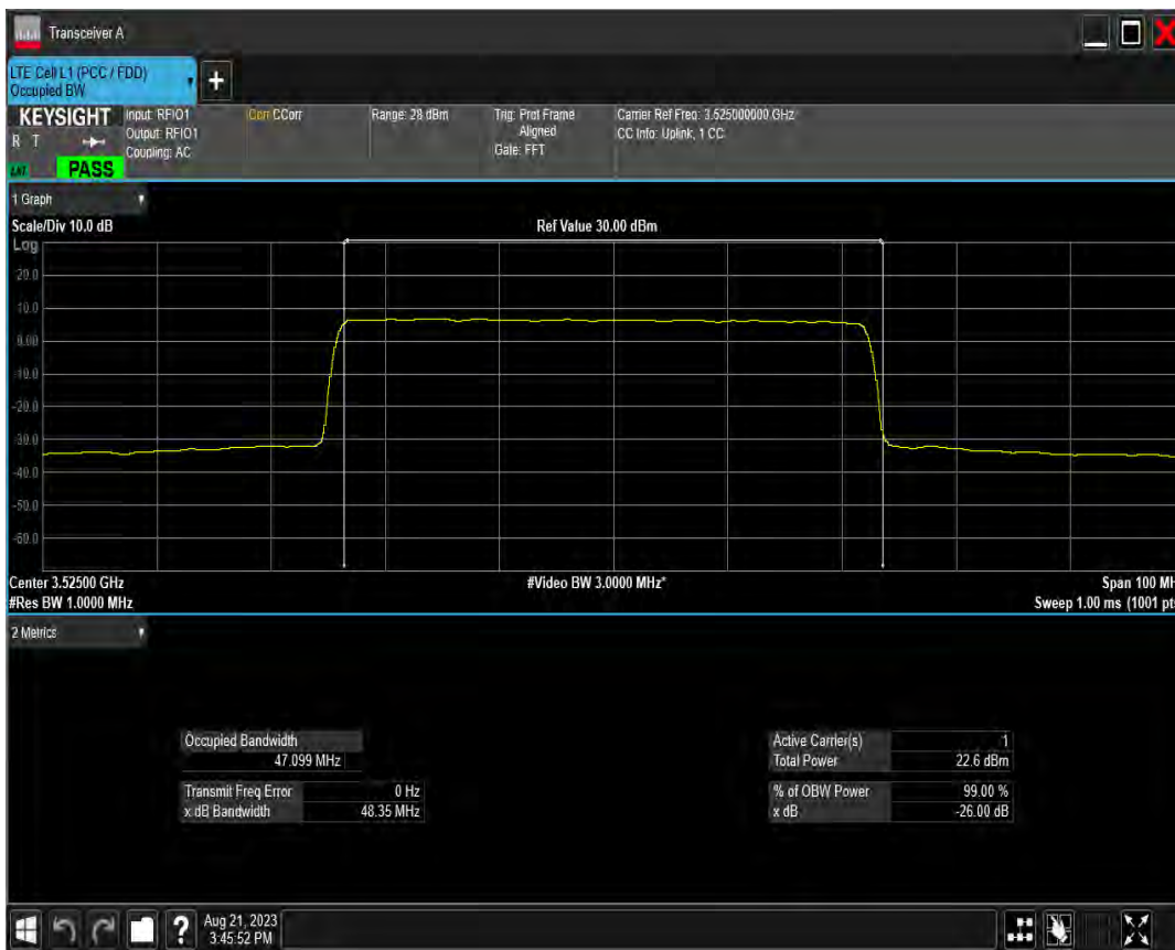
n78(3450-3550) SCS=30kHz DFT 16QAM BW=60MHz Channel=632000 RB=162@0
