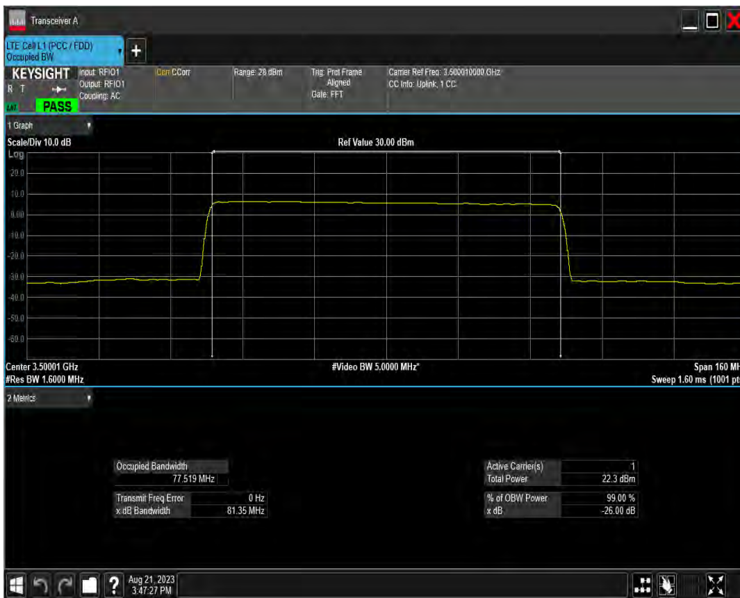
n78(3450-3550) SCS=30kHz DFT 64QAM BW=80MHz Channel=634000 RB=216@0
