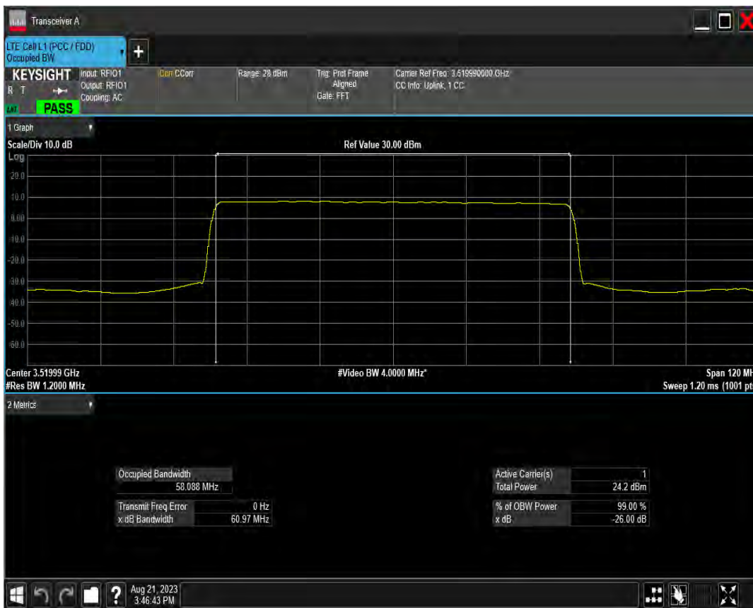
n78(3450-3550) SCS=30kHz DFT BPSK BW=60MHz Channel=632000 RB=162 @0
