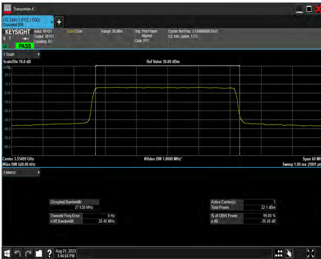
n78(3450-3550) SCS=30kHz DFT 64QAM BW=40MHz Channel=631334 RB=100@0
