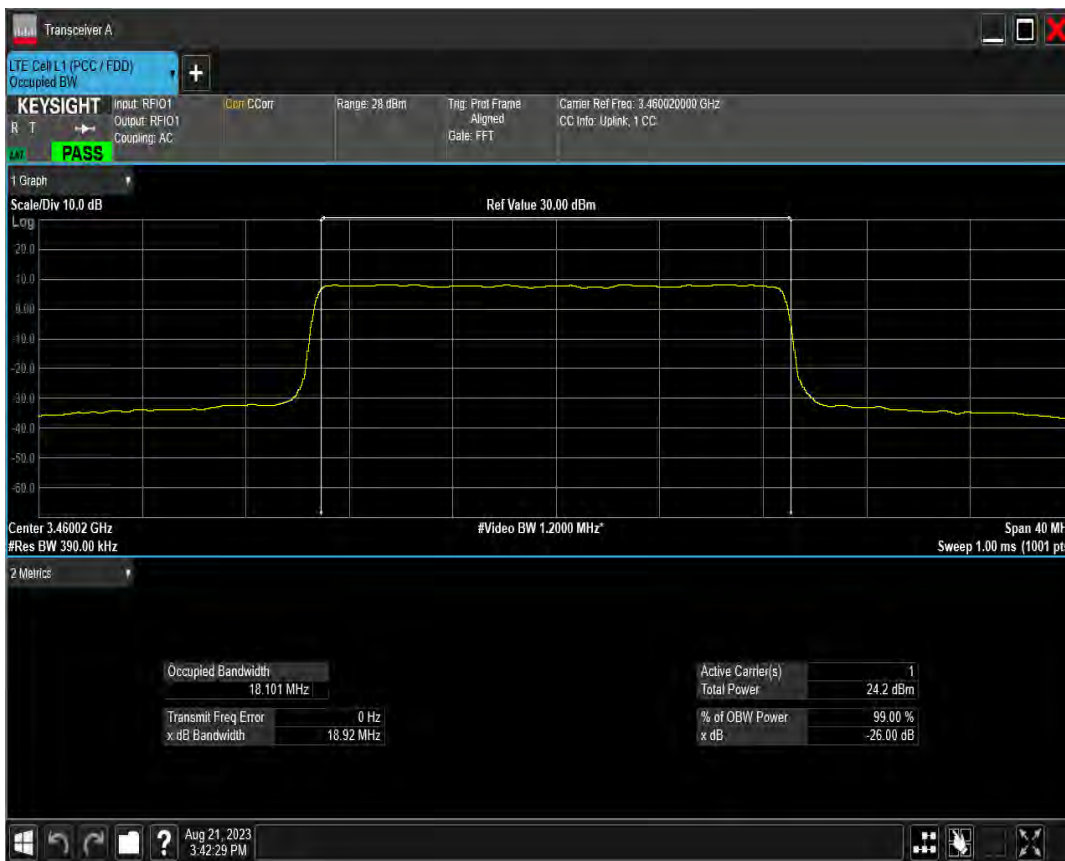
n78(3450-3550) SCS=30kHz DFT QPSK BW=30MHz Channel=633334 RB=75@0
