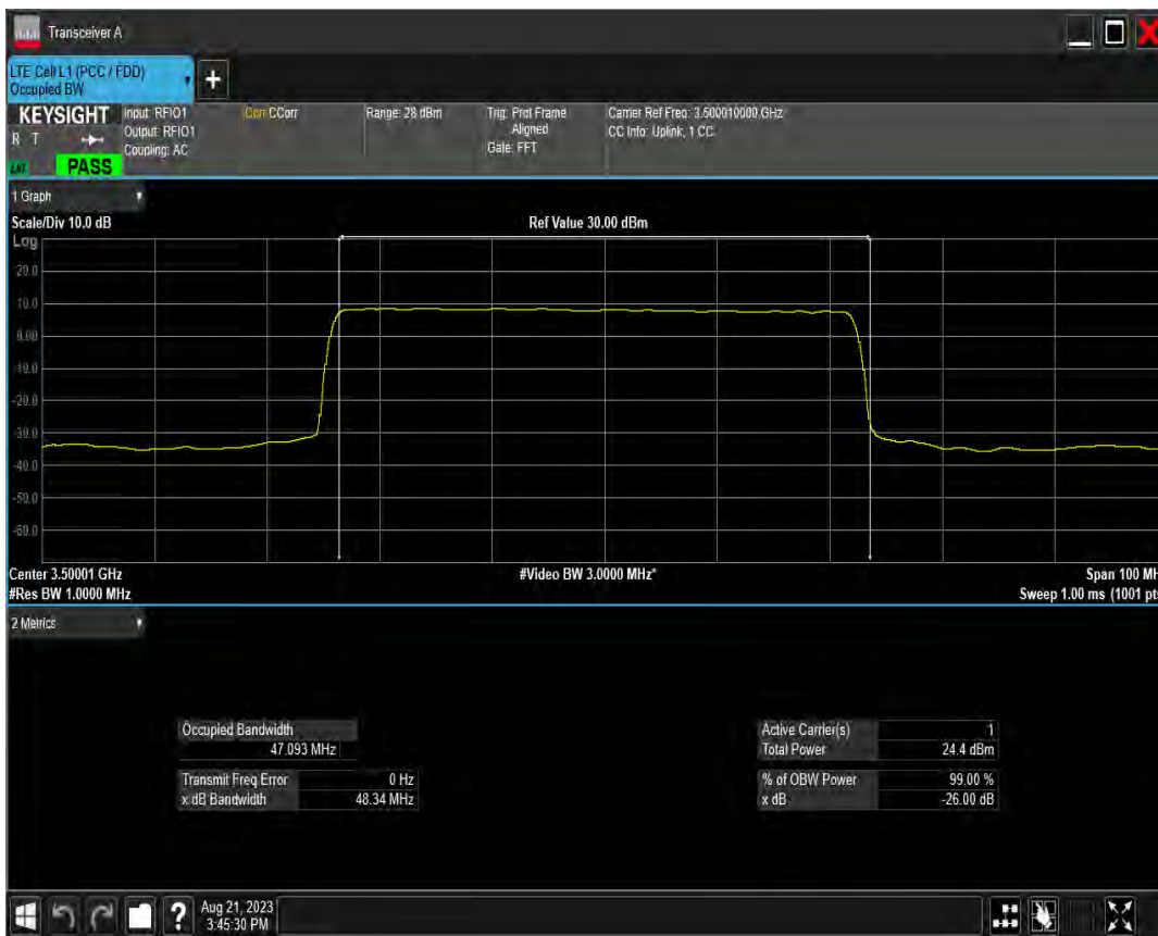
n78(3450-3550) SCS=30kHz DFT BPSK BW=50MHz Channel=635000 RB=128@0
