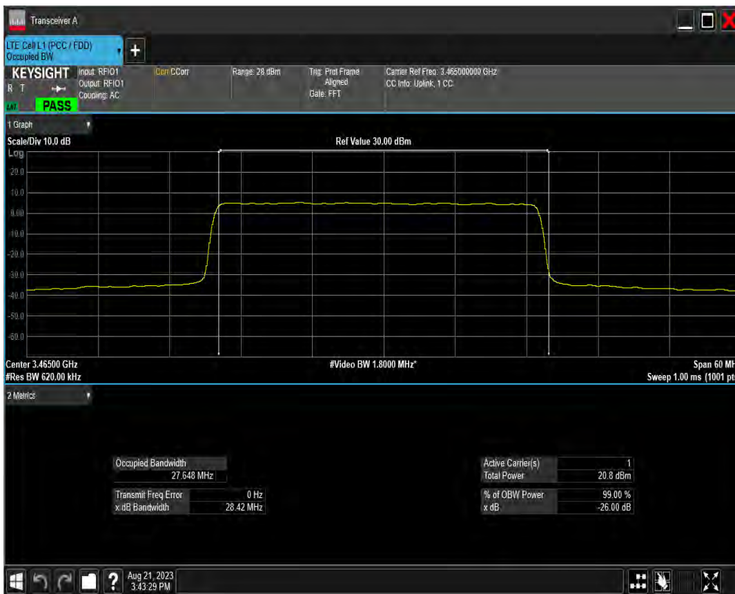
n78(3450-3550) SCS=30kHz DFT 256QAM BW=30MHz Channel=633334 RB=75@0
