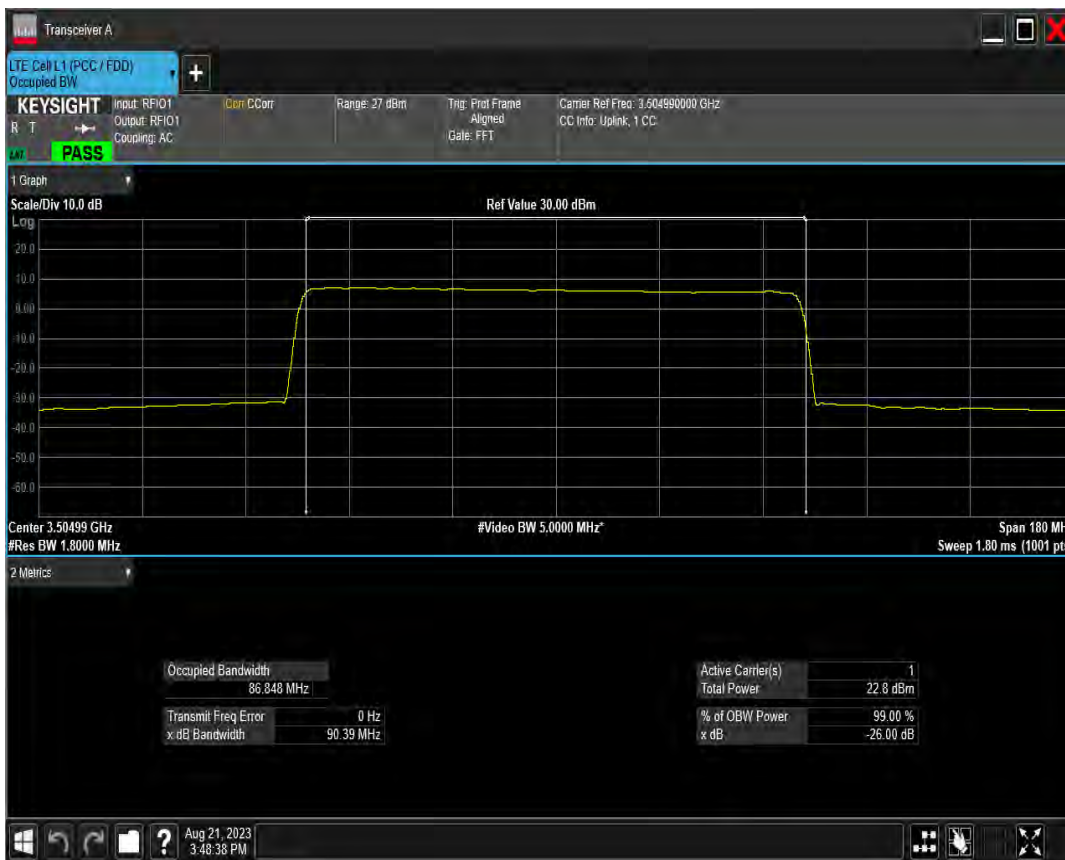
n78(3450-3550) SCS=30kHz DFT 256QAM BW=100MHz Channel=633332 RB=270@0
