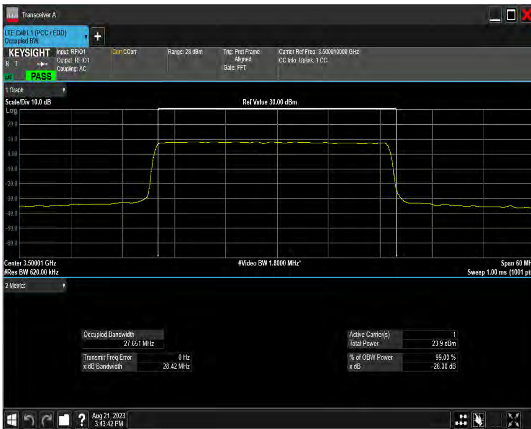
n78(3450-3550) SCS=30kHz DFT QPSK BW=30MHz Channel=635666 RB=75@0
