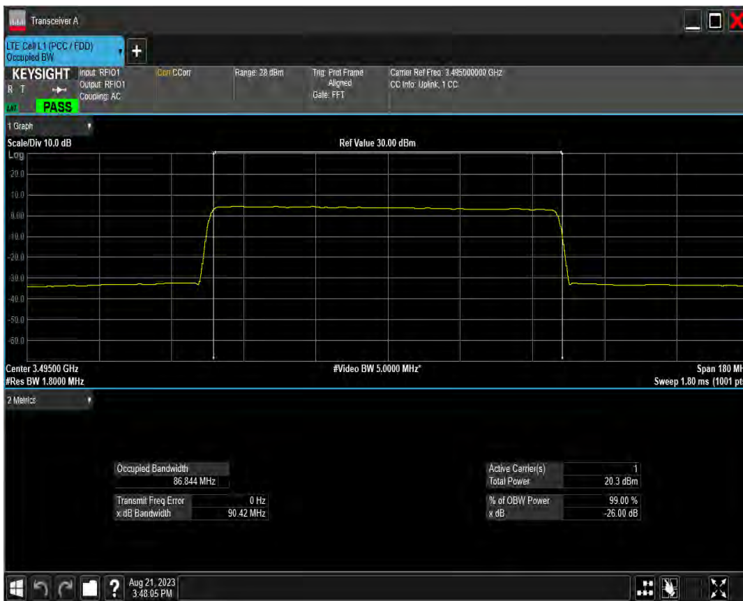
n78(3450-3550) SCS=30kHz DFT 64QAM BW=100MHz Channel=633332 RB=270@0
