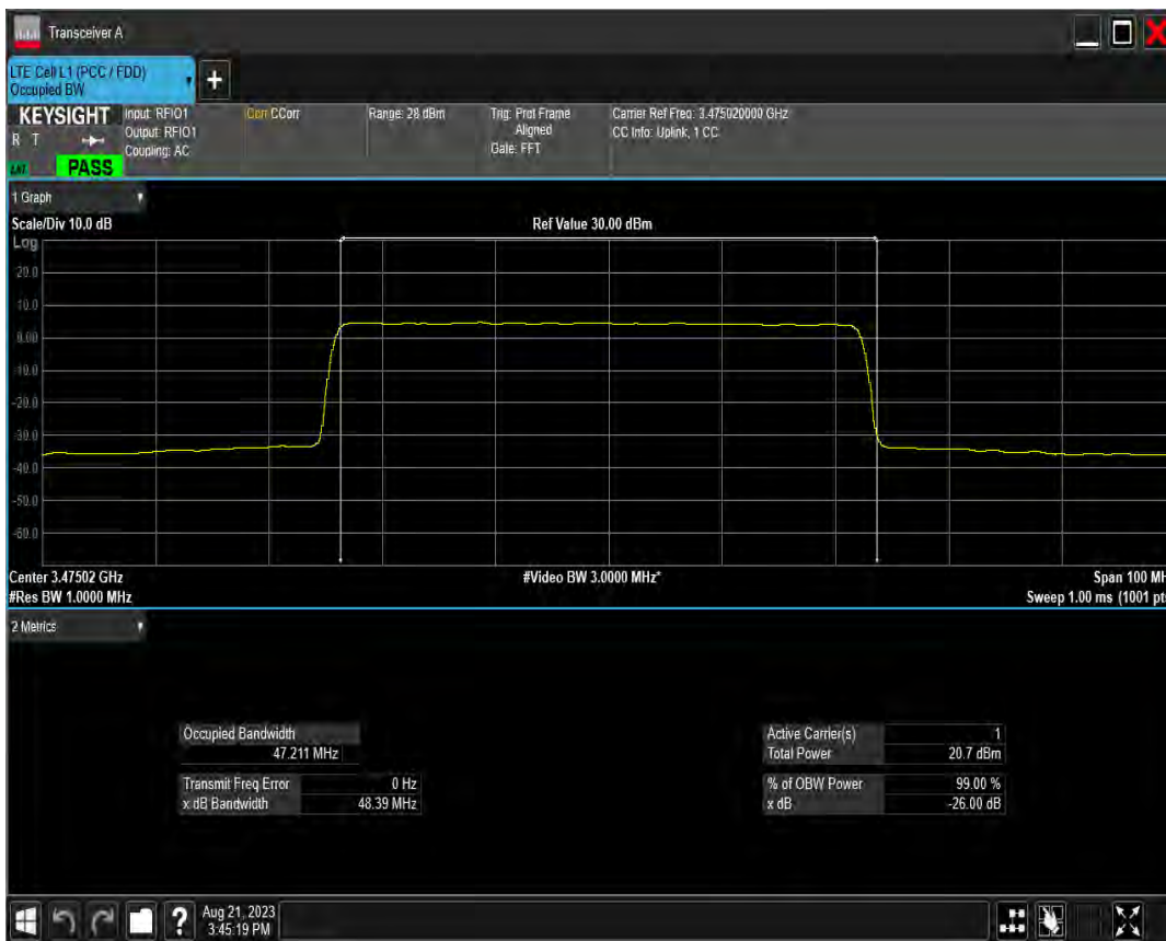
n78(3450-3550) SCS=30kHz DFT 256QAM BW=50MHz Channel=633334 RB=128@0
