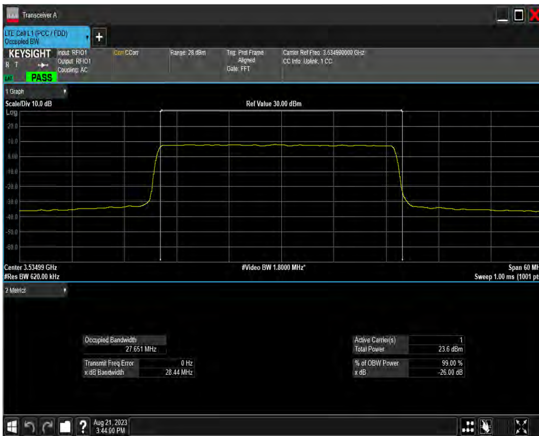
n78(3450-3550) SCS=30kHz DFT QPSK BW=40MHz Channel=631334 RB=100@0
