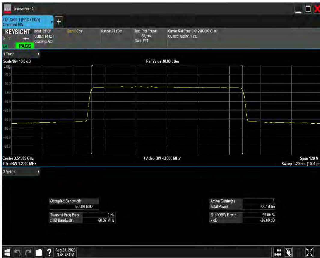
n78(3450-3550) SCS=30kHz DFT 16QAM BW=80MHz Channel=632668 RB=216@0
