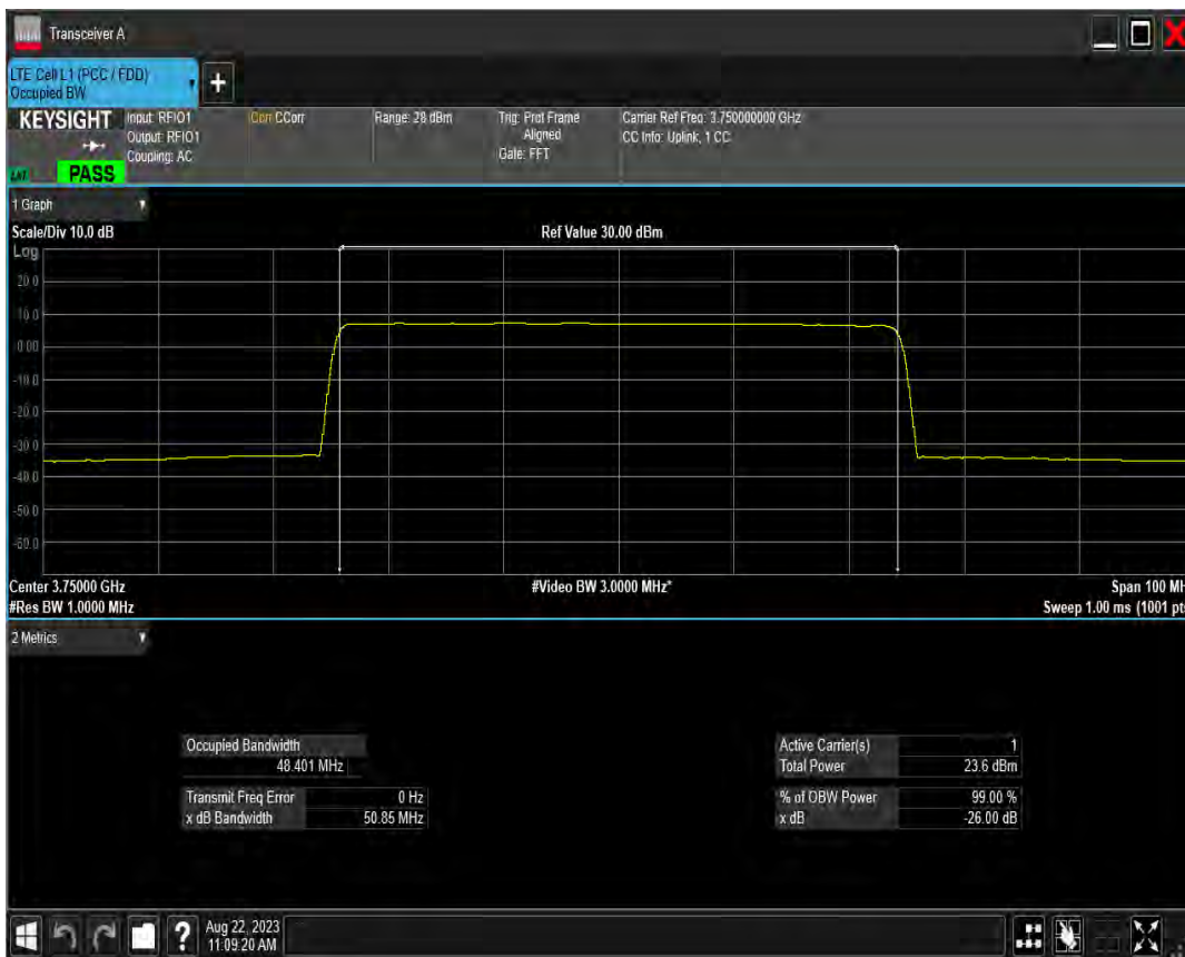
n78(3700-3800) SCS=15kHz DFT QPSK BW=50MHz Channel=651666 RB=270@0
