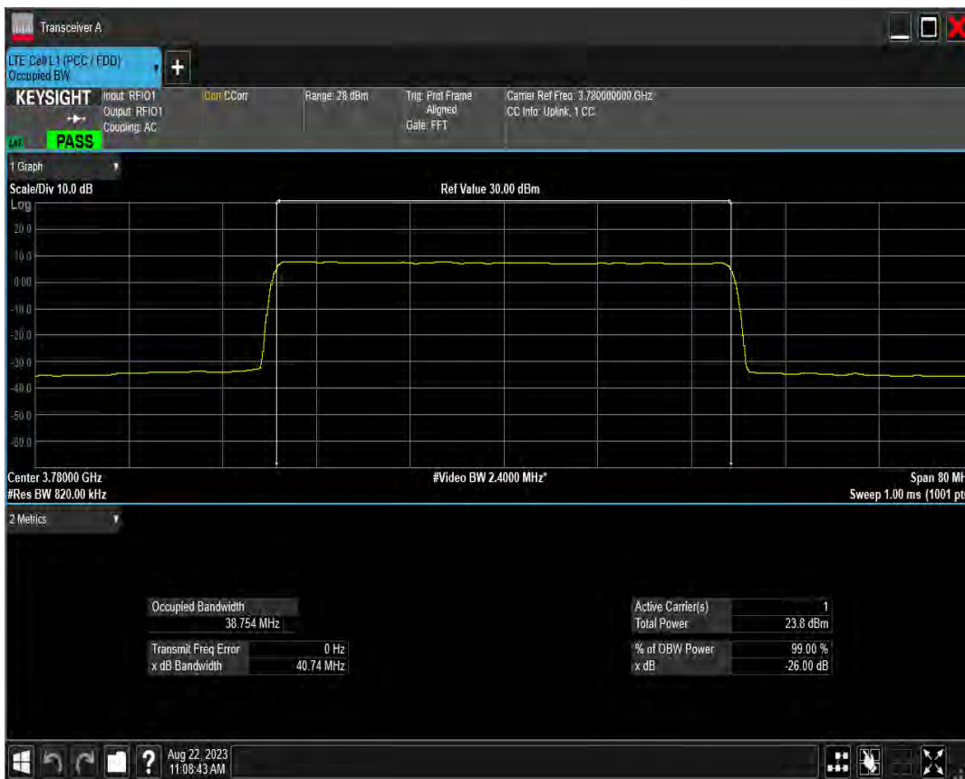
n78(3700-3800) SCS=15kHz DFT QPSK BW=50MHz Channel=648334 RB=270@0
