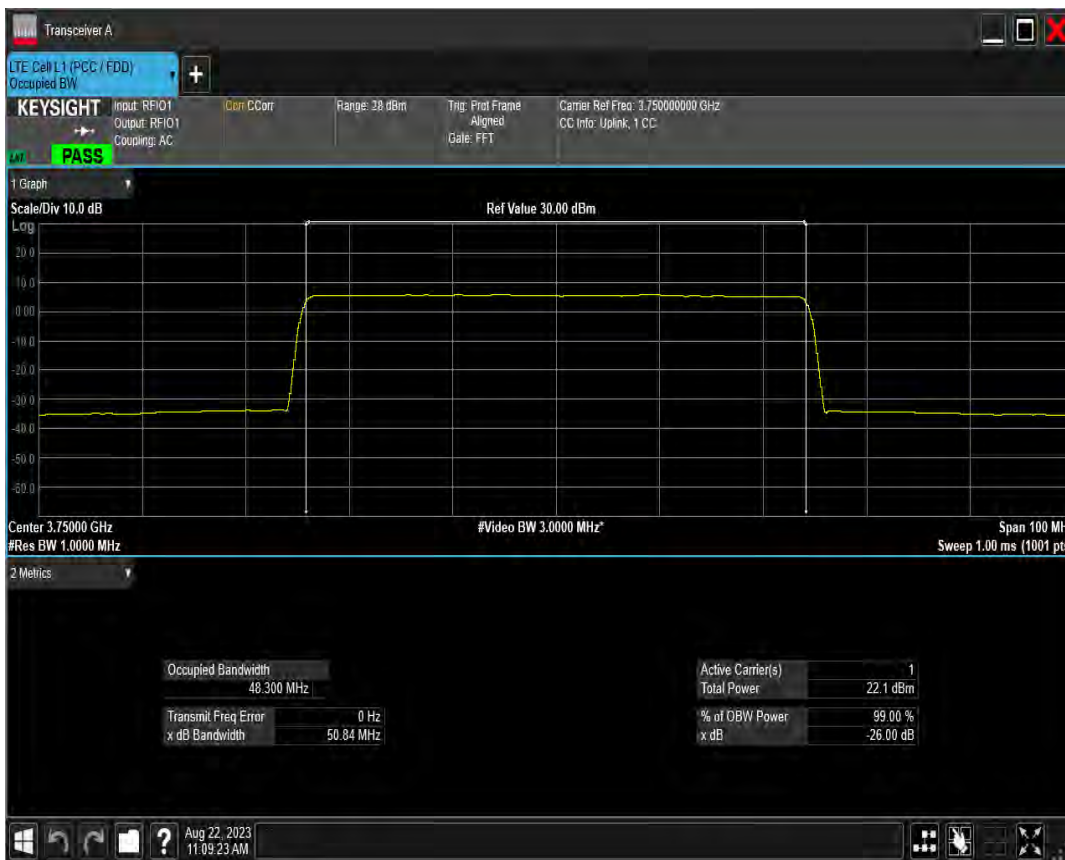
n78(3700-3800) SCS=15kHz DFT 64QAM BW=50MHz Channel=651666 RB=270@0
