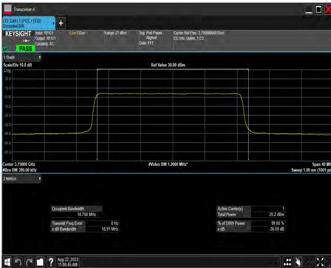
n78(3700-3800) SCS=15kHz DFT 256QAM BW=20MHz Channel=652666 RB=100@0
