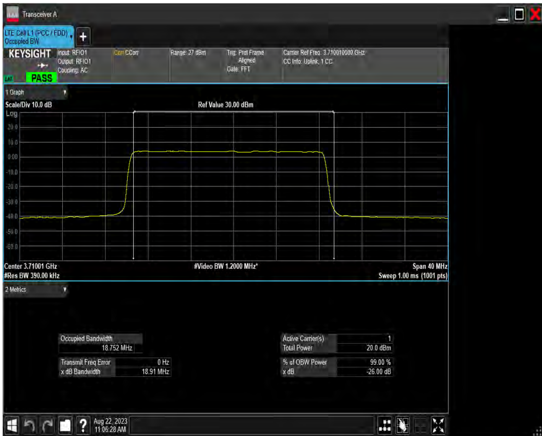
n78(3700-3800) SCS=15kHz DFT 256QAM BW=15MHz Channel=652832 RB=75 @0
