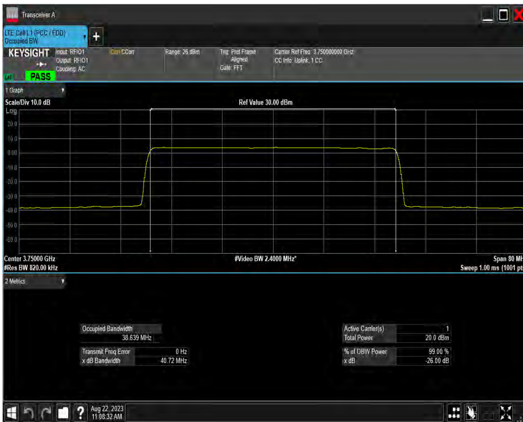
n78(3700-3800) SCS=15kHz DFT 256QAM BW=40MHz Channel=652000 RB=216@0
