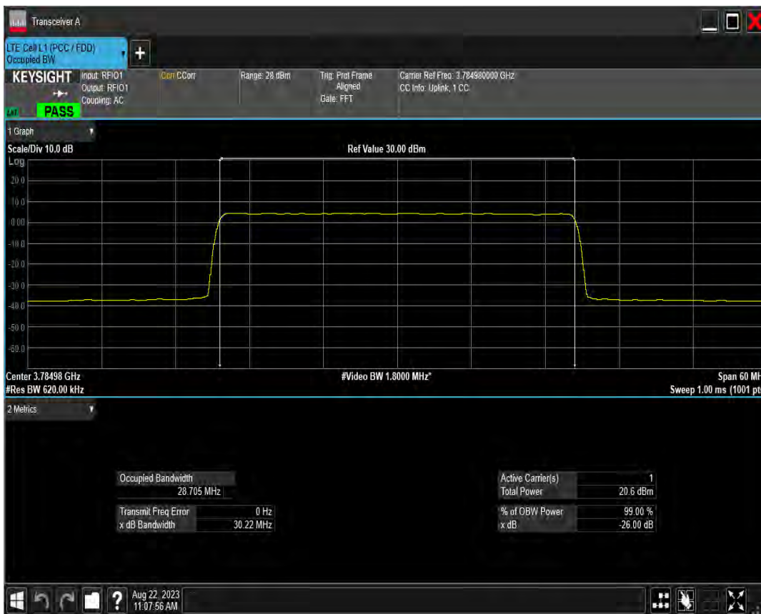
n78(3700-3800) SCS=15kHz DFT 256QAM BW=40MHz Channel=648000 RB=216@0
