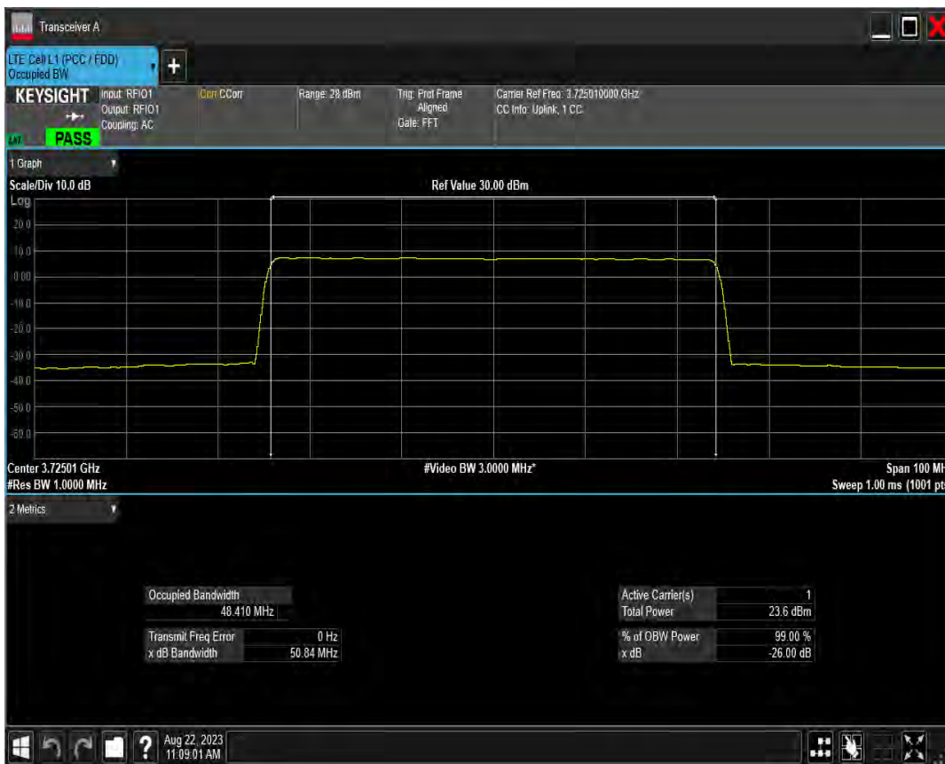
n78(3700-3800) SCS=15kHz DFT QPSK BW=50MHz Channel=650000 RB=270@0
