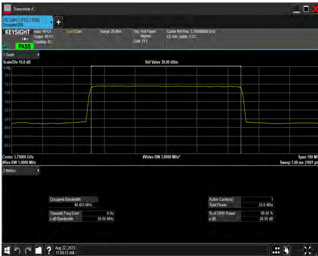
n78(3700-3800) SCS=15kHz DFT BPSK BW=50MHz Channel=651666 RB=270@0
