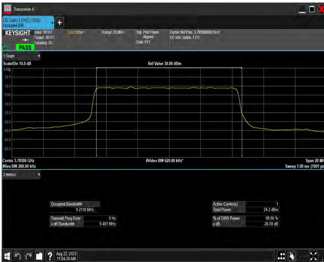
n78(3700-3800) SCS=15kHz DFT BPSK BW=15MHz Channel=650000 RB=75@0
