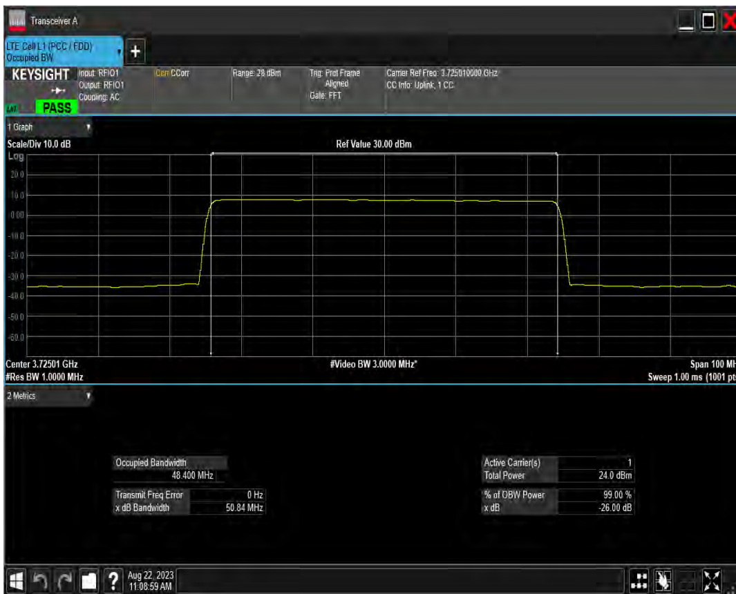
n78(3700-3800) SCS=15kHz DFT BPSK BW=40MHz Channel=652000 RB=216@0
