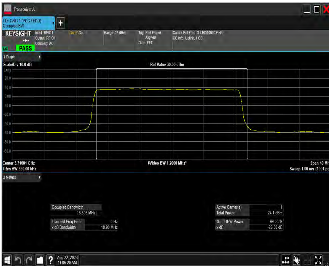
n78(3700-3800) SCS=15kHz DFT BPSK BW=20MHz Channel=650000 RB=100@0
