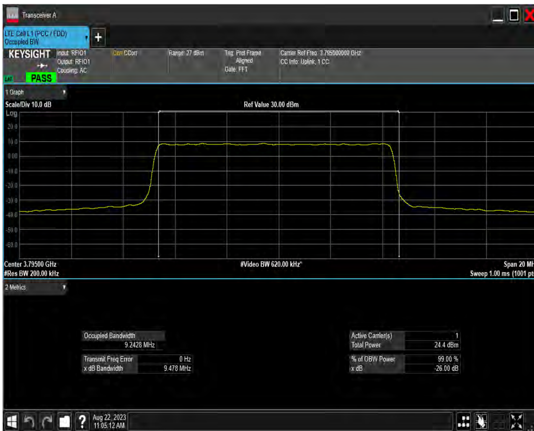
n78(3700-3800) SCS=15kHz DFT QPSK BW=15MHz Channel=647168 RB=75@0
