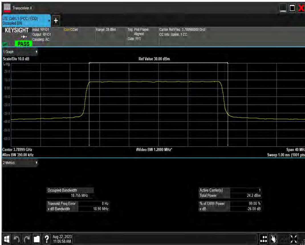
n78(3700-3800) SCS=15kHz DFT QPSK BW=20MHz Channel=650000 RB=100@0
