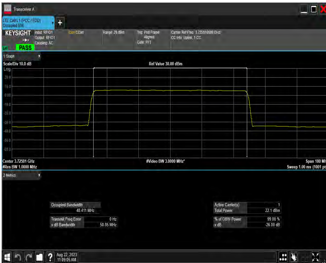
n78(3700-3800) SCS=15kHz DFT 64QAM BW=50MHz Channel=650000 RB=270@0
