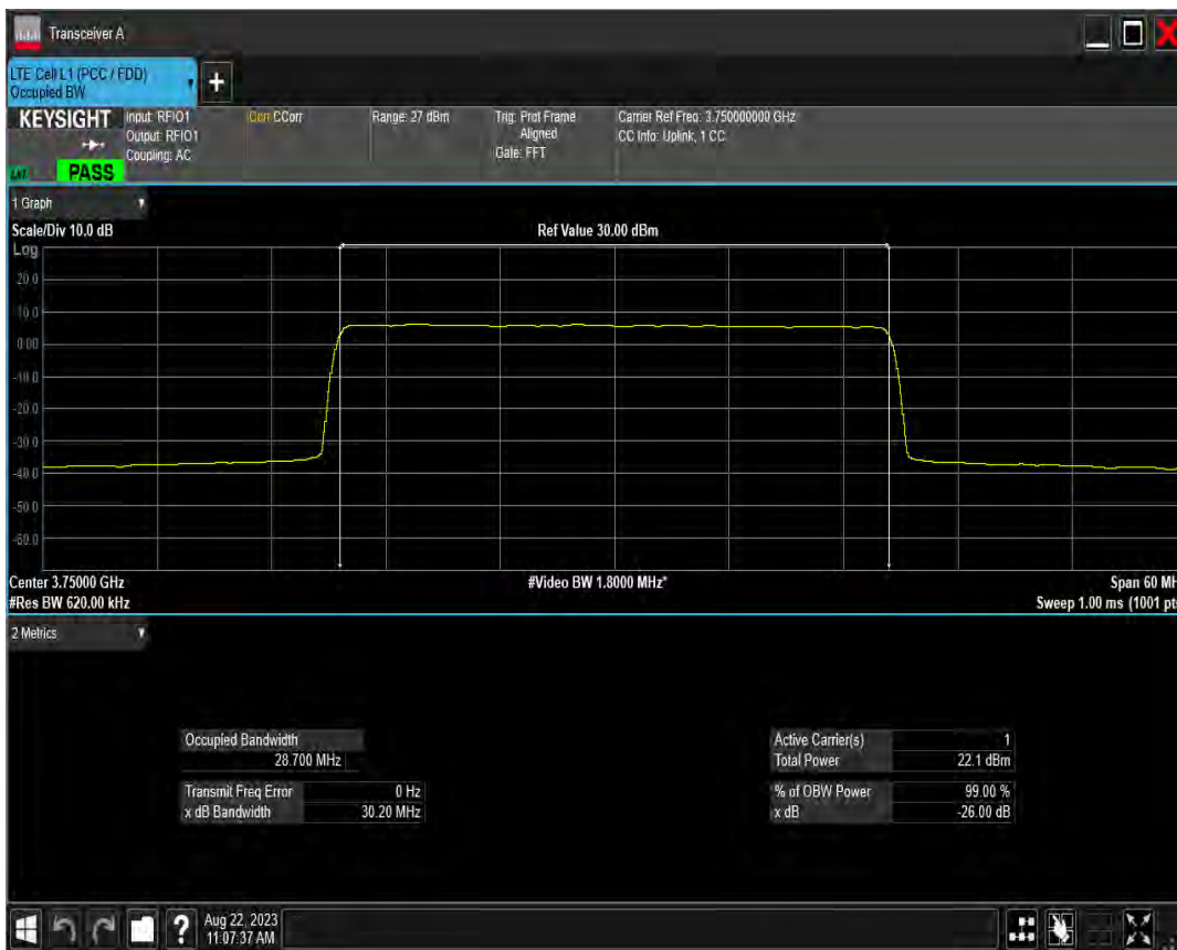
n78(3700-3800) SCS=15kHz DFT 64QAM BW=30MHz Channel=647668 RB=160@0
