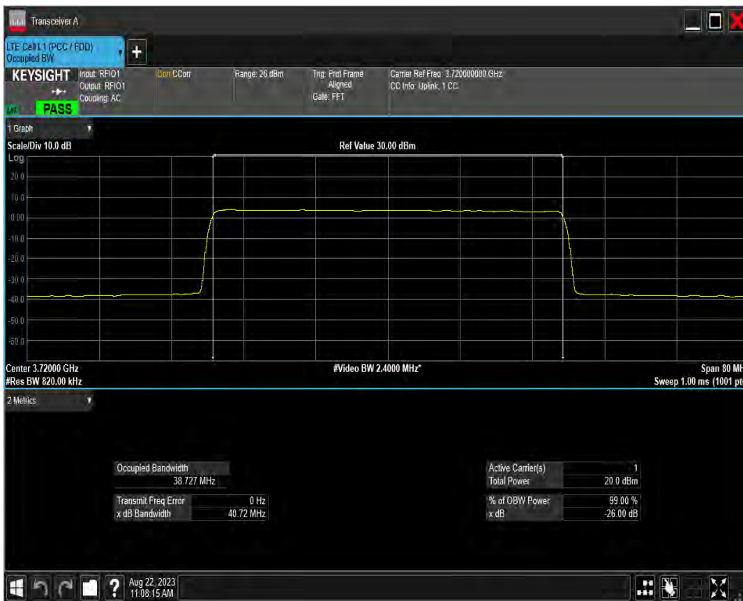
n78(3700-3800) SCS=15kHz DFT 256QAM BW=50MHz Channel=650000 RB=270@0
