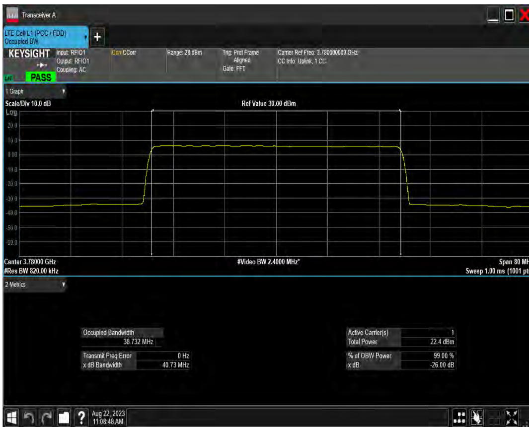
n78(3700-3800) SCS=15kHz DFT 64QAM BW=50MHz Channel=648334 RB=270@0
