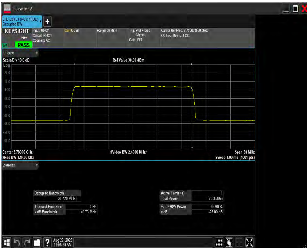
n78(3700-3800) SCS=15kHz DFT 256QAM BW=30MHz Channel=652332 RB=160@0
