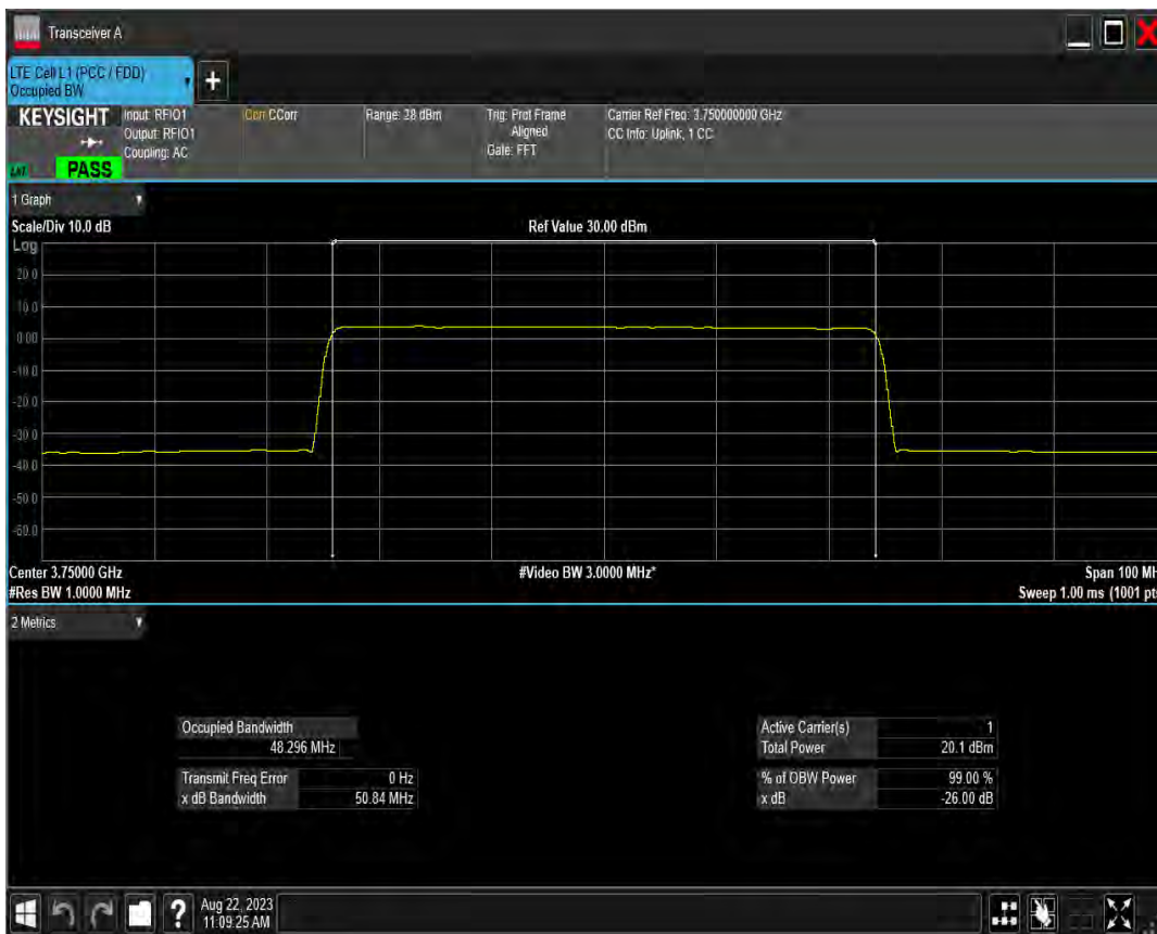
n78(3700-3800) SCS=15kHz DFT 256QAM BW=50MHz Channel=651666 RB=270@0
