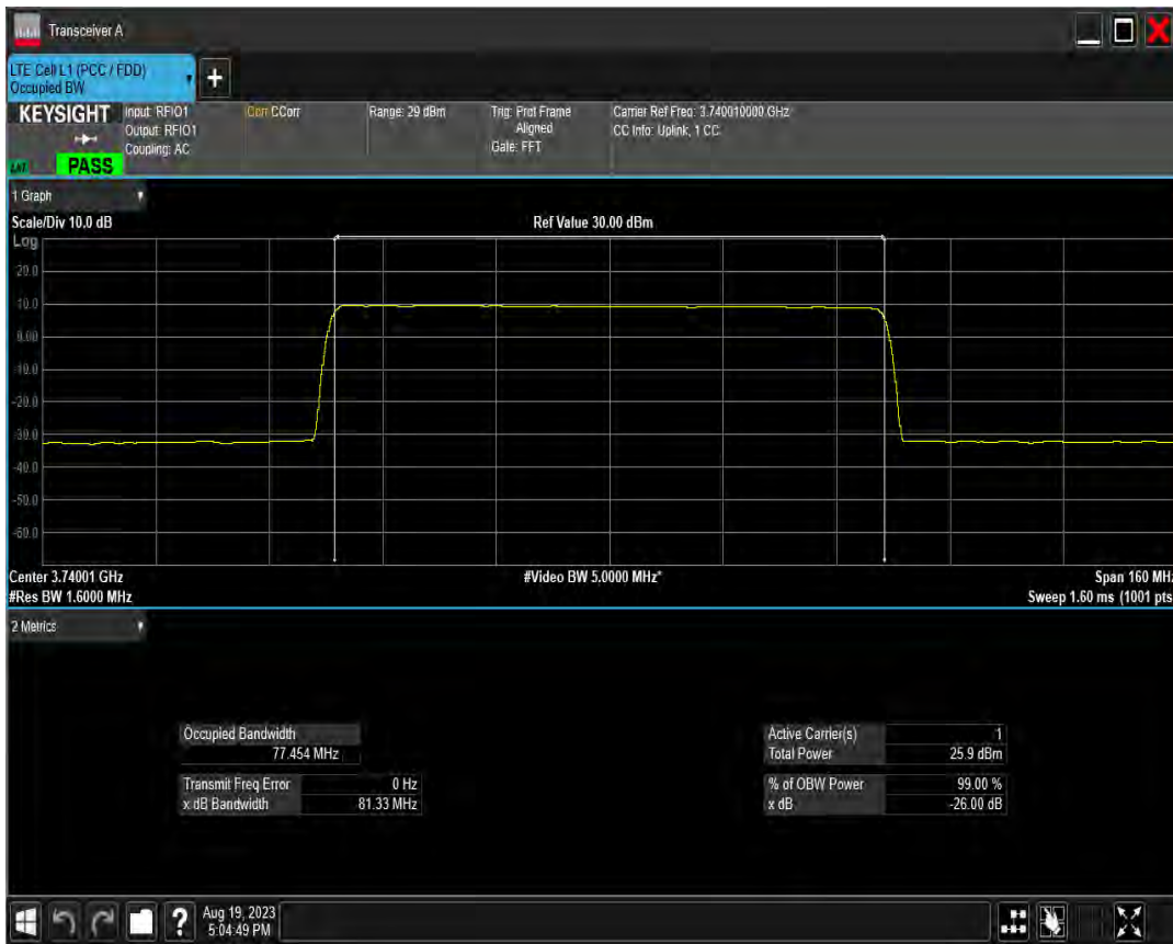
n78(3700-3800) SCS=30kHz DFT BPSK BW=80MHz Channel=650000 RB=216@0
