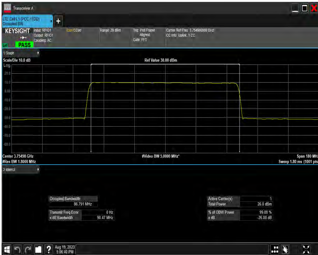
n78(3700-3800) SCS=30kHz DFT 256QAM BW=100MHz Channel=650000 RB=270@0
