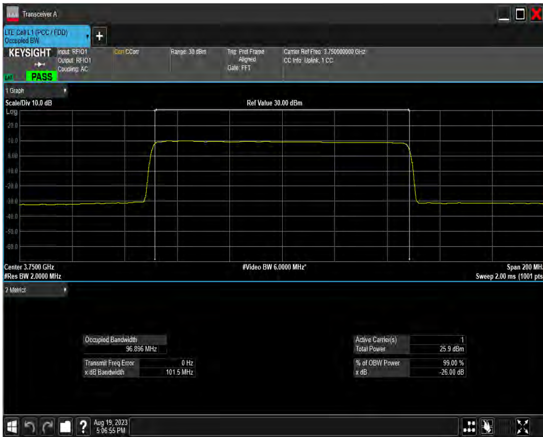
n78(3700-3800) SCS=30kHz DFT BPSK BW=10MHz Channel=647000 RB=24@0
