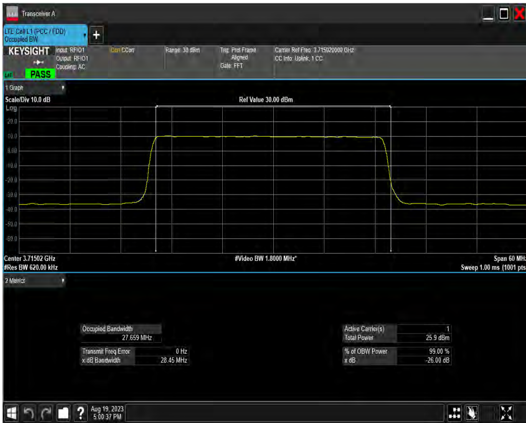
n78(3700-3800) SCS=30kHz DFT BPSK BW=30MHz Channel=650000 RB=75@0
