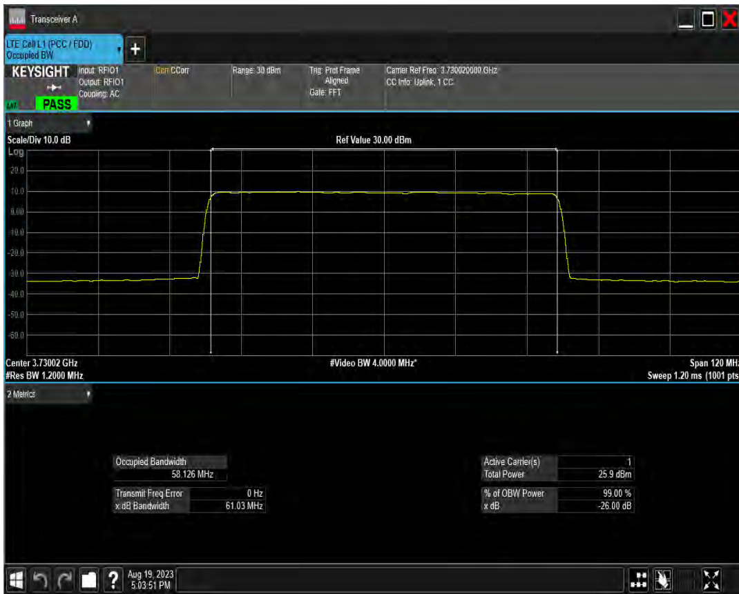
n78(3700-3800) SCS=30kHz DFT 16QAM BW=50MHz Channel=651666 RB=128@0
