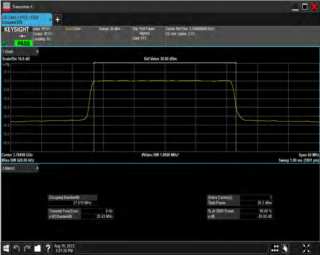
n78(3700-3800) SCS=30kHz DFT 64QAM BW=50MHz Channel=648334 RB=128@0
