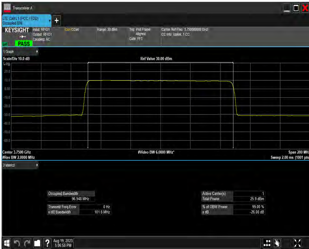
n78(3700-3800) SCS=30kHz DFT QPSK BW=10MHz Channel=647000 RB=24@0
