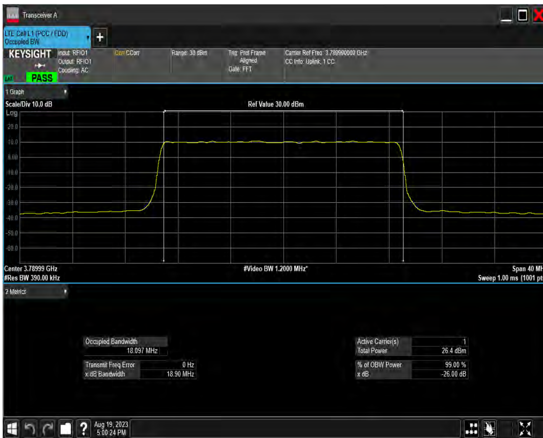
n78(3700-3800) SCS=30kHz DFT 64QAM BW=30MHz Channel=647668 RB=75@0
