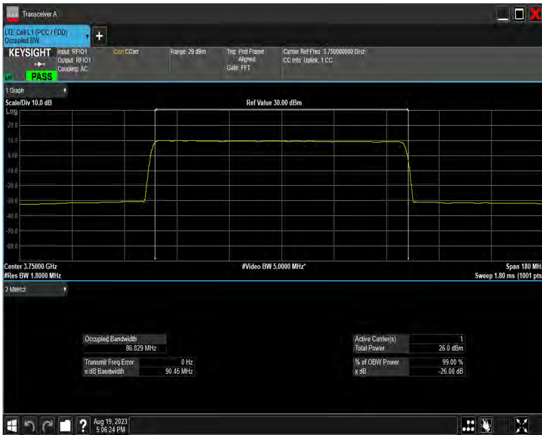
n78(3700-3800) SCS=30kHz DFT 256QAM BW=80MHz Channel=650666 RB=216@0
