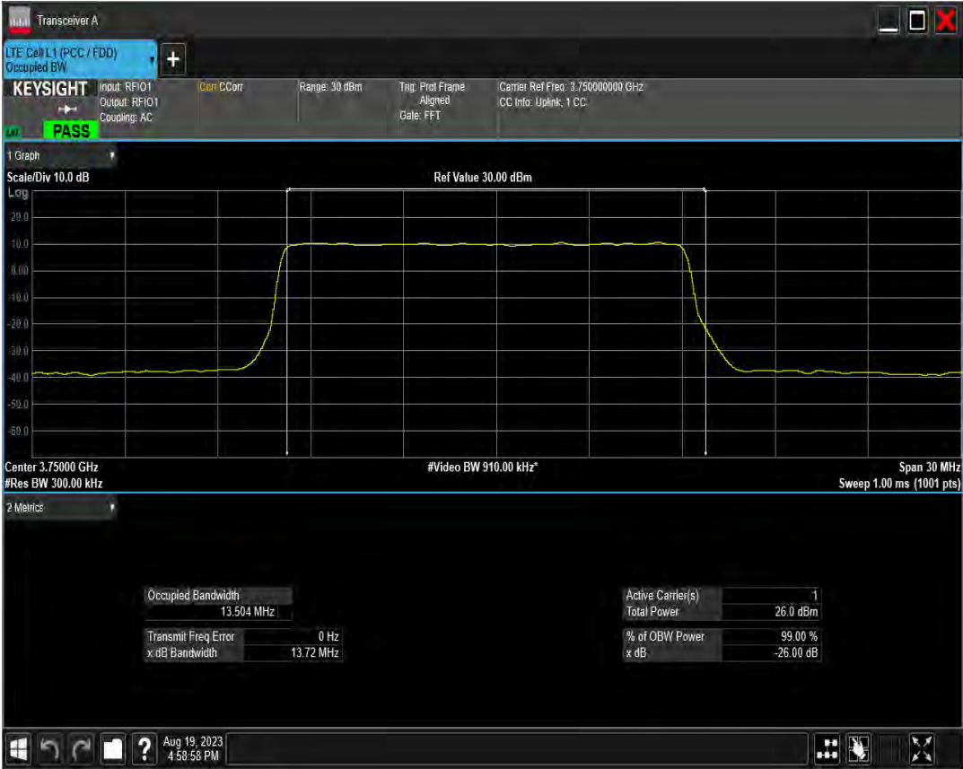
n78(3700-3800) SCS=30kHz DFT QPSK BW=15MHz Channel=652832 RB=36@0
