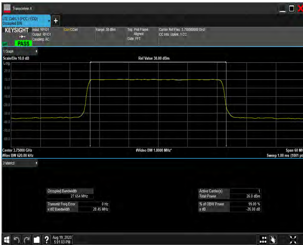
n78(3700-3800) SCS=30kHz DFT 16QAM BW=30MHz Channel=652332 RB=75@0
