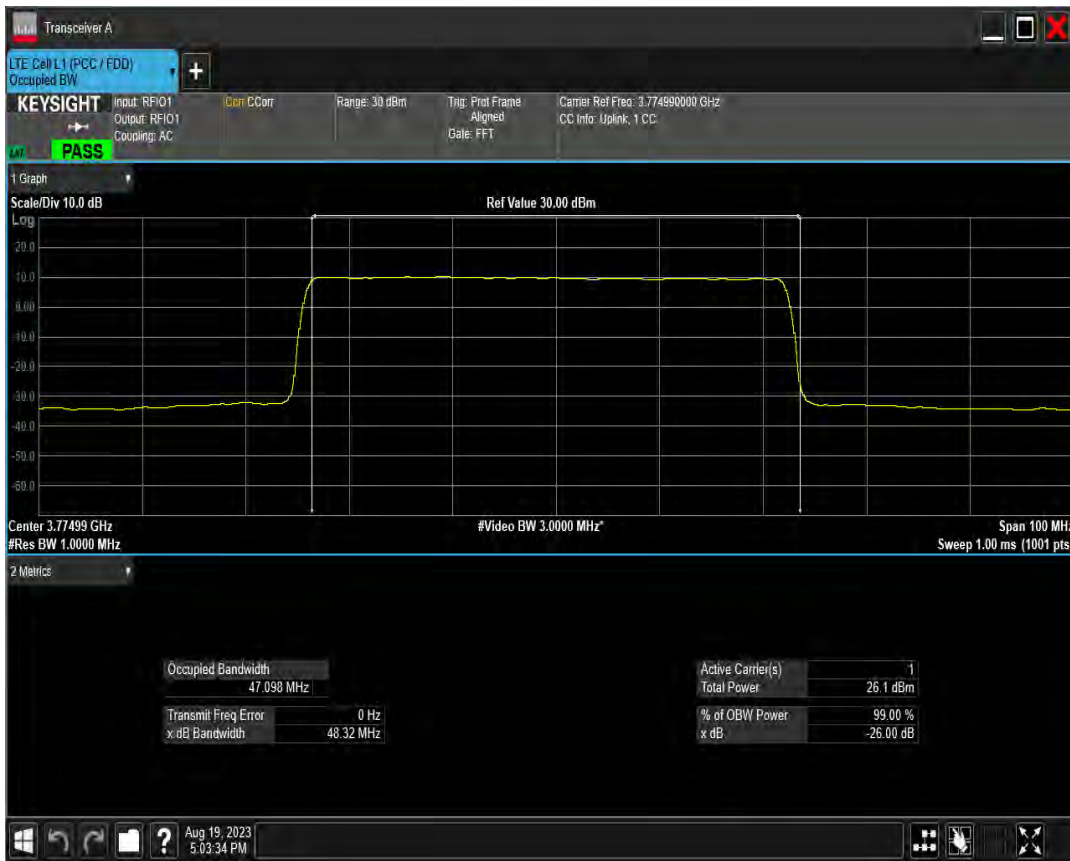
n78(3700-3800) SCS=30kHz DFT 64QAM BW=60MHz Channel=648668 RB=162@0
