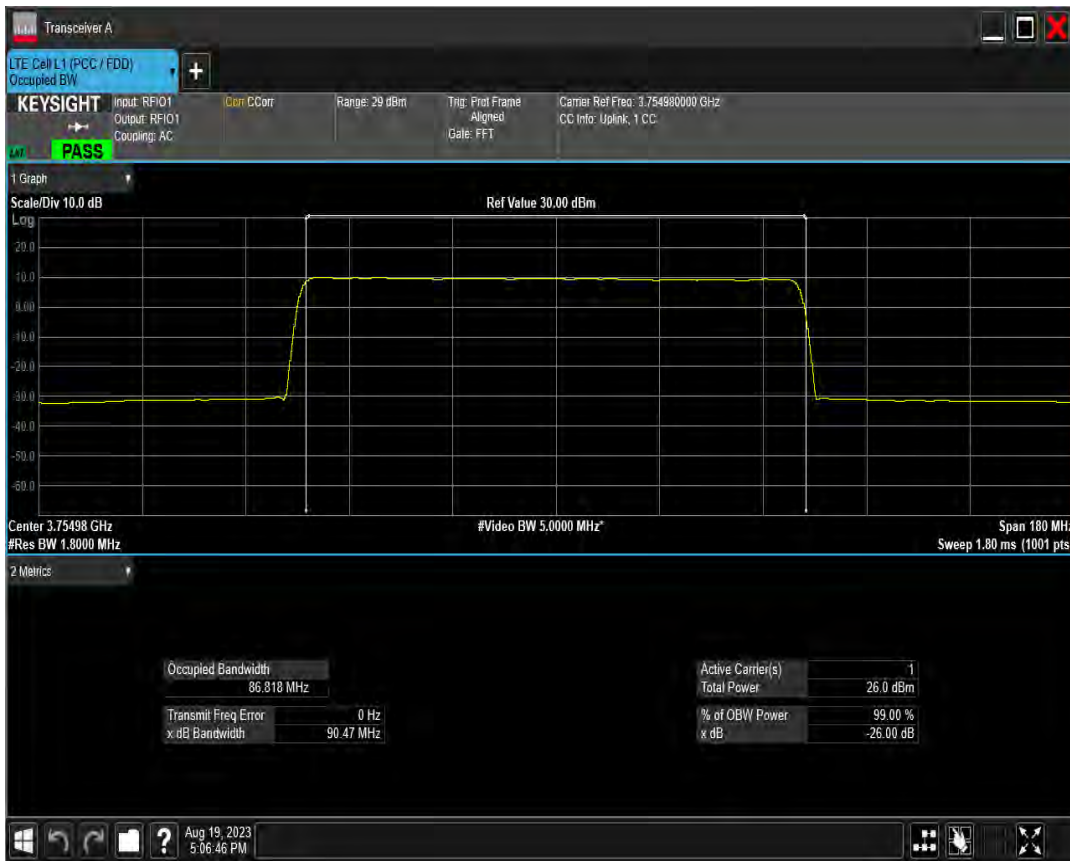
n78(3700-3800) SCS=30kHz DFT 256QAM BW=90MHz Channel=650000 RB=240@0
