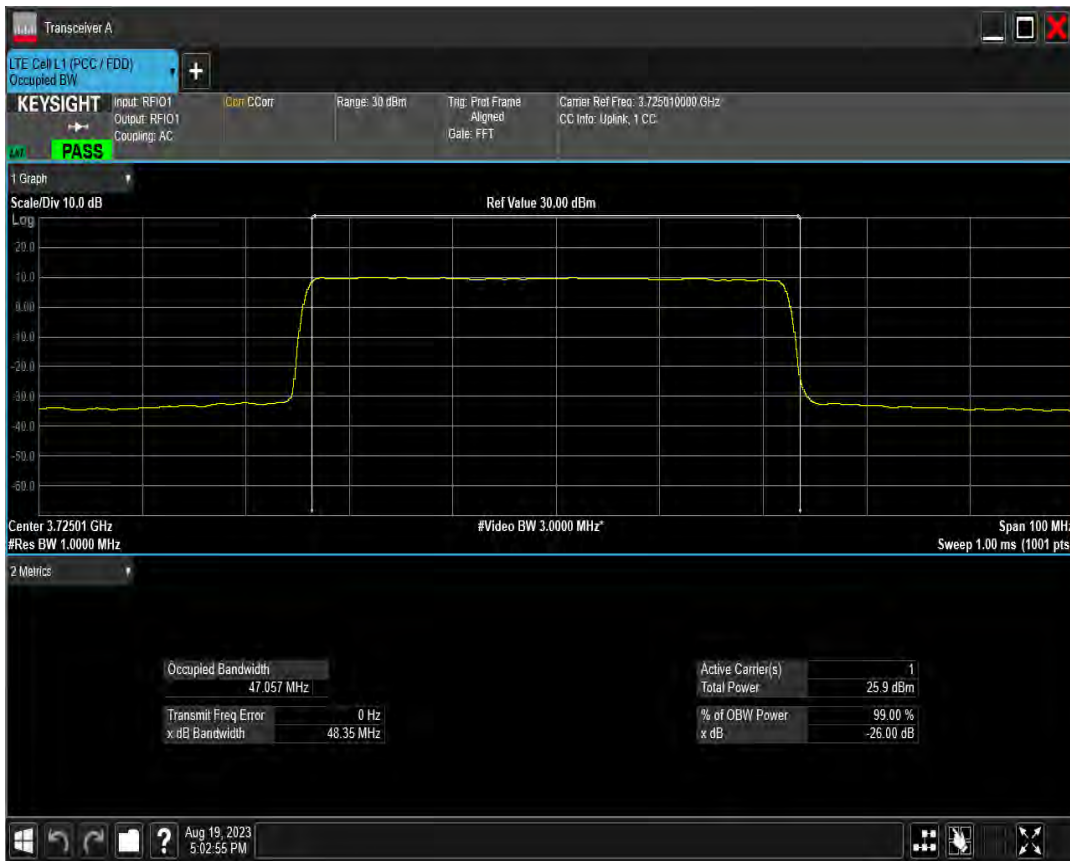
n78(3700-3800) SCS=30kHz DFT 256QAM BW=40MHz Channel=648000 RB=100@0
