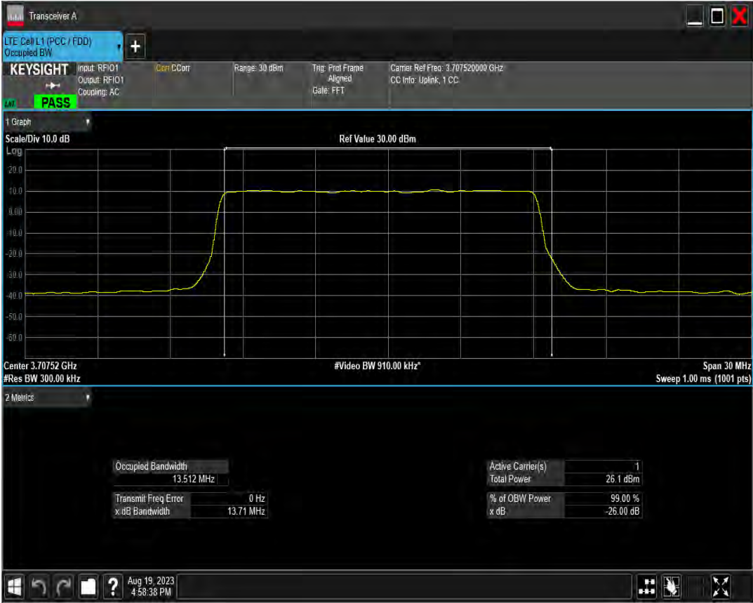
n78(3700-3800) SCS=30kHz DFT QPSK BW=15MHz Channel=650000 RB=36@0
