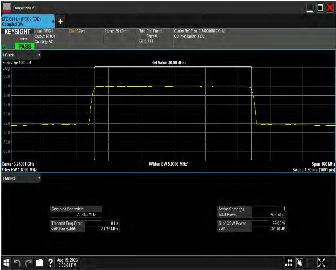
n78(3700-3800) SCS=30kHz DFT 256QAM BW=80MHz Channel=650000 RB=216@0
