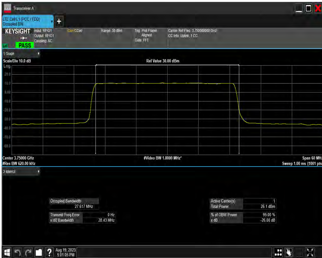
n78(3700-3800) SCS=30kHz DFT 64QAM BW=40MHz Channel=652000 RB=100@0
