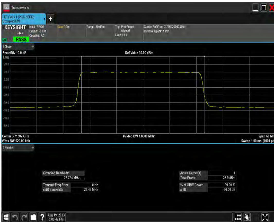
n78(3700-3800) SCS=30kHz DFT 16QAM BW=30MHz Channel=650000 RB=75@0
