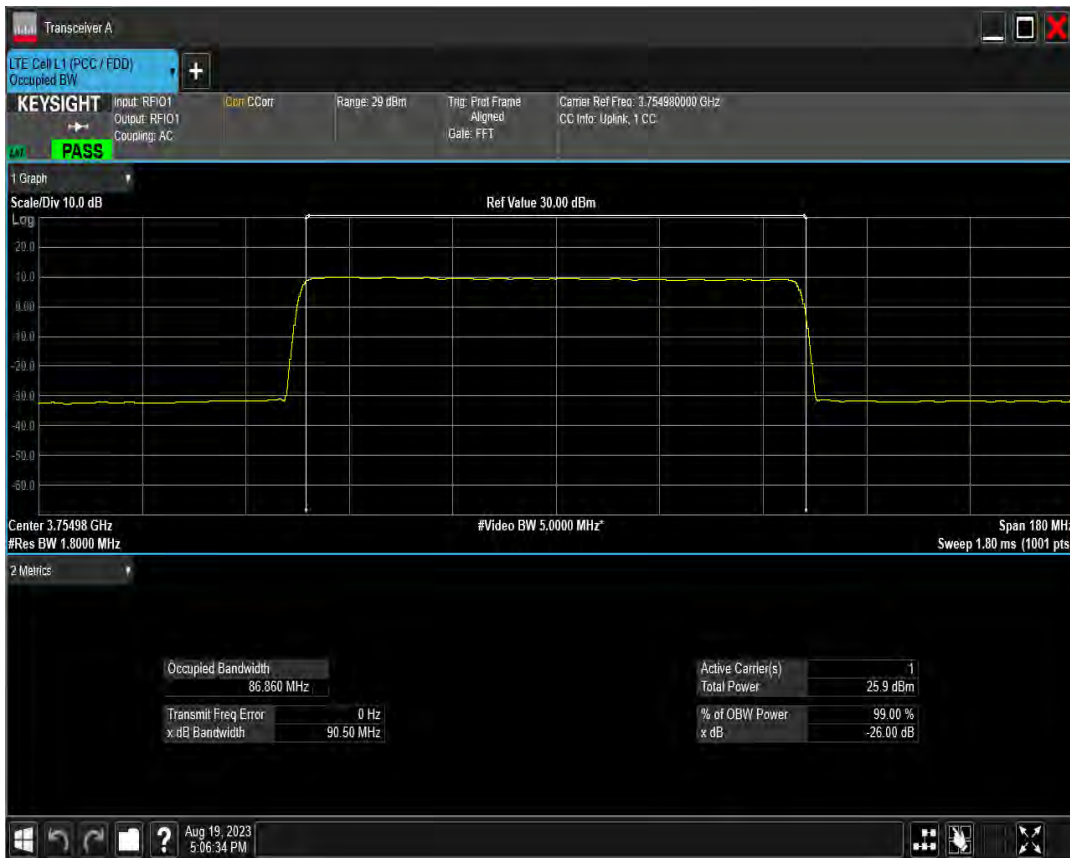
n78(3700-3800) SCS=30kHz DFT QPSK BW=10MHz Channel=650000 RB=24@0
