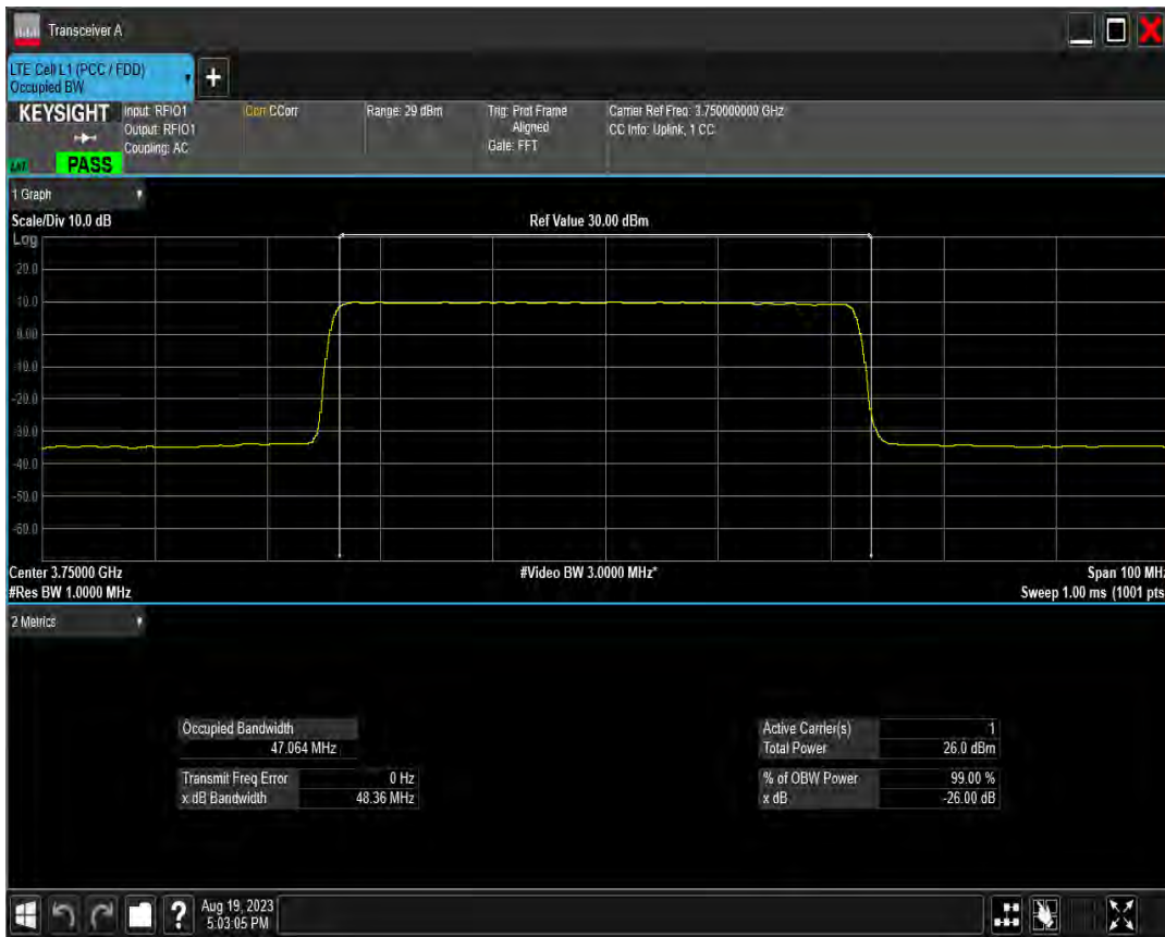
n78(3700-3800) SCS=30kHz DFT BPSK BW=60MHz Channel=650000 RB=162@0
