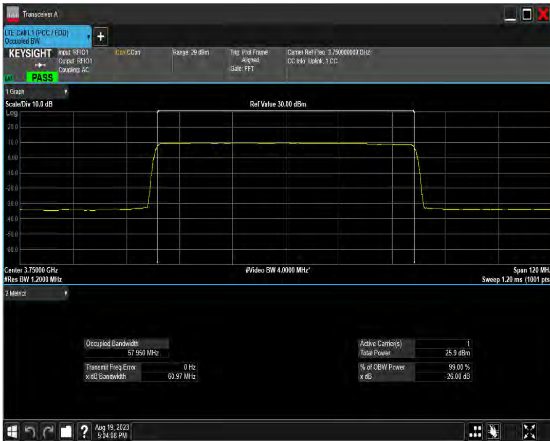
n78(3700-3800) SCS=30kHz DFT BPSK BW=60MHz Channel=651332 RB=162@0
