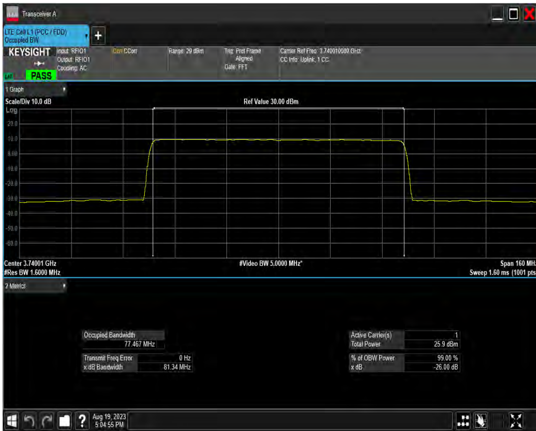
n78(3700-3800) SCS=30kHz DFT 16QAM BW=80MHz Channel=650000 RB=216@0
