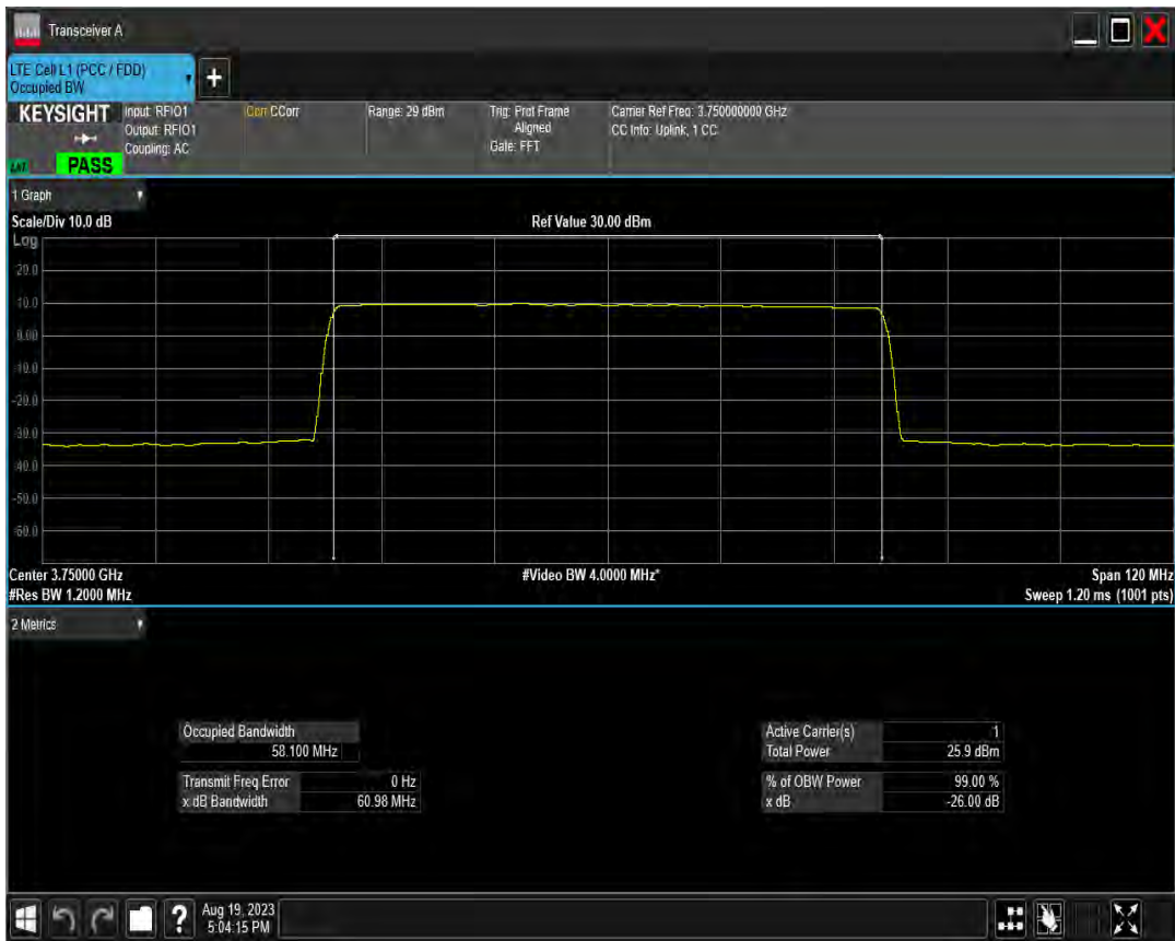
n78(3700-3800) SCS=30kHz DFT 64QAM BW=60MHz Channel=651332 RB=162@0
