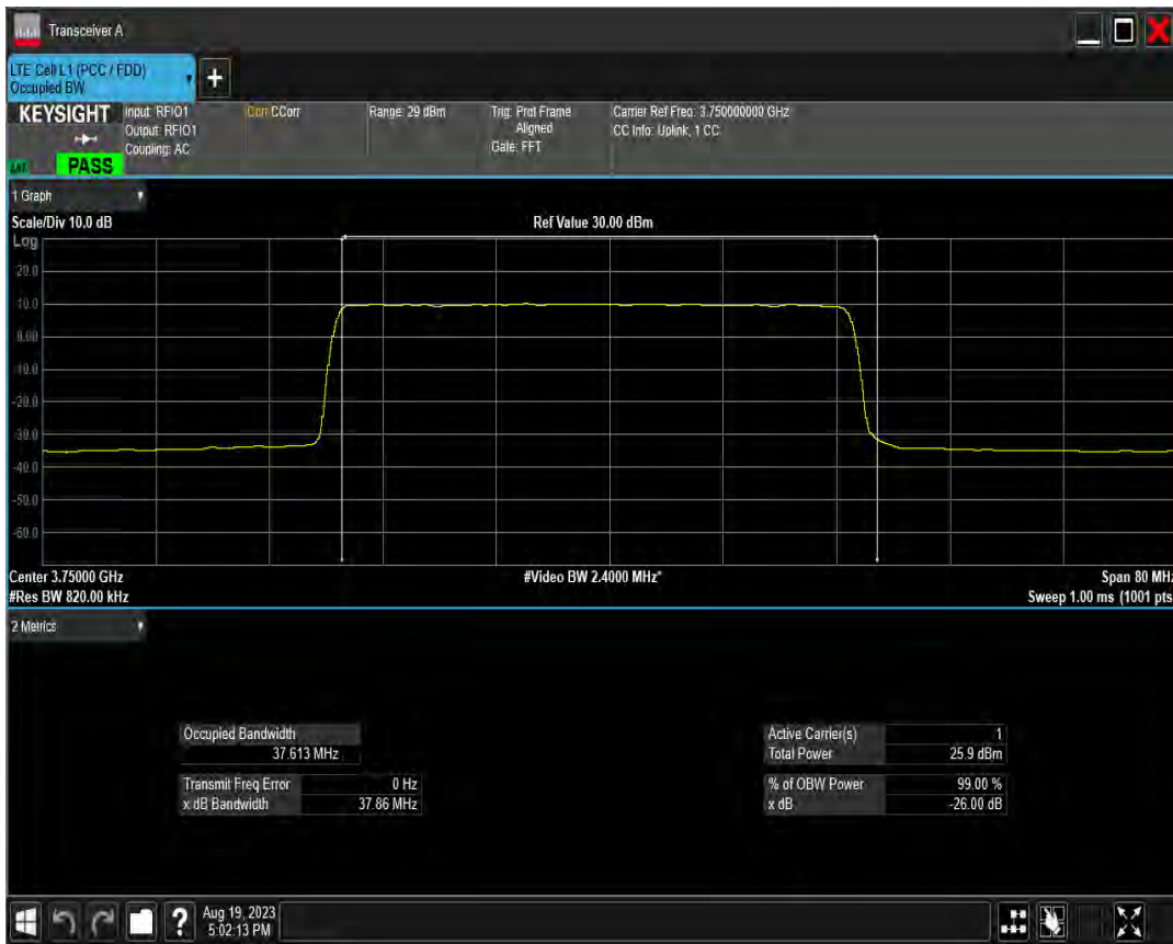
n78(3700-3800) SCS=30kHz DFT 256QAM BW=50MHz Channel=650000 RB=128@0
