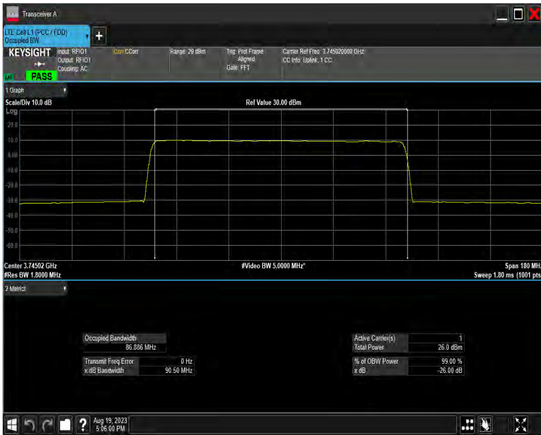
n78(3700-3800) SCS=30kHz DFT 64QAM BW=80MHz Channel=650000 RB=216@0
