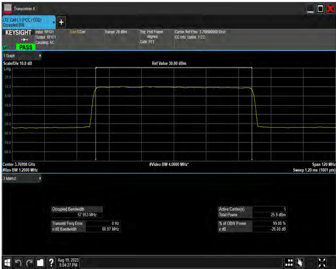
n78(3700-3800) SCS=30kHz DFT BPSK BW=60MHz Channel=648668 RB=162@0
