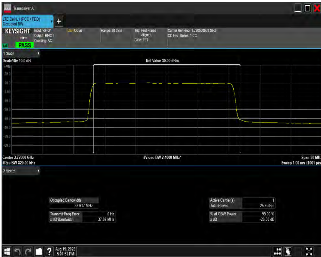
n78(3700-3800) SCS=30kHz DFT 256QAM BW=40MHz Channel=650000 RB=100@0
