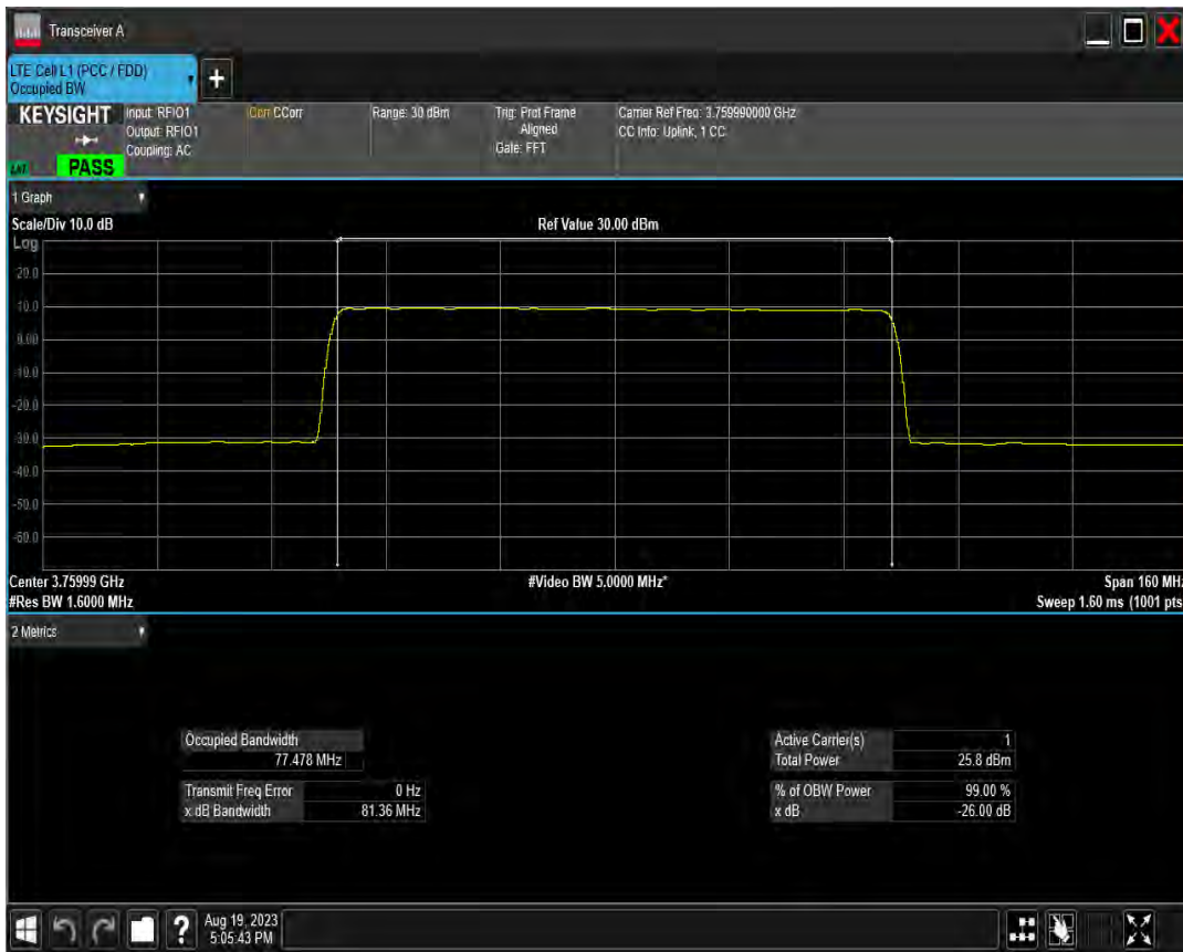
n78(3700-3800) SCS=30kHz DFT 256QAM BW=90MHz Channel=649668 RB=240@0
