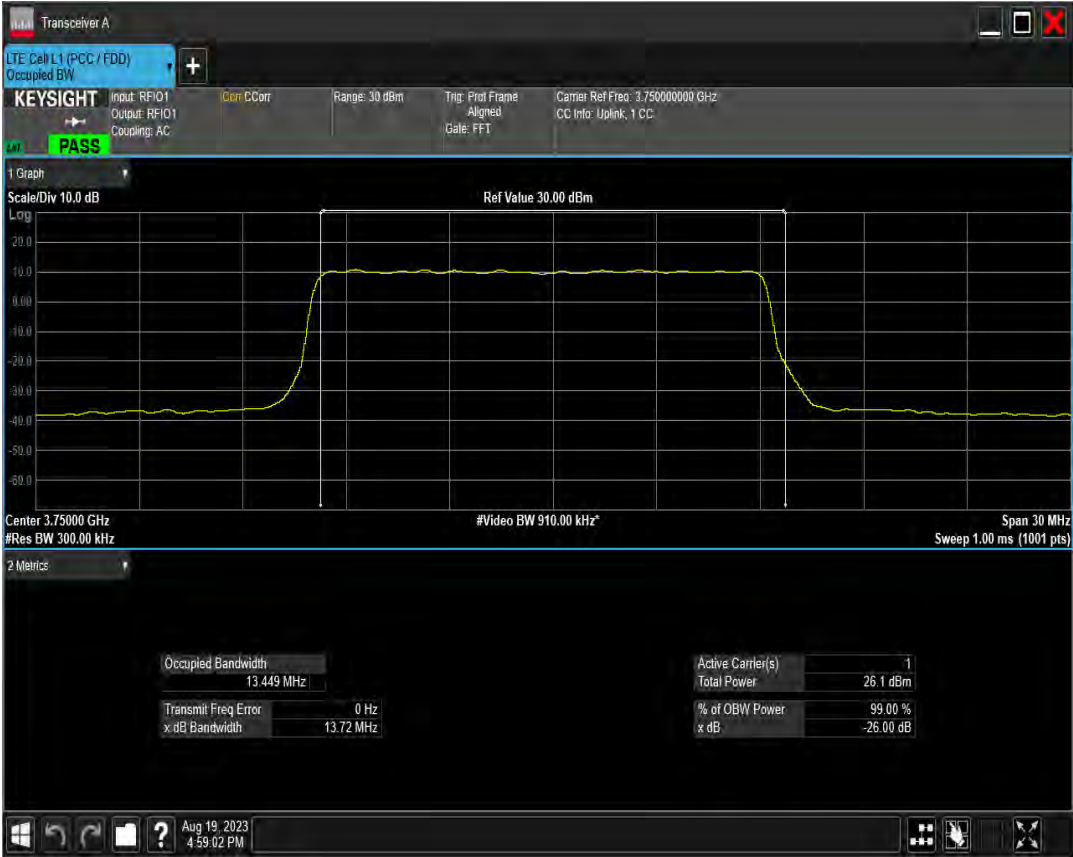
n78(3700-3800) SCS=30kHz DFT 64QAM BW=15MHz Channel=652832 RB=36@0
