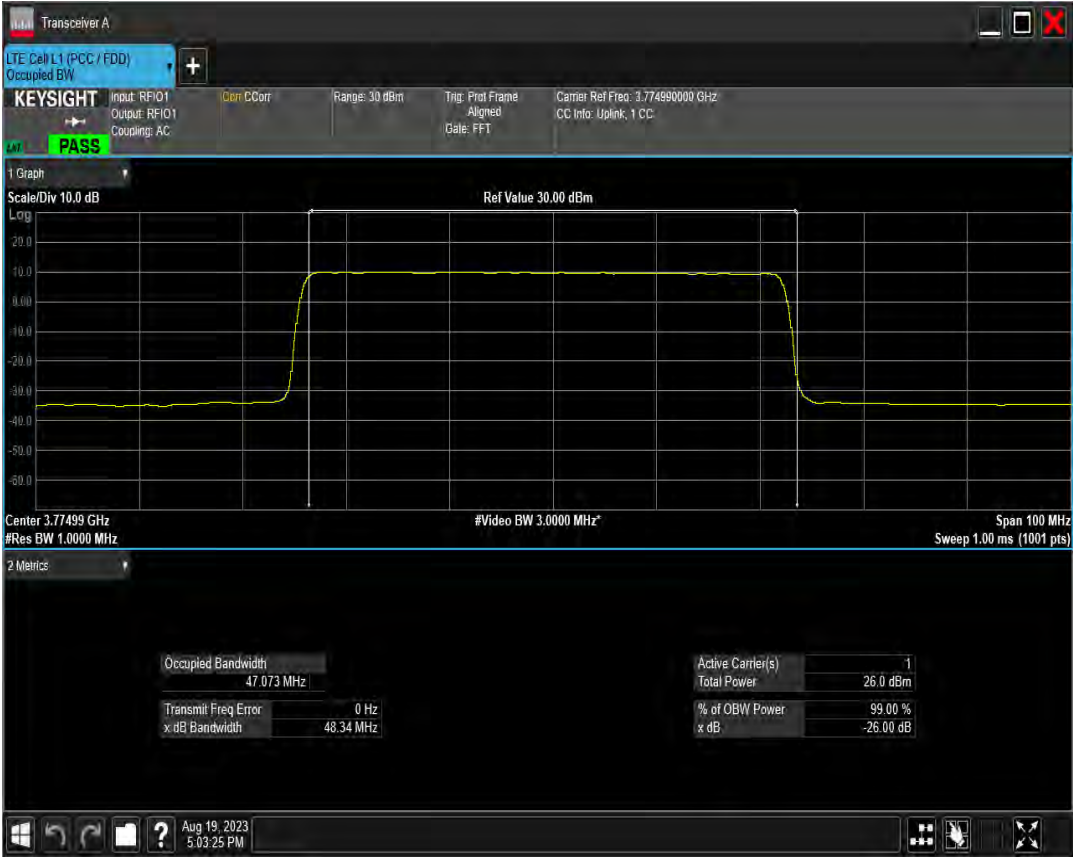
n78(3700-3800) SCS=30kHz DFT BPSK BW=40MHz Channel=652000 RB=100@0
