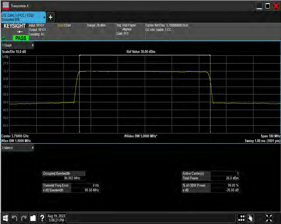
n78(3700-3800) SCS=30kHz DFT 64QAM BW=90MHz Channel=649668 RB=240@0
