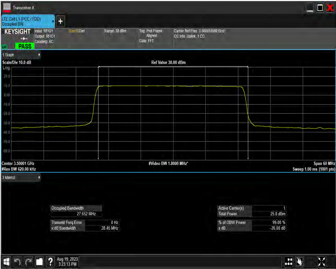
n78(3450-3550) SCS=30kHz DFT QPSK BW=30MHz Channel=631000 RB=75@0
