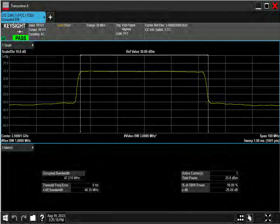
n78(3450-3550) SCS=30kHz DFT QPSK BW=50MHz Channel=635000 RB=128@0
