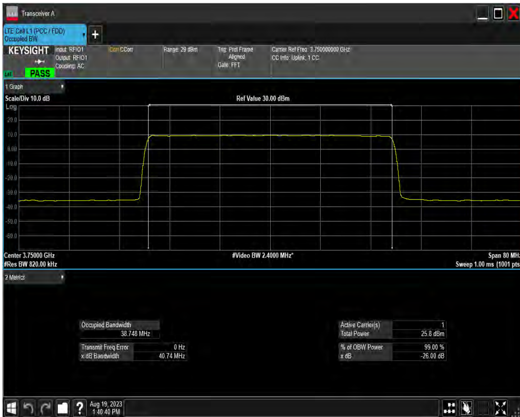
n78(3700-3800) SCS=15kHz DFT BPSK BW=30MHz Channel=652332 RB=160@0
