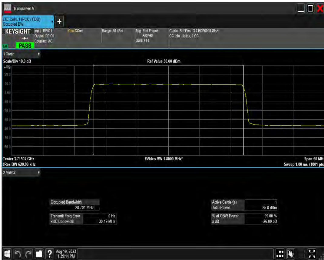
n78(3700-3800) SCS=15kHz DFT BPSK BW=30MHz Channel=650000 RB=160@0
