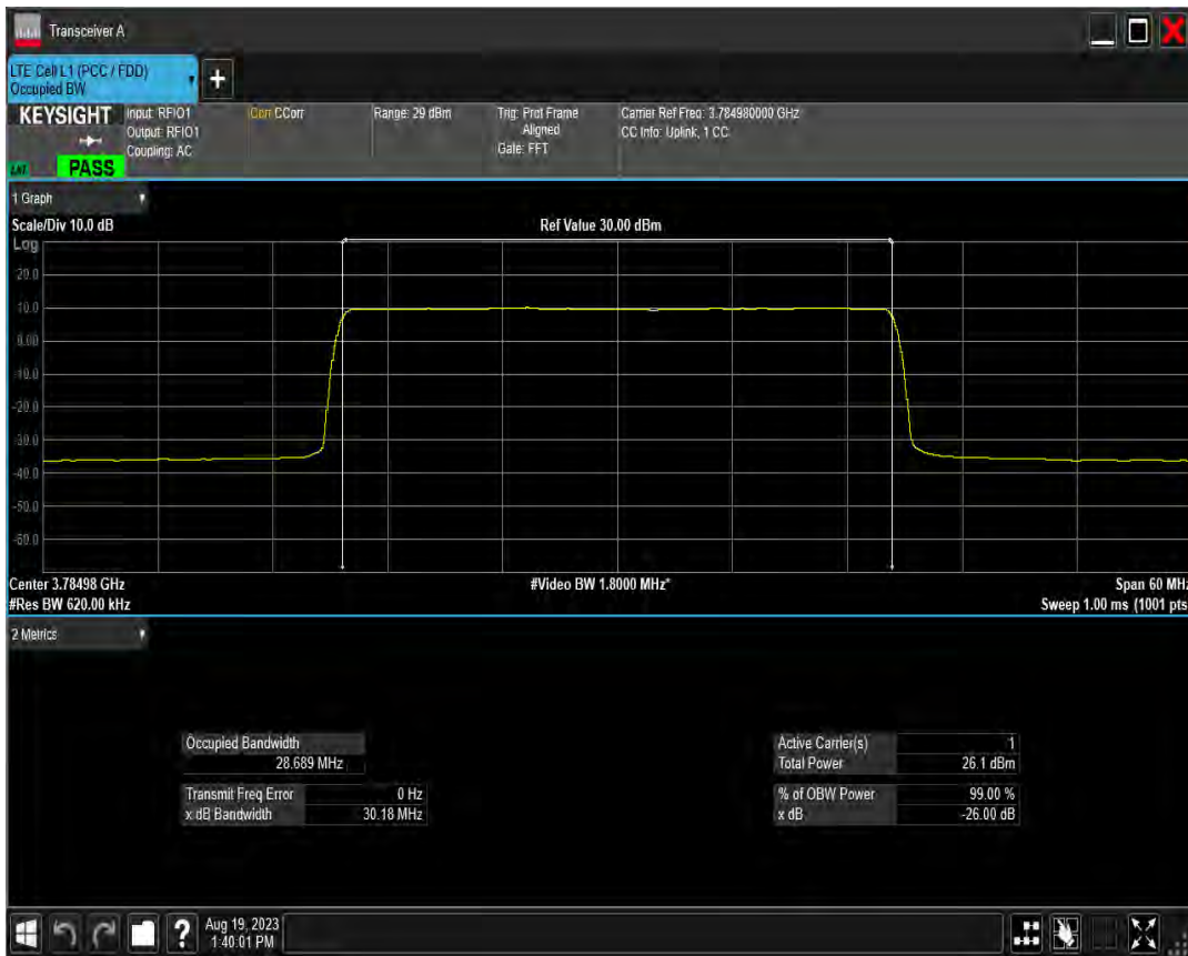
n78(3700-3800) SCS=15kHz DFT QPSK BW=40MHz Channel=648000 RB=216@0
