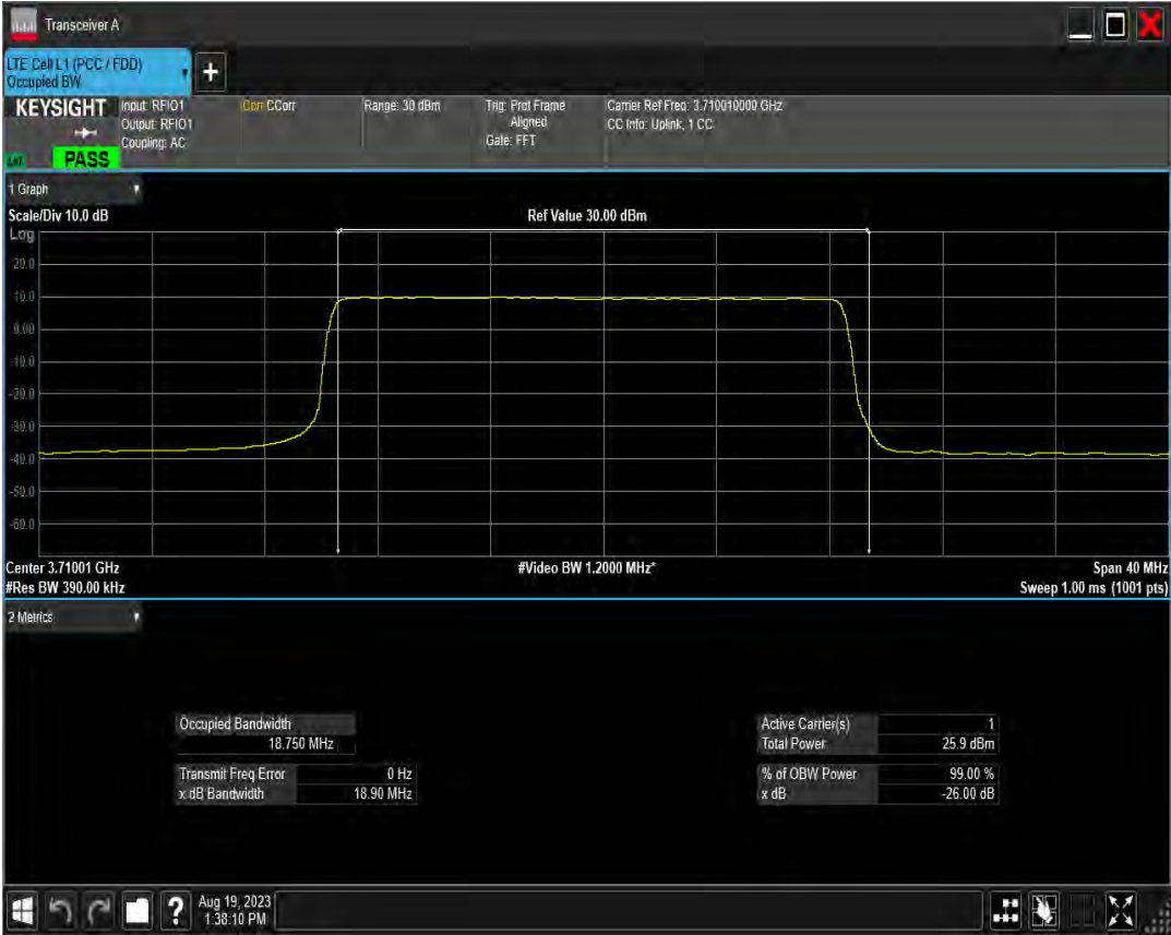
n78(3700-3800) SCS=15kHz DFT BPSK BW=20MHz Channel=650000 RB=100@0
