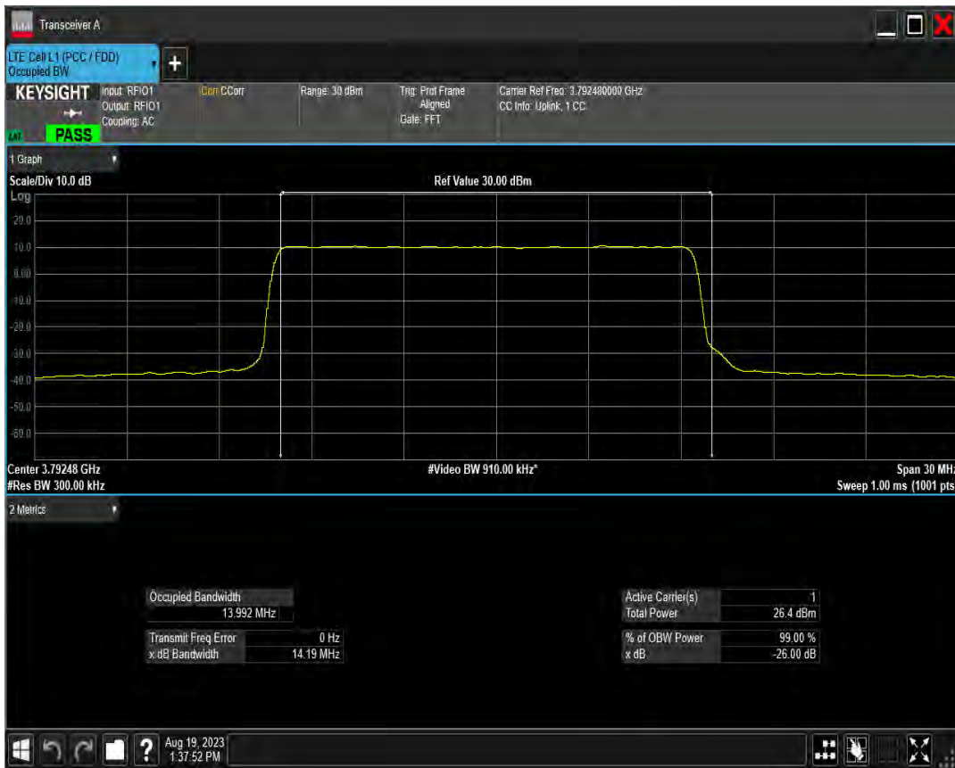
n78(3700-3800) SCS=15kHz DFT QPSK BW=20MHz Channel=650000 RB=100@0
