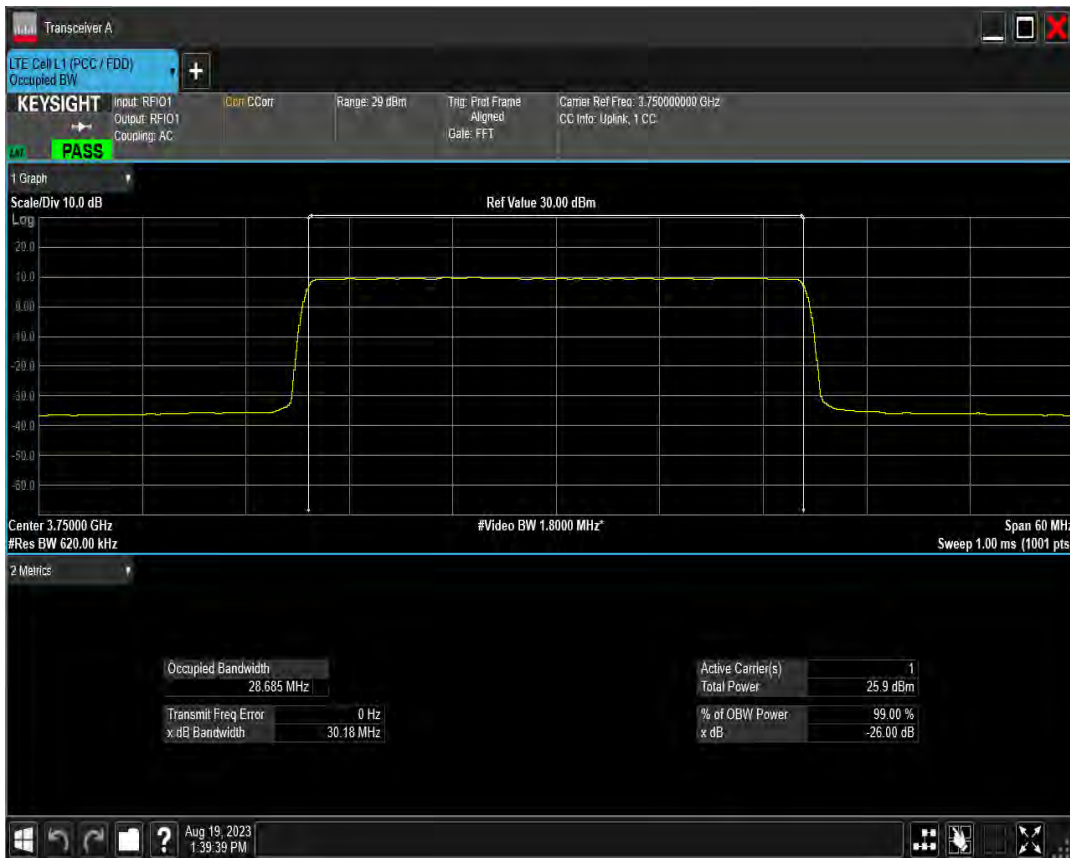
n78(3700-3800) SCS=15kHz DFT QPSK BW=30MHz Channel=652332 RB=160@0
