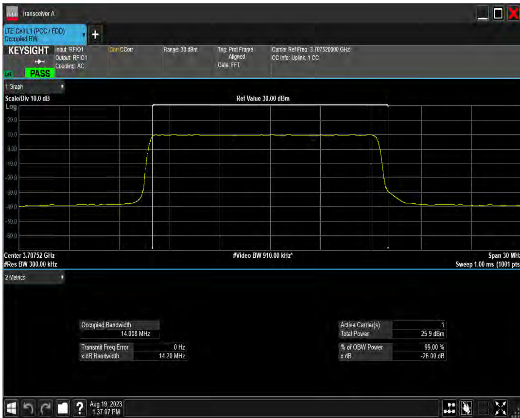
n78(3700-3800) SCS=15kHz DFT BPSK BW=15MHz Channel=650000 RB=75@0
