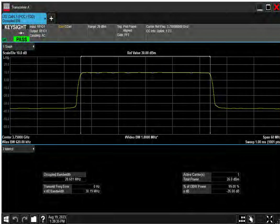
n78(3700-3800) SCS=15kHz DFT BPSK BW=40MHz Channel=648000 RB=216@0
