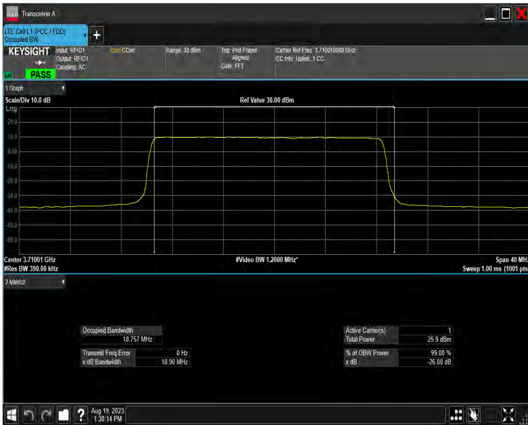
n78(3700-3800) SCS=15kHz DFT QPSK BW=20MHz Channel=652666 RB=100@0
