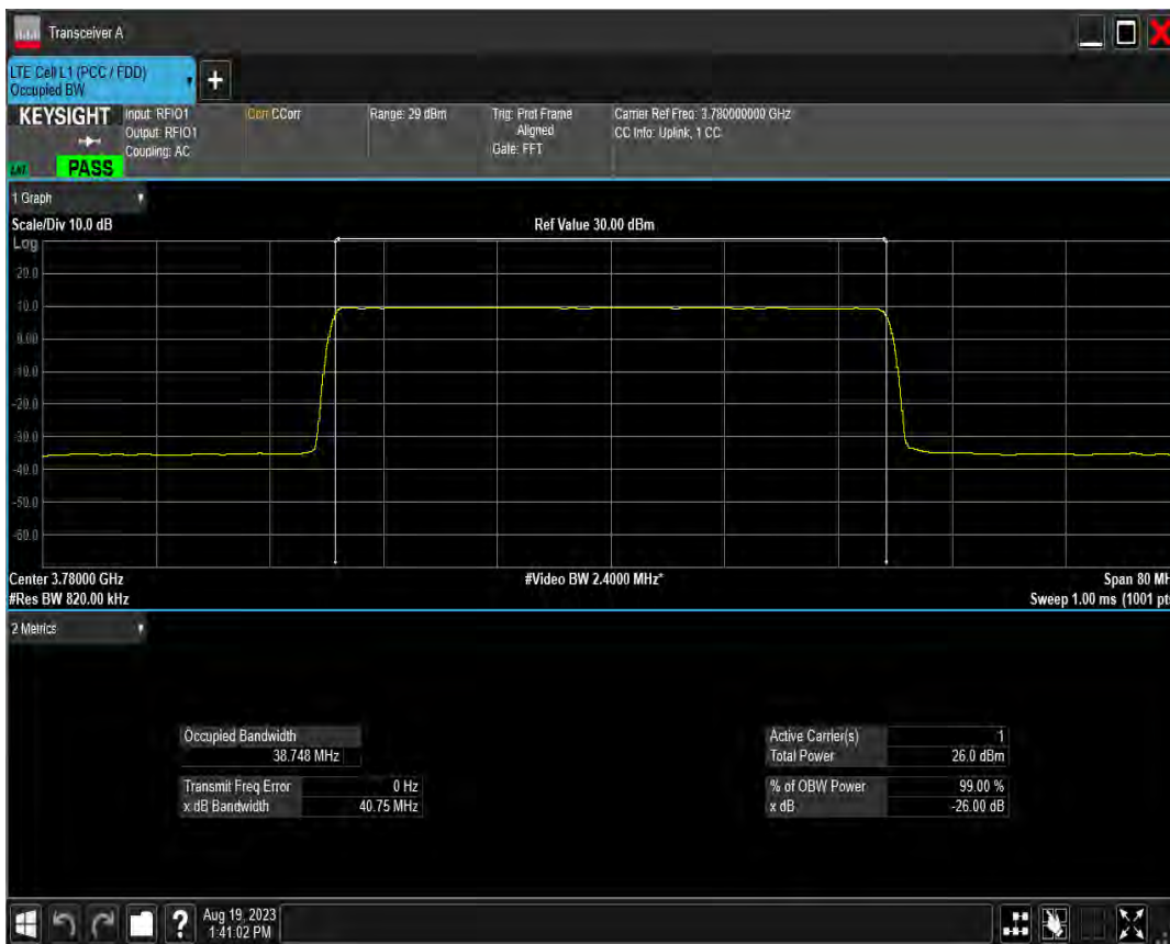
n78(3700-3800) SCS=15kHz DFT BPSK BW=50MHz Channel=648334 RB=270@0
