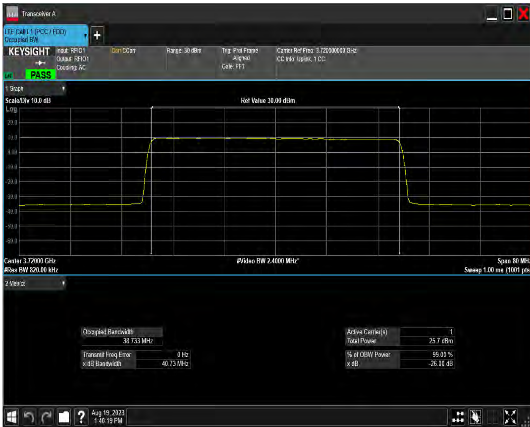
n78(3700-3800) SCS=15kHz DFT BPSK BW=40MHz Channel=650000 RB=216@0
