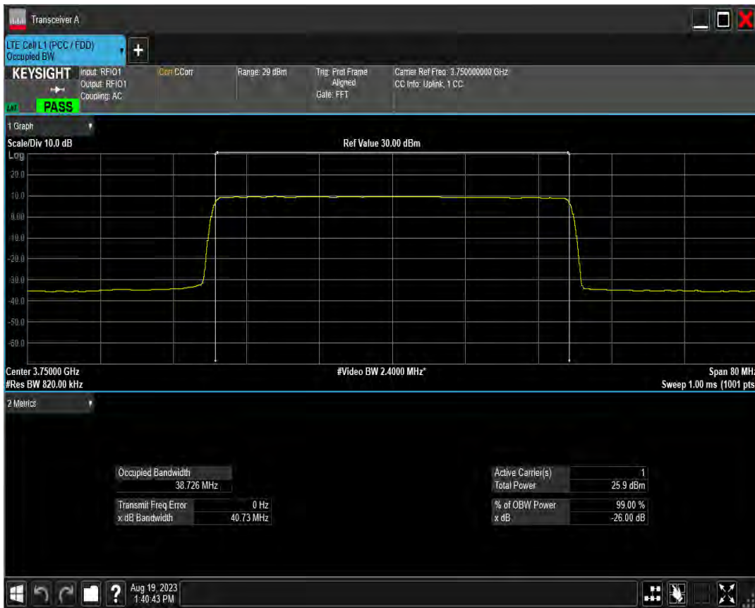
n78(3700-3800) SCS=15kHz DFT QPSK BW=50MHz Channel=648334 RB=270@0
