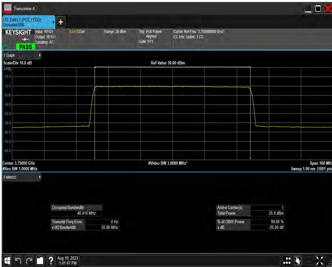
n78(3700-3800) SCS=15kHz DFT QPSK BW=40MHz Channel=652000 RB=216@0
