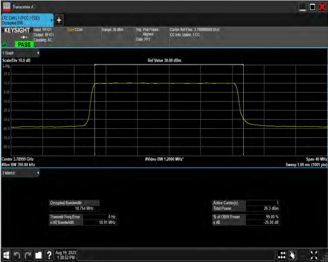
n78(3700-3800) SCS=15kHz DFT BPSK BW=30MHz Channel=647668 RB=160@0
