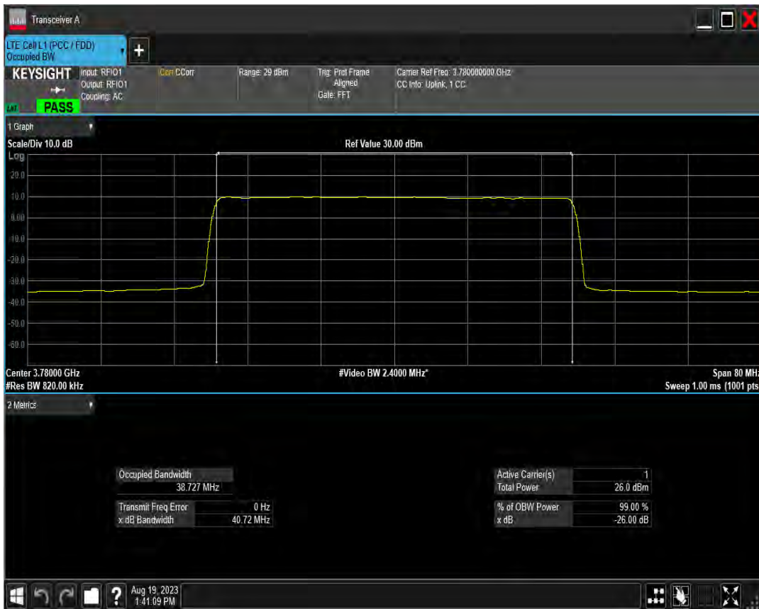
n78(3700-3800) SCS=15kHz DFT 64QAM BW=50MHz Channel=648334 RB=270@0
