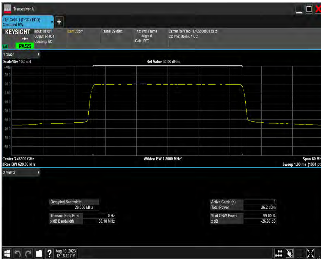
n78(3450-3550) SCS=15kHz DFT QPSK BW=40MHz Channel=631334 RB=216@0
