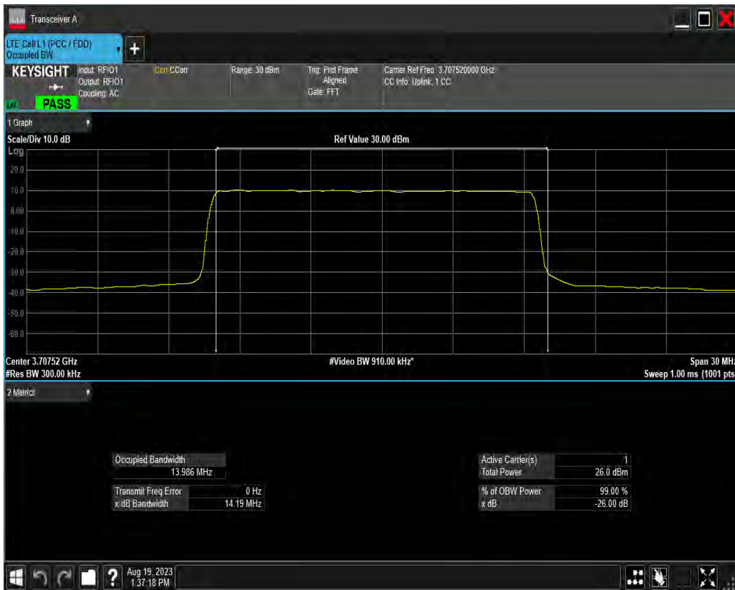
n78(3700-3800) SCS=15kHz DFT 256QAM BW=20MHz Channel=650000 RB=100@0
