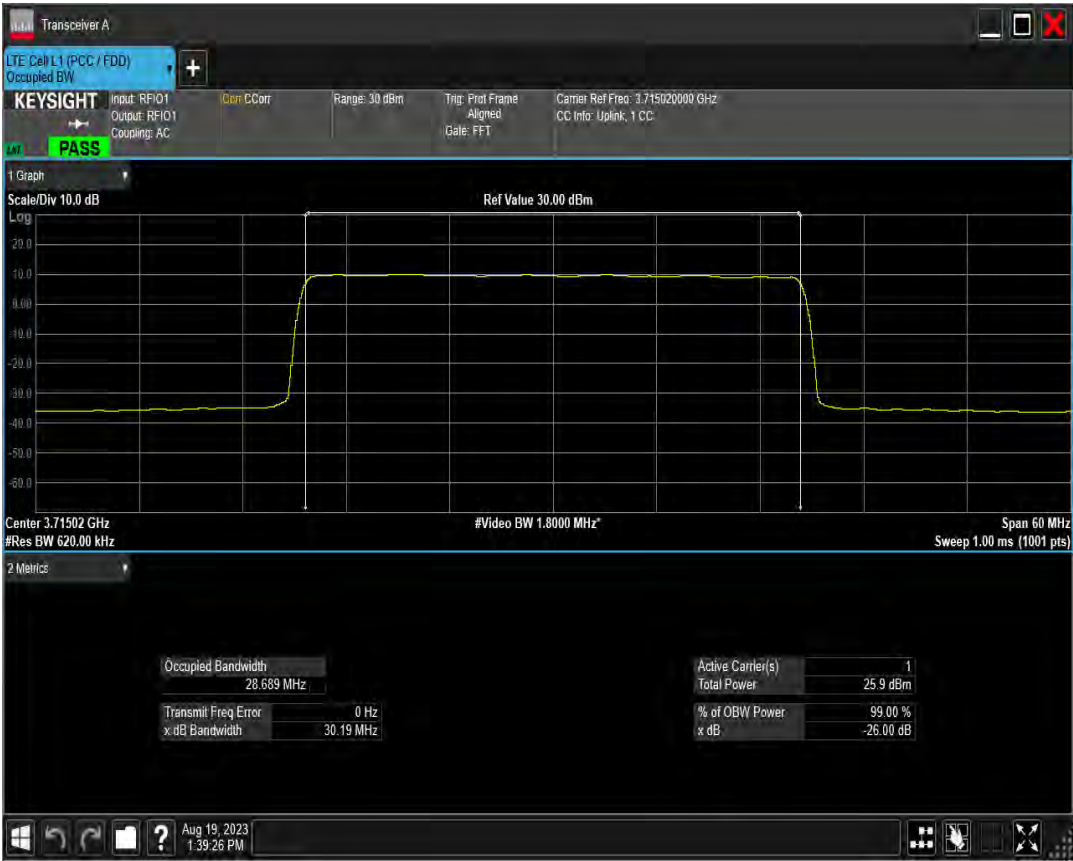
n78(3700-3800) SCS=15kHz DFT 256QAM BW=30MHz Channel=650000 RB=160@0
