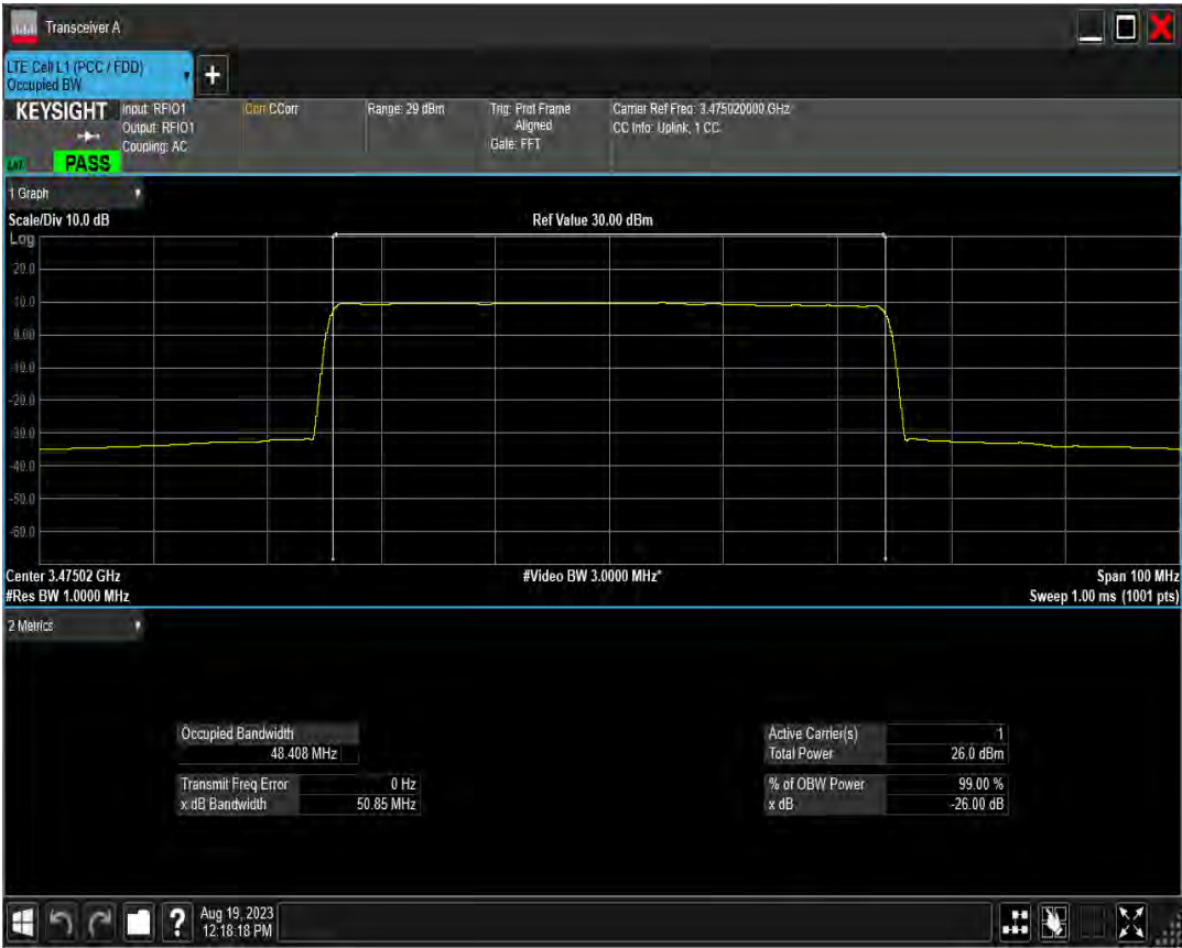
n78(3450-3550) SCS=15kHz DFT QPSK BW=50MHz Channel=633334 RB=270@0
