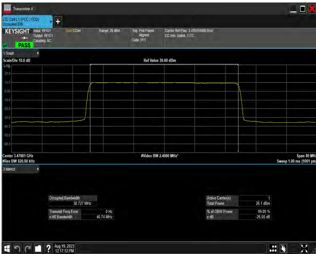
n78(3450-3550) SCS=15kHz DFT BPSK BW=40MHz Channel=633334 RB=216@0
