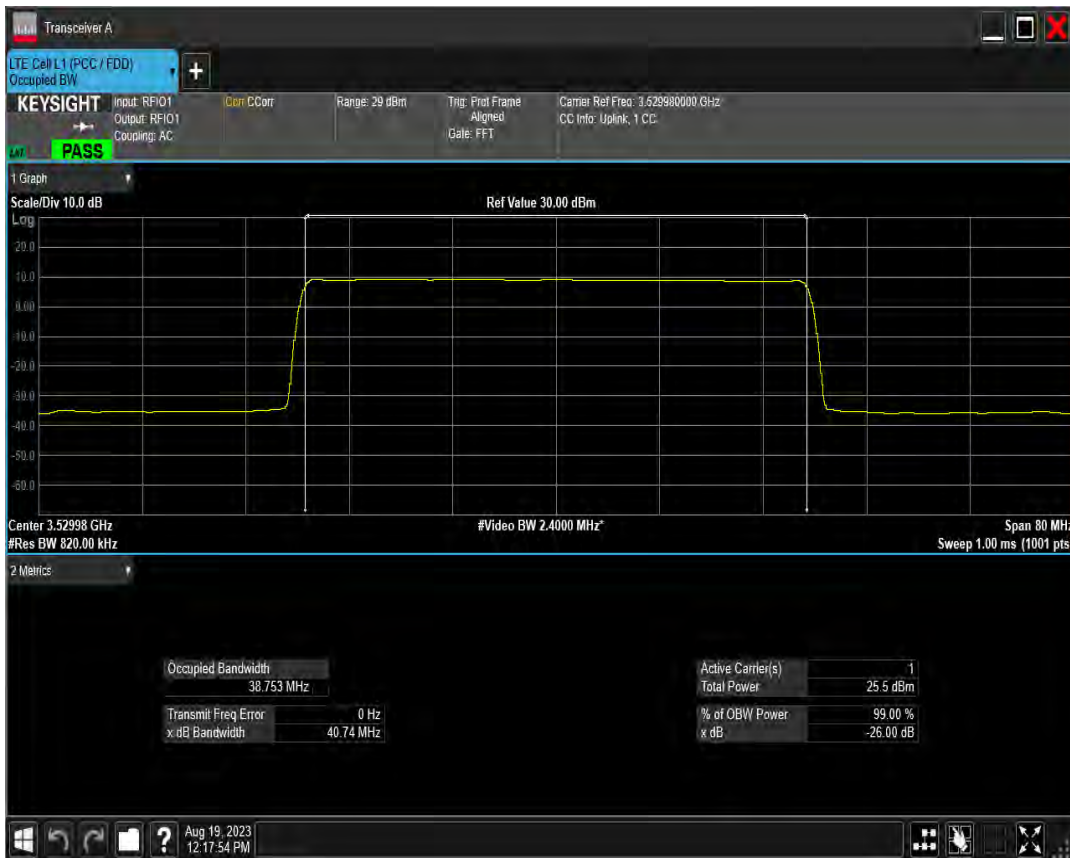
n78(3450-3550) SCS=15kHz DFT BPSK BW=50MHz Channel=635000 RB=270@0
