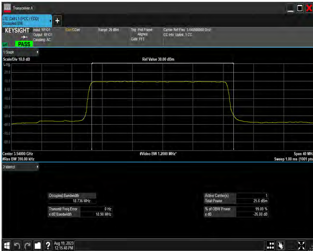
n78(3450-3550) SCS=15kHz DFT BPSK BW=30MHz Channel=631000 RB=160@0
