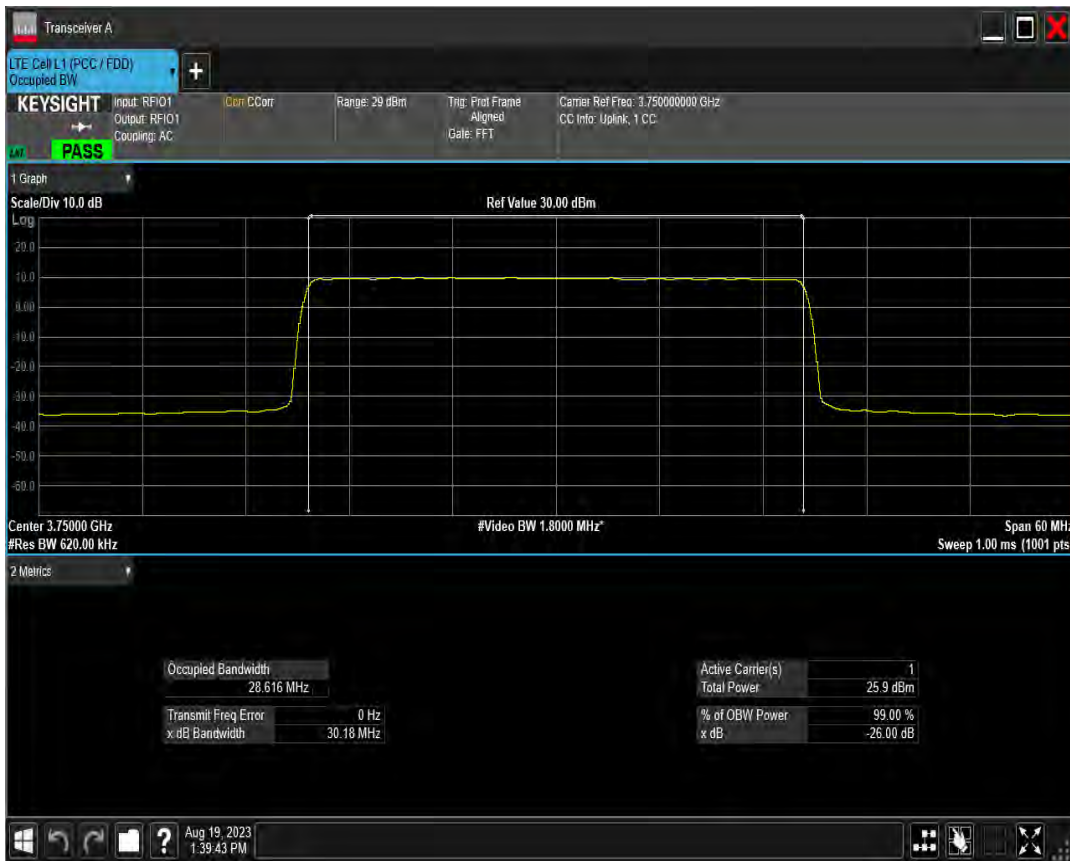
n78(3700-3800) SCS=15kHz DFT 64QAM BW=30MHz Channel=647668 RB=160@0
