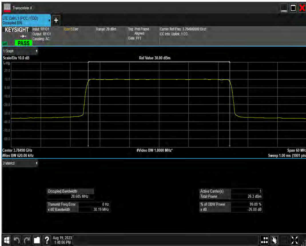
n78(3700-3800) SCS=15kHz DFT 64QAM BW=40MHz Channel=648000 RB=216@0
