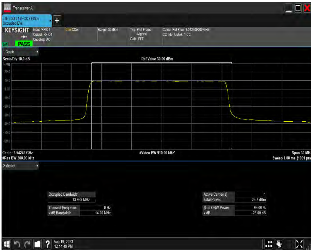
n78(3450-3550) SCS=15kHz DFT QPSK BW=20MHz Channel=630668 RB=100@0
