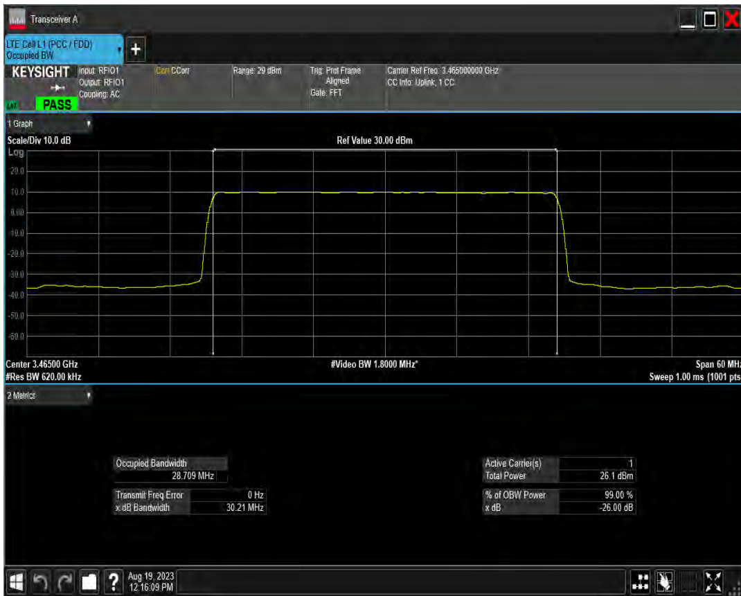
n78(3450-3550) SCS=15kHz DFT BPSK BW=30MHz Channel=633334 RB=160@0
