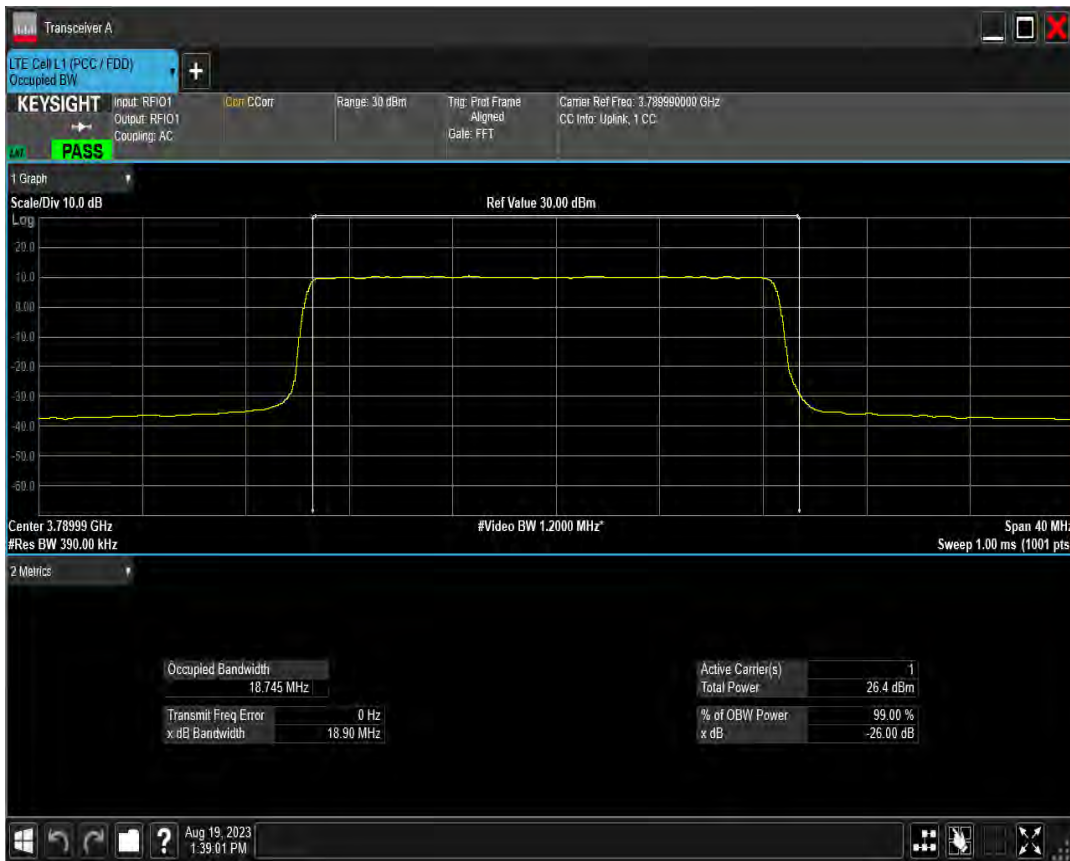
n78(3700-3800) SCS=15kHz DFT 64QAM BW=20MHz Channel=650000 RB=100@0
