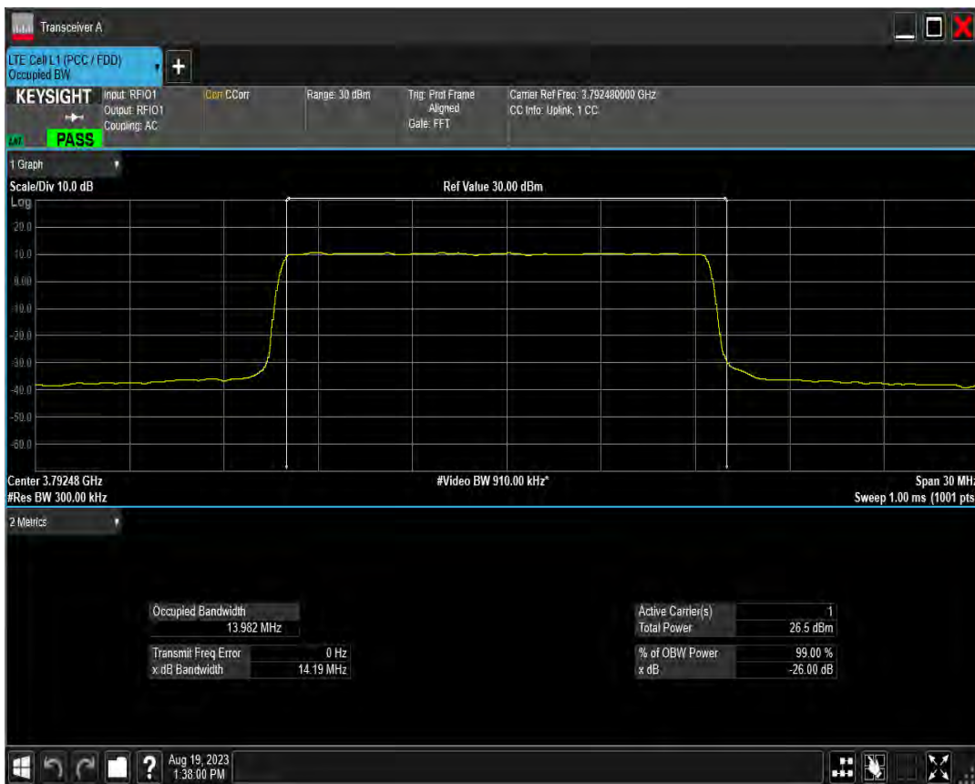
n78(3700-3800) SCS=15kHz DFT 256QAM BW=15MHz Channel=650000 RB=75 @0
