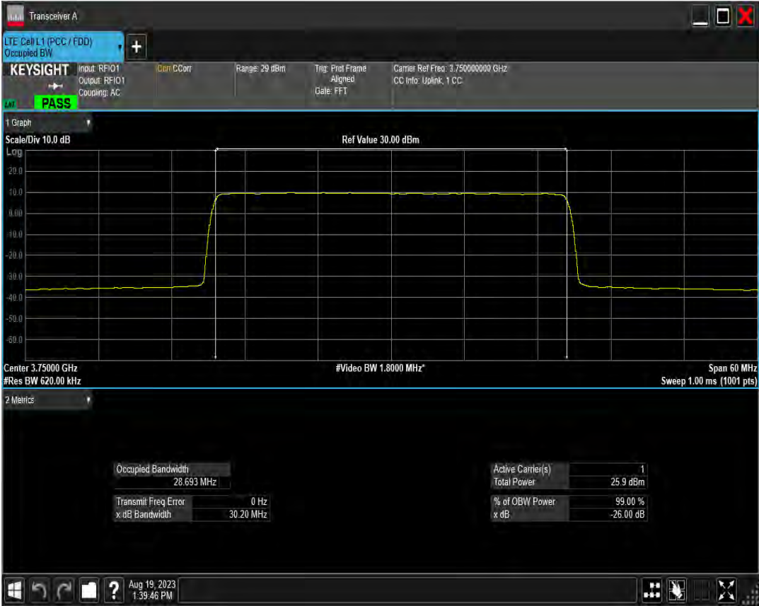
n78(3700-3800) SCS=15kHz DFT 256QAM BW=30MHz Channel=652332 RB=160@0
