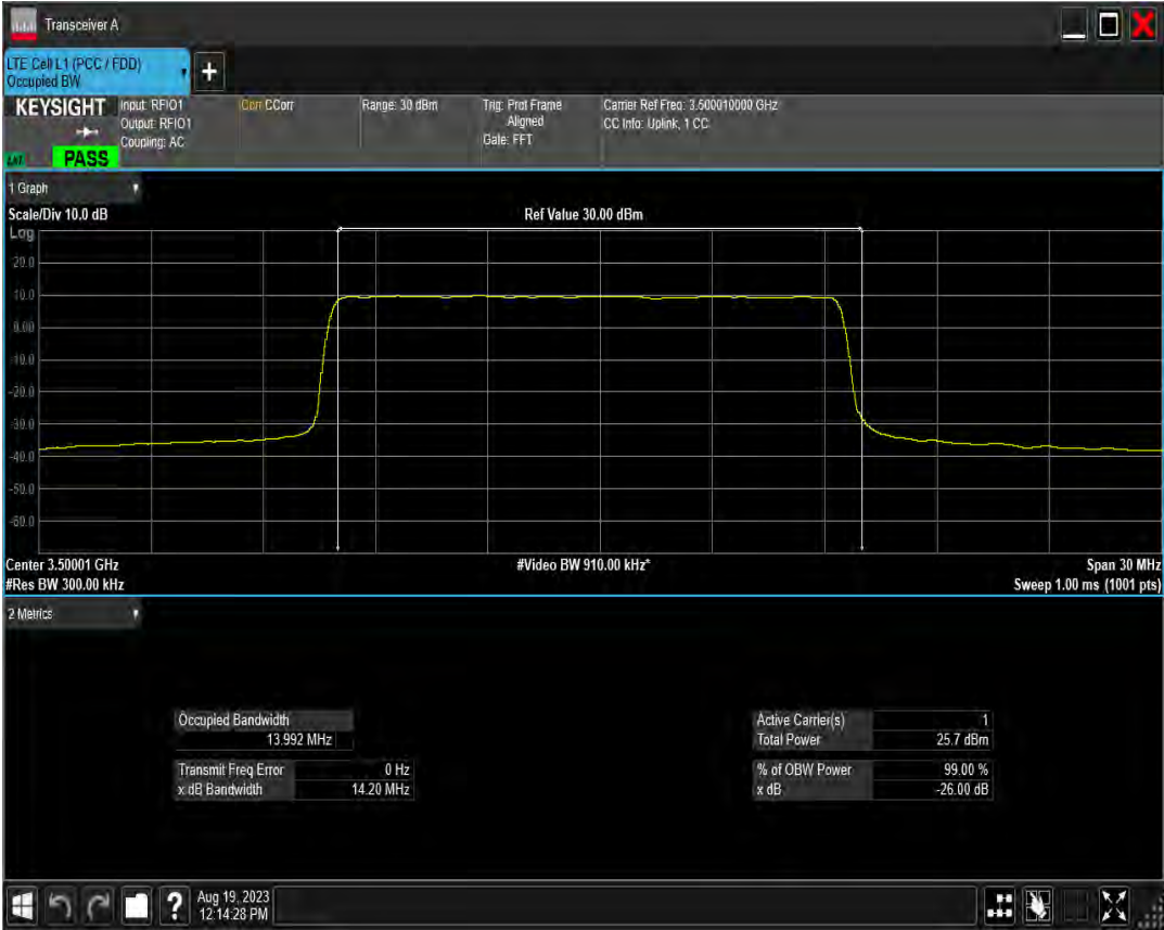
n78(3450-3550) SCS=15kHz DFT QPSK BW=15MHz Channel=636166 RB=75@0
