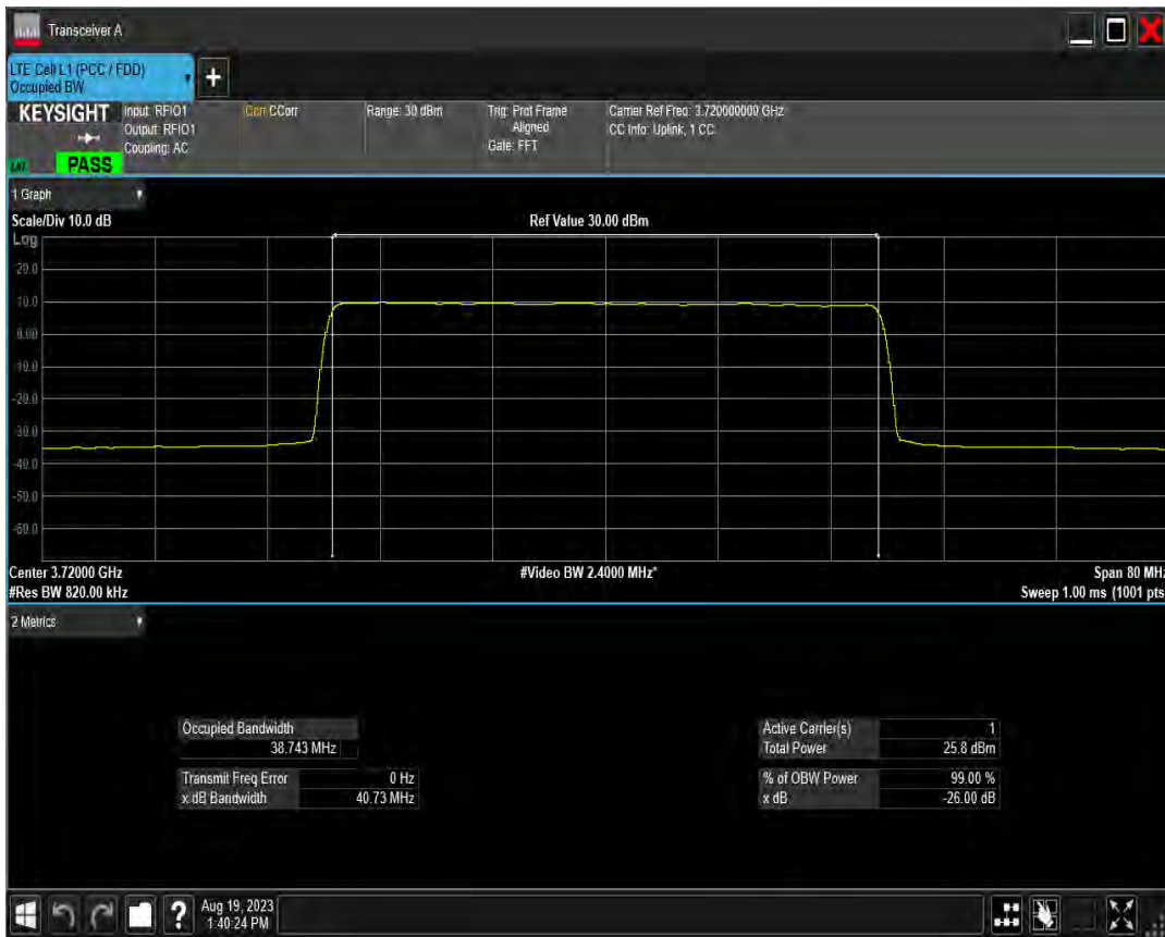
n78(3700-3800) SCS=15kHz DFT 16QAM BW=40MHz Channel=652000 RB=216@0
