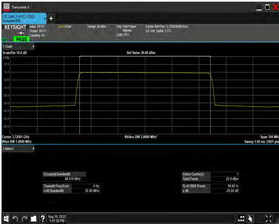
n78(3700-3800) SCS=15kHz DFT 16QAM BW=50MHz Channel=650000 RB=270@0
