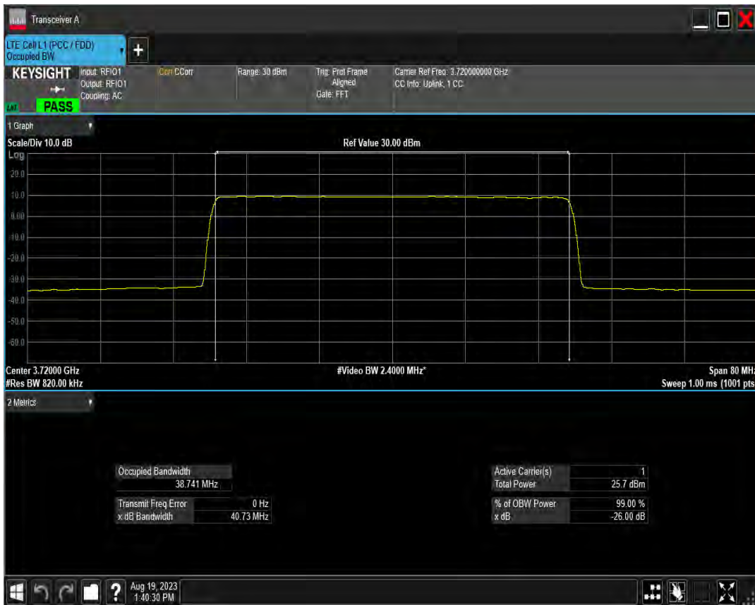
n78(3700-3800) SCS=15kHz DFT 256QAM BW=40MHz Channel=650000 RB=216@0
