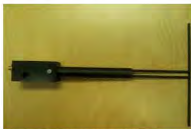
Figure 1 – MVG COMOSAR Validation Dipole
