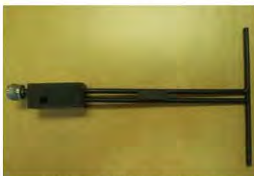
Figure 1 – MVG COMOSAR Validation Dipole
