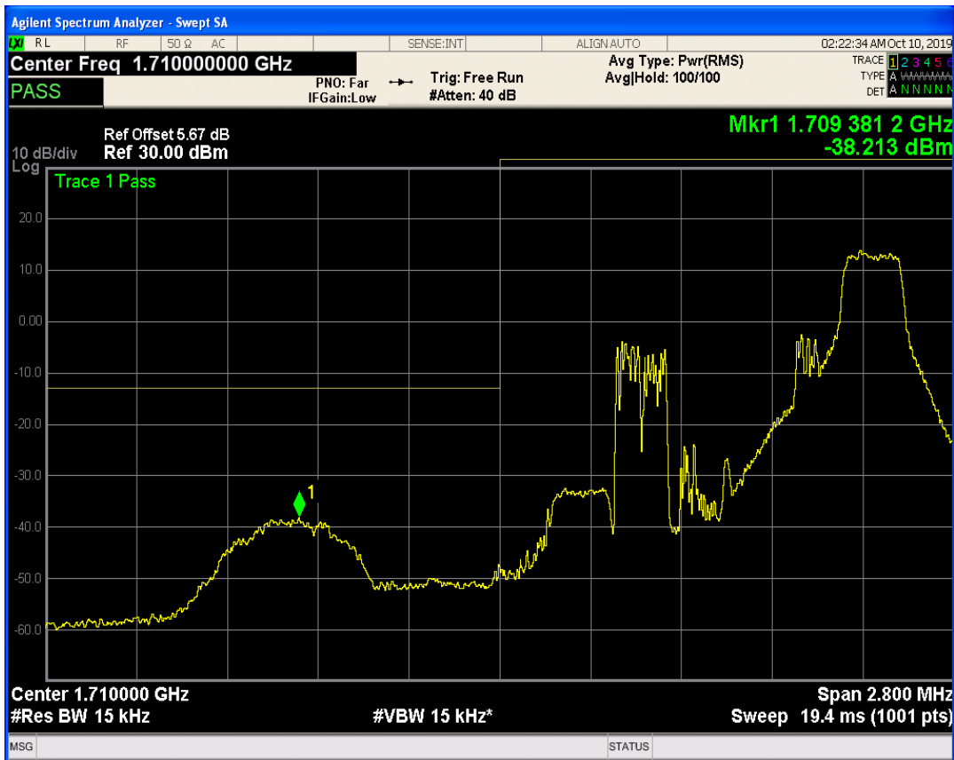
LTE Band4 QAM16 BW=1.4MHz Channel=19957 RB Size=1 Position=#0
