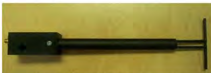
Figure 1 – MVG COMOSAR Validation Dipole
