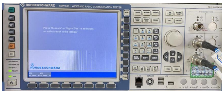
CMW 500 (2G/3G/4G Test Equipment)
