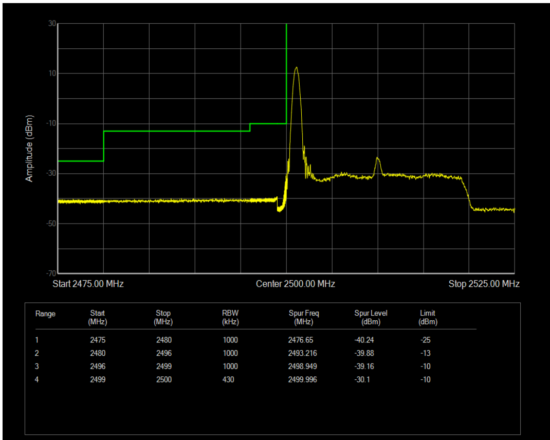
Band7 QPSK BW=20MHz Channel=20850 RB Size=1 Position=#Max
