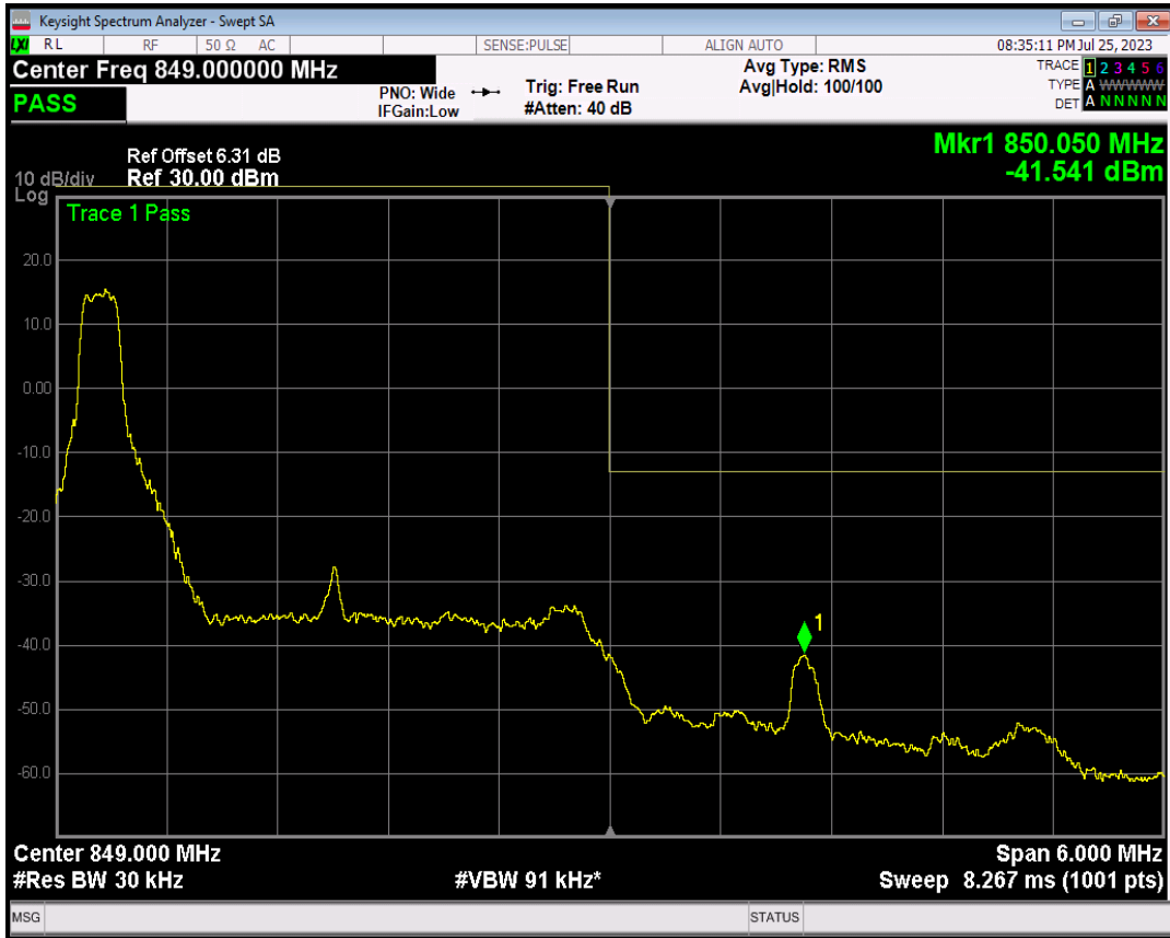
Band5 16QAM BW=3MHz Channel=20635 RB Size=1 Position=#Max
