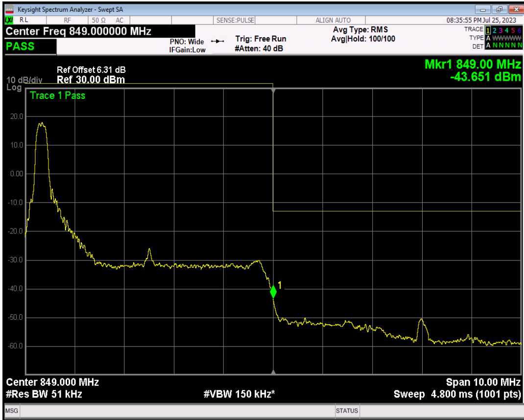
Band5 16QAM BW=5MHz Channel=20625 RB Size=1 Position=#Max
