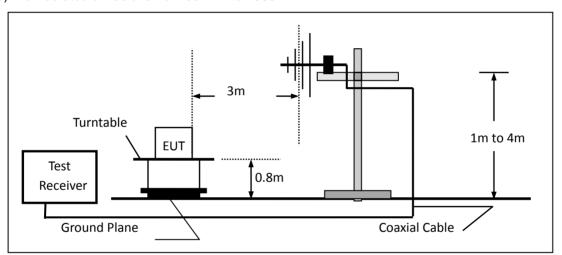
(c) For radiated emissions above 1000MHz
