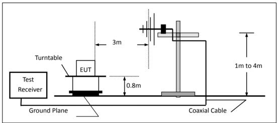
(c) For radiated emissions above 1000MHz
