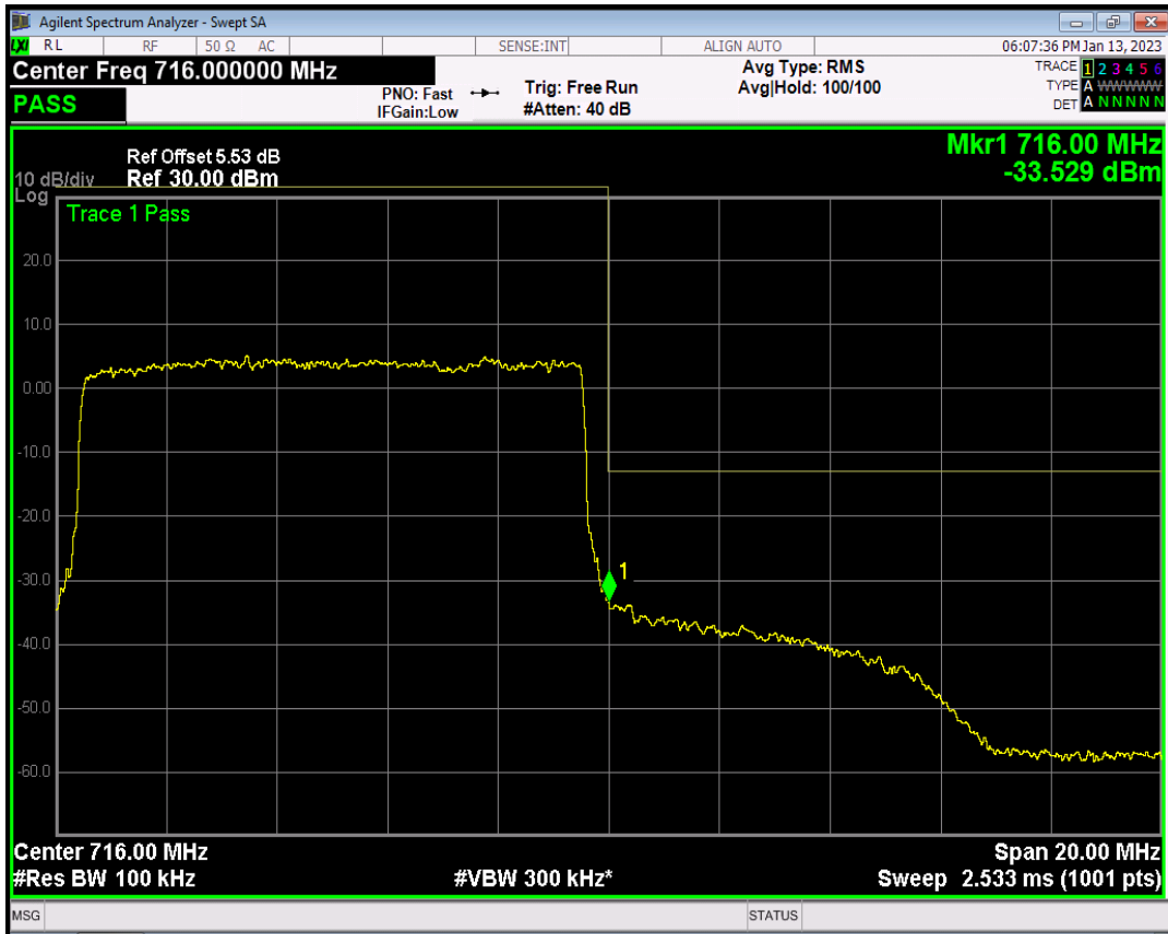
Band17 QAM16 BW=10MHz Channel=23800 RB Size=50 Position=#0
