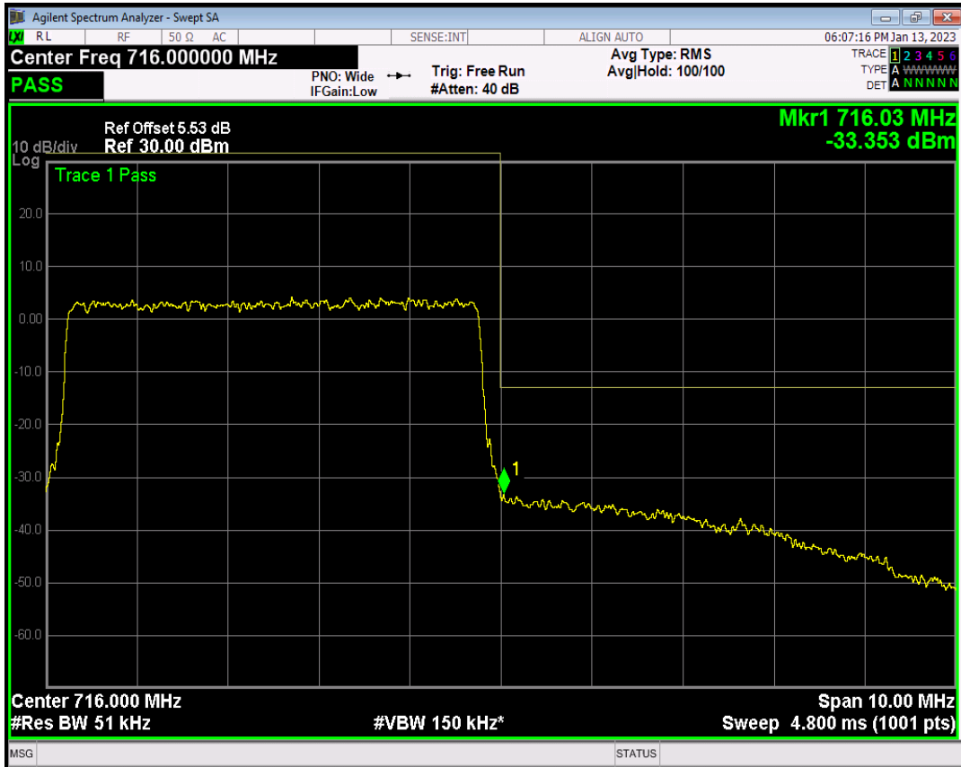
Band17 QPSK BW=10MHz Channel=23780 RB Size=50 Position=#0
