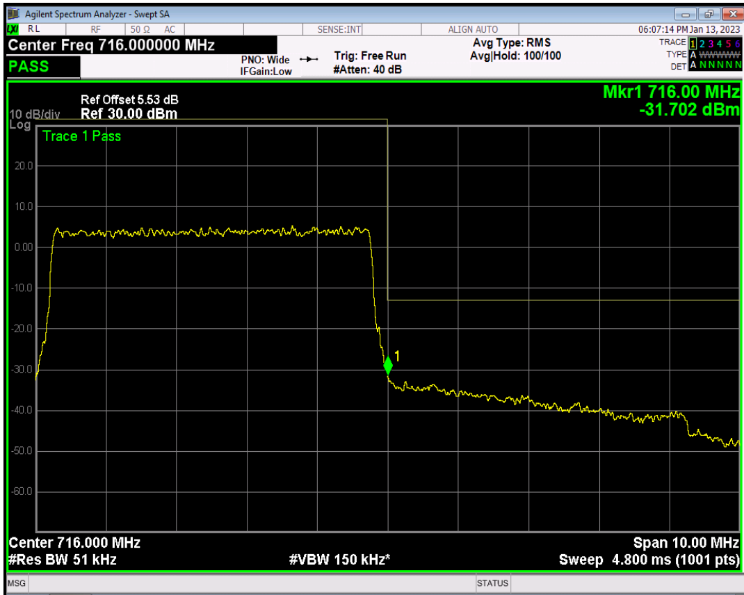
Band17 QAM16 BW=5MHz Channel=23825 RB Size=25 Position=#0
