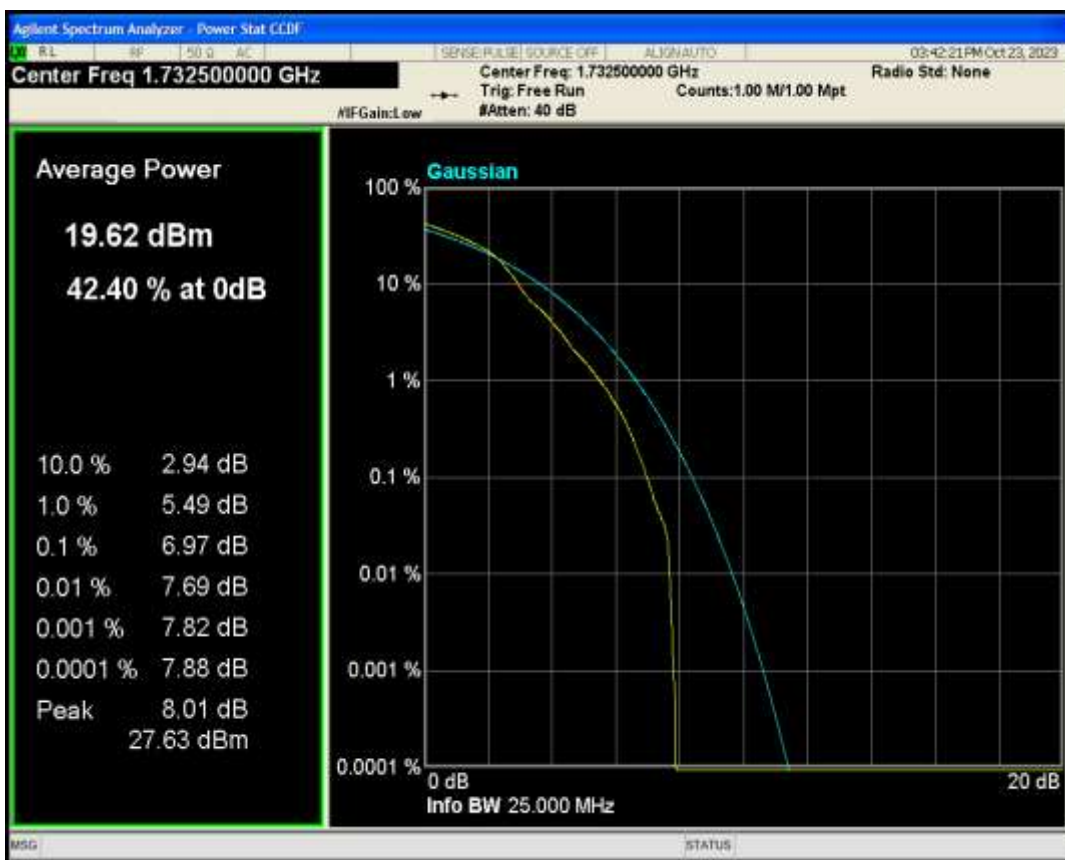
Band4 QPSK BW=5MHz Channel=20175 RB Size=1 Position=#0
