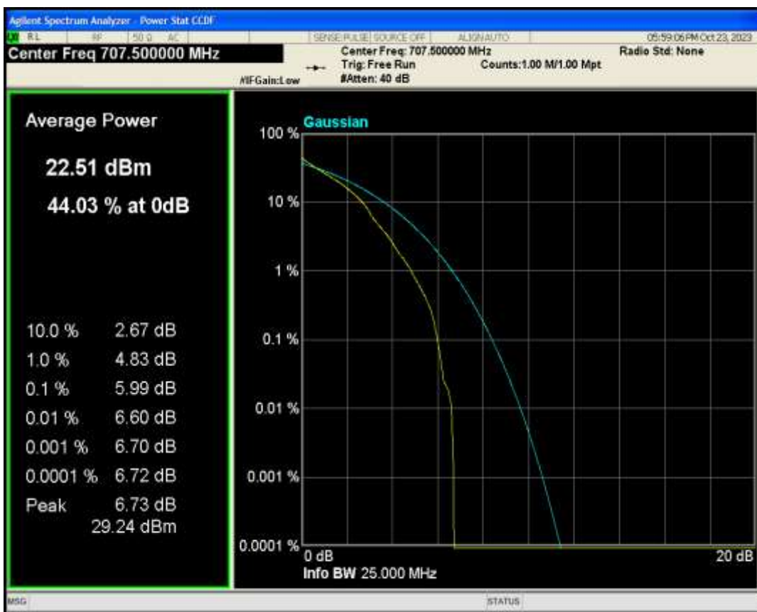
Band12 QAM16 BW=10MHz Channel=23095 RB Size=1 Position=#0
