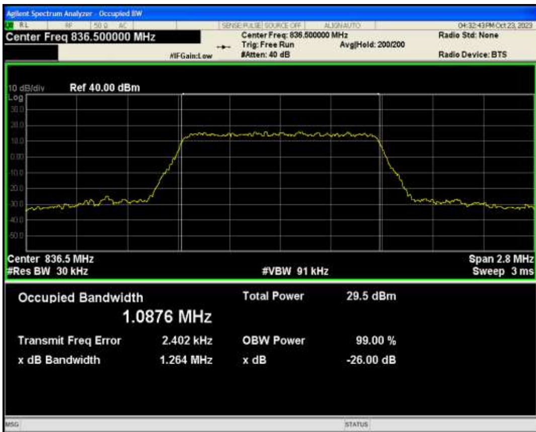
Band5 QAM16 BW=1.4MHz Channel=20525 RB Size=6 Position=#0
