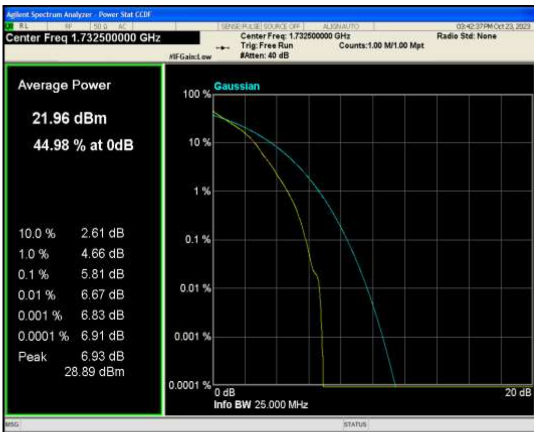
Band4 QAM16 BW=15MHz Channel=20175 RB Size=1 Position=#0
