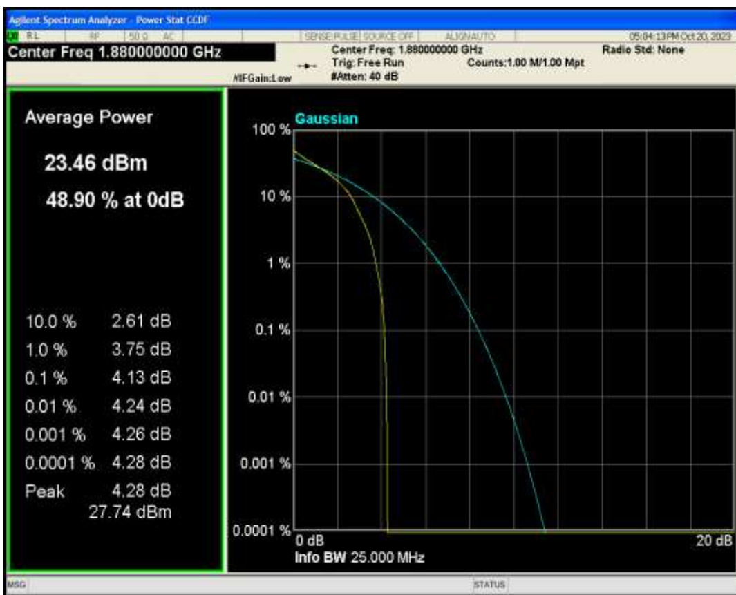
Band2 QAM16 BW=5MHz Channel=18900 RB Size=1 Position=#0
