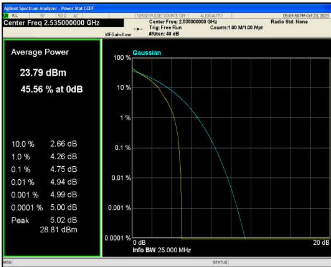
Band7 QAM16 BW=10MHz Channel=21100 RB Size=1 Position=#0
