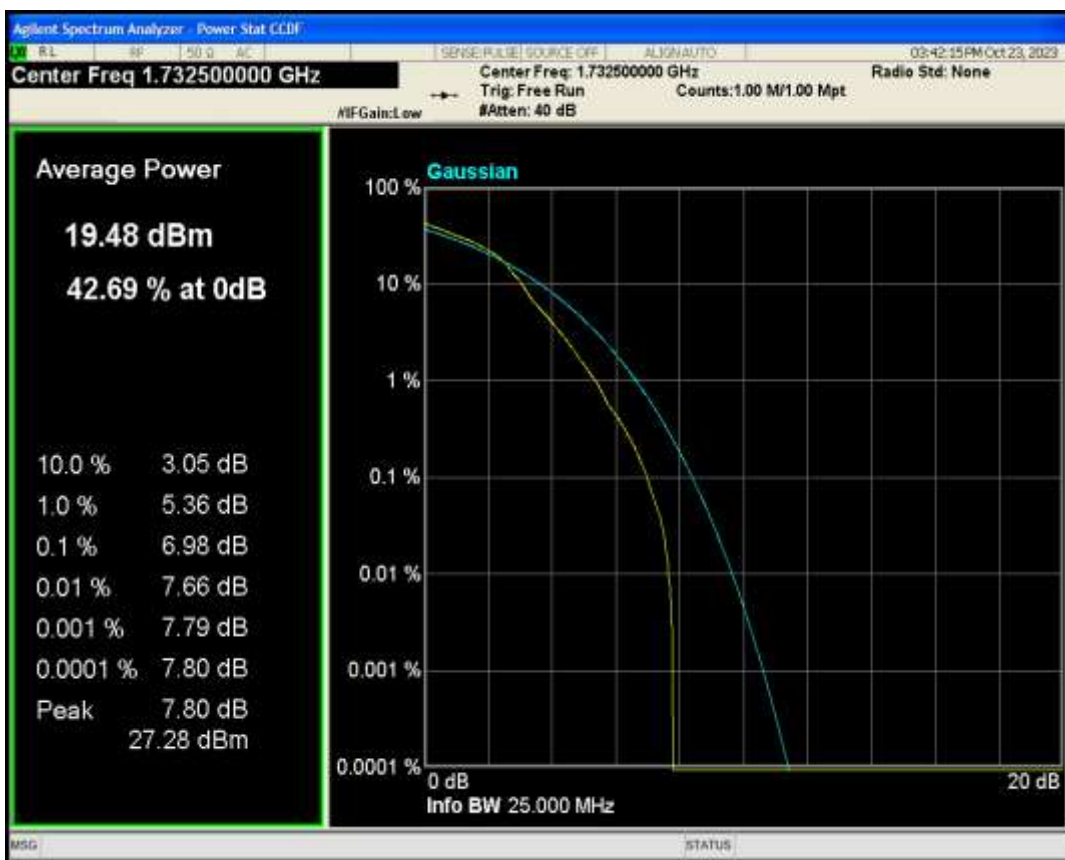
Band4 QPSK BW=3MHz Channel=20175 RB Size=1 Position=#0
