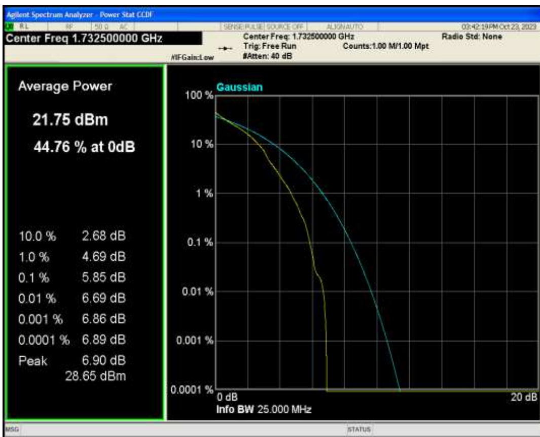
Band4 QAM16 BW=3MHz Channel=20175 RB Size=1 Position=#0
