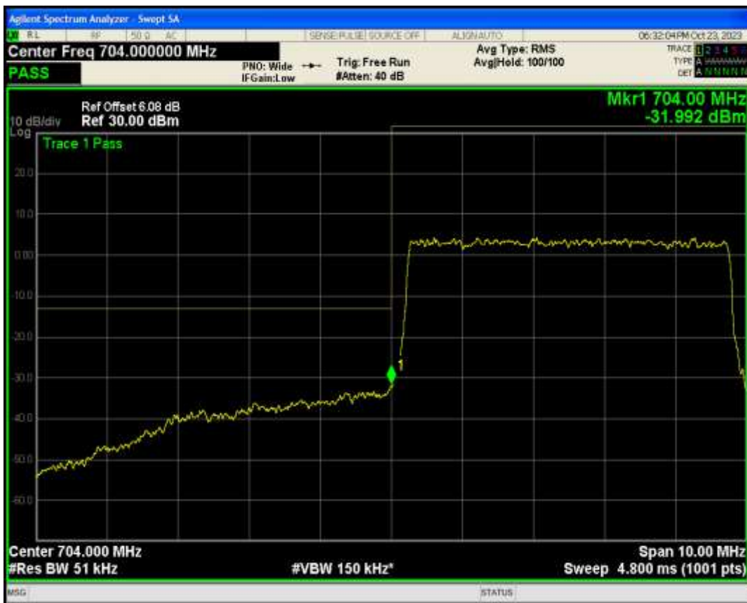
Band17 QAM16 BW=5MHz Channel=23755 RB Size=25 Position=#0
