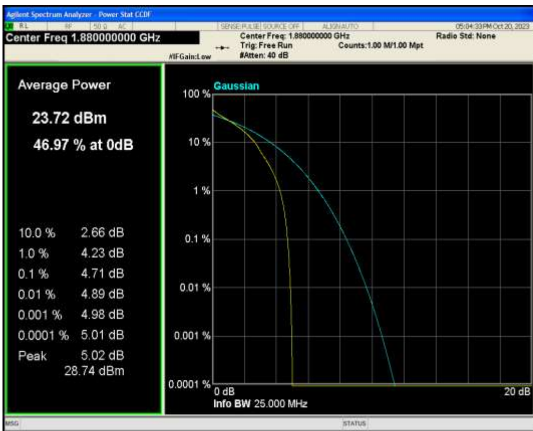
Band2 QAM16 BW=20MHz Channel=18900 RB Size=1 Position=#0
