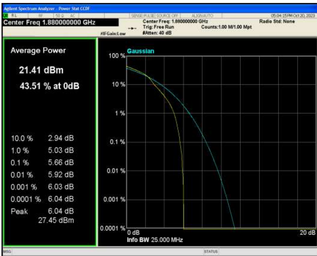
Band2 QPSK BW=10MHz Channel=18900 RB Size=1 Position=#0
