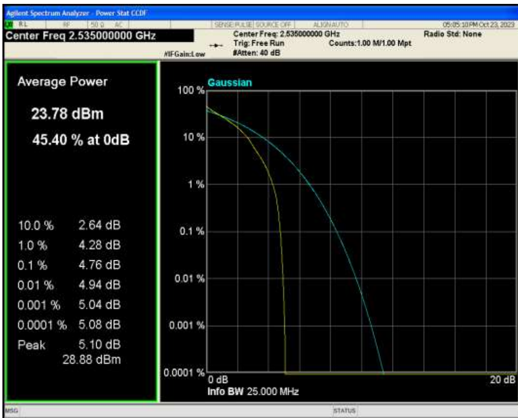
Band7 QAM16 BW=20MHz Channel=21100 RB Size=1 Position=#0
