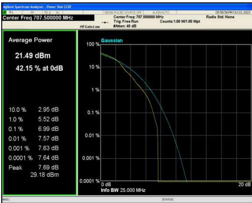
Band12 QPSK BW=5MHz Channel=23095 RB Size=1 Position=#0
