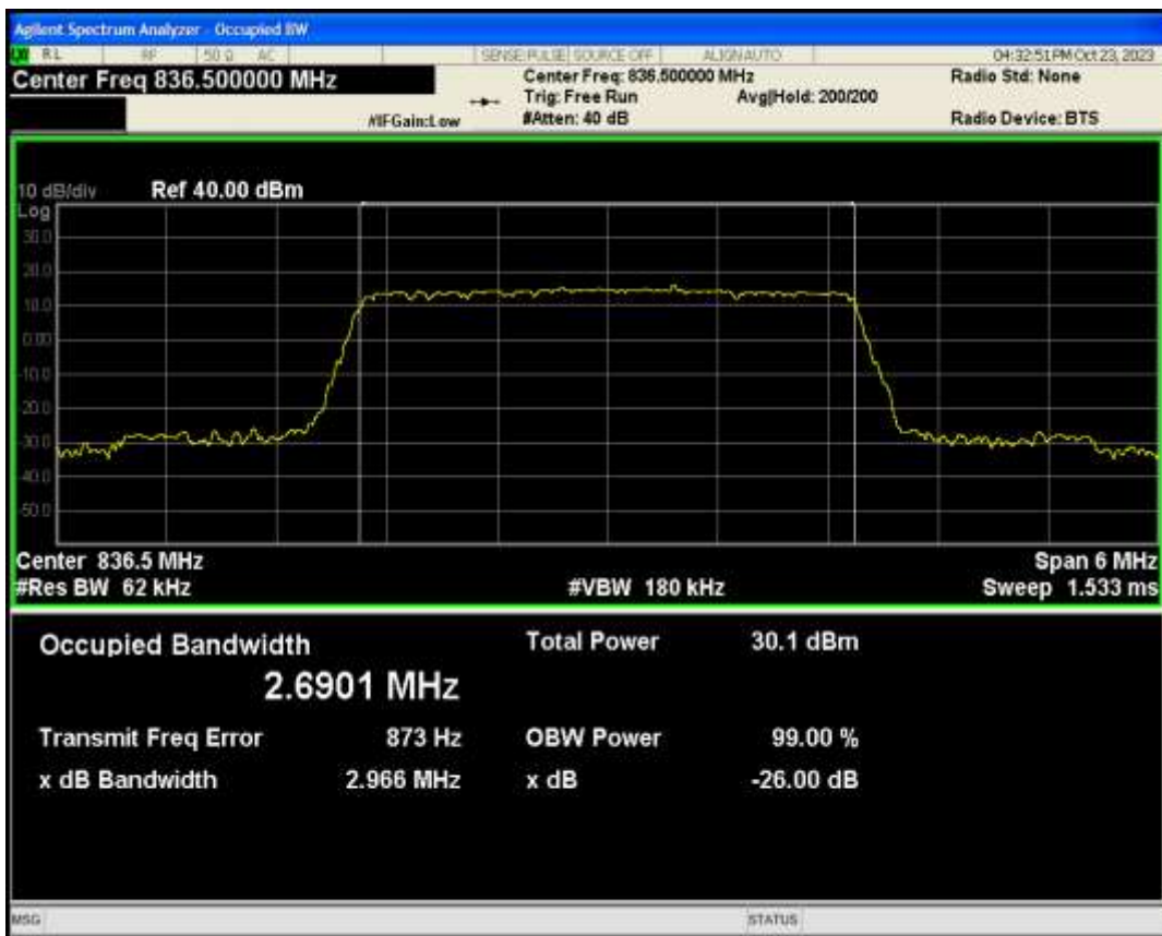
Band5 QAM16 BW=3MHz Channel=20525 RB Size=15 Position=#0
