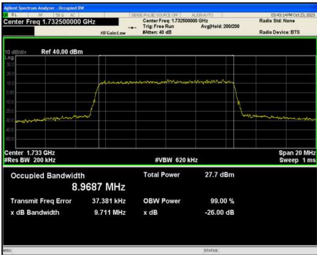
Band4 QAM16 BW=10MHz Channel=20175 RB Size=50 Position=#0
