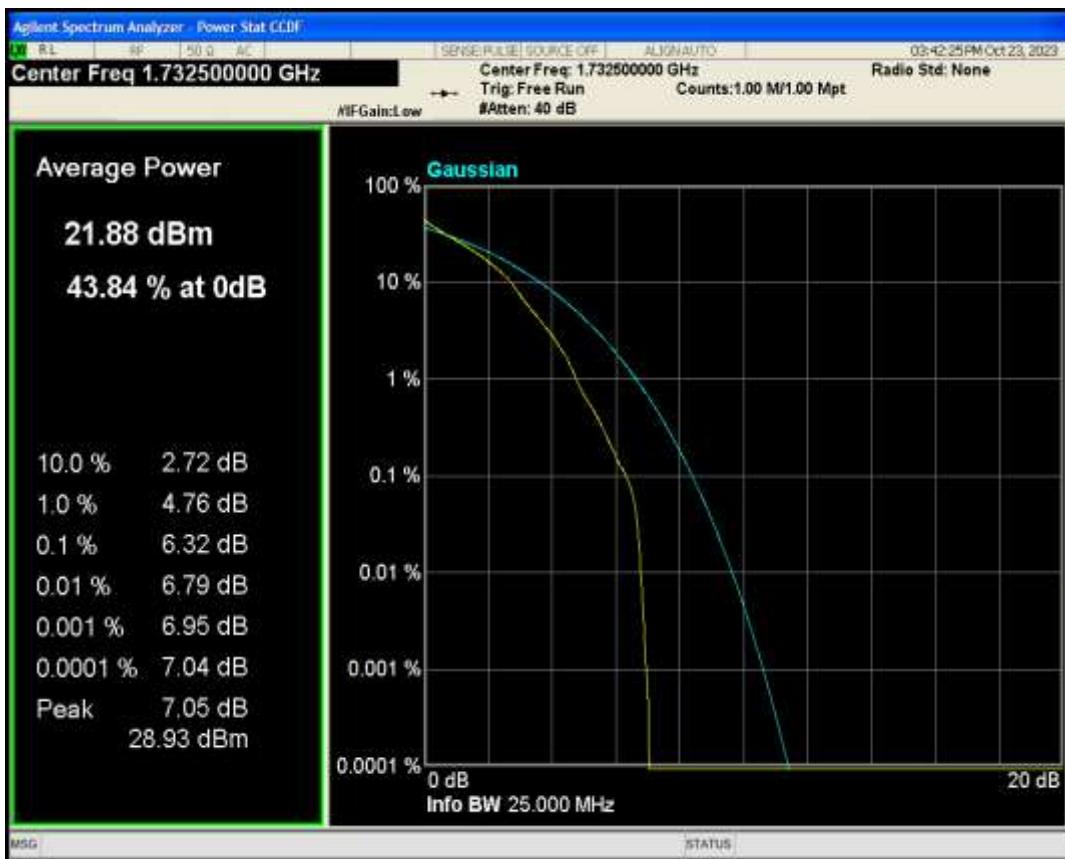
Band4 QAM16 BW=5MHz Channel=20175 RB Size=1 Position=#0
