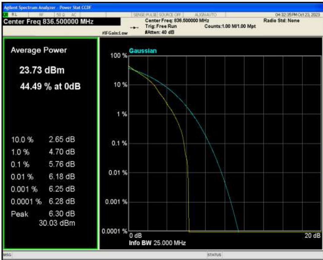
Band5 QAM16 BW=10MHz Channel=20525 RB Size=1 Position=#0
