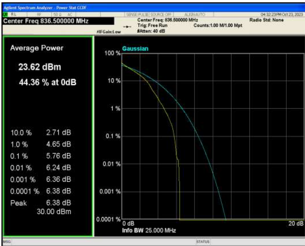
Band5 QAM16 BW=3MHz Channel=20525 RB Size=1 Position=#0
