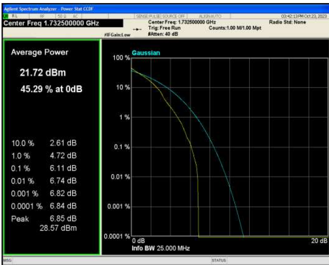
Band4 QAM16 BW=1.4MHz Channel=20175 RB Size=1 Position=#0
