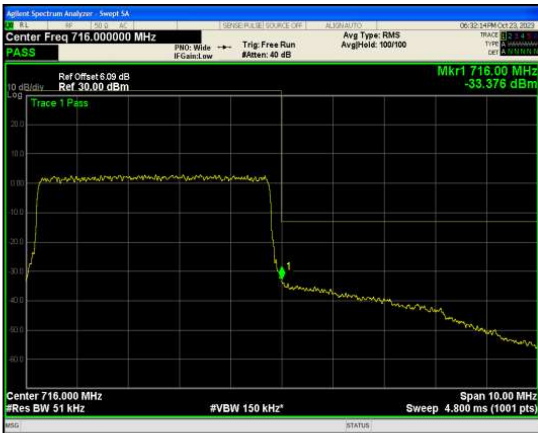
Band17 QPSK BW=10MHz Channel=23780 RB Size=50 Position=#0
