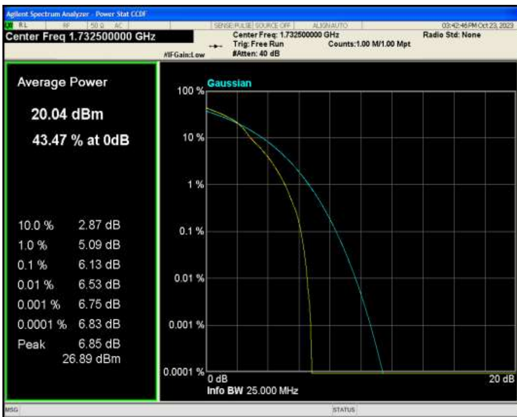
Band5 QPSK BW=1.4MHz Channel=20525 RB Size=1 Position=#0
