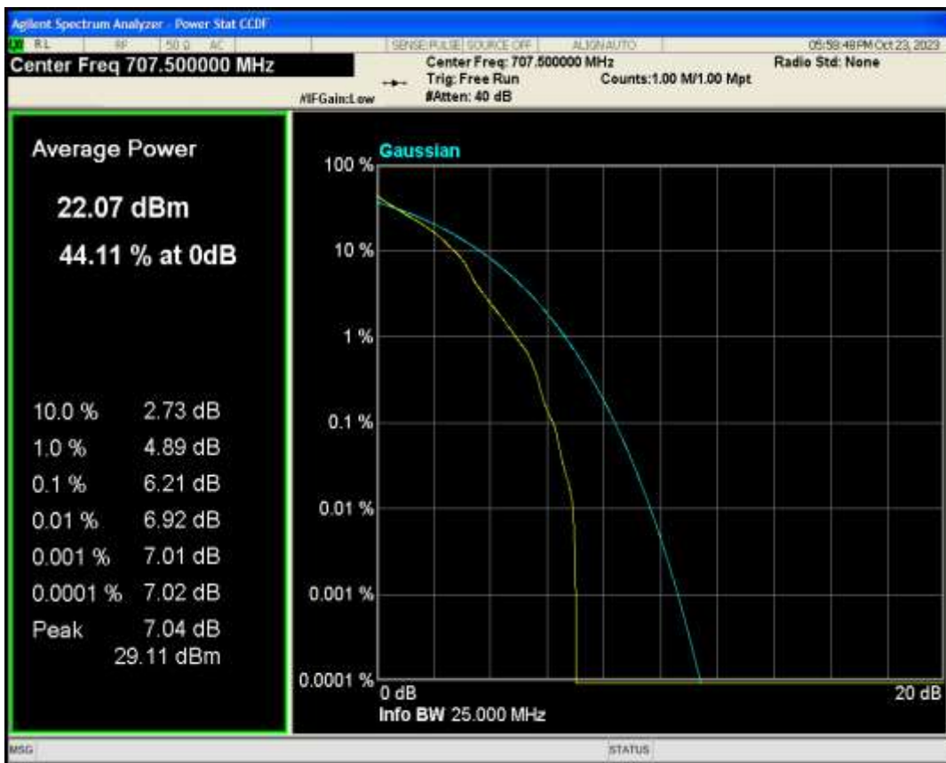
Band12 QAM16 BW=1.4MHz Channel=23095 RB Size=1 Position=#0
