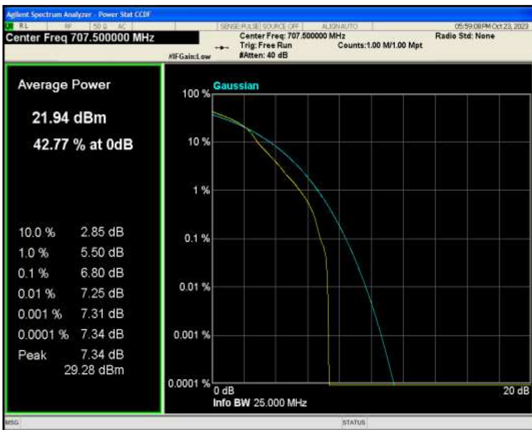
Band17 QPSK BW=5MHz Channel=23790 RB Size=1 Position=#0
