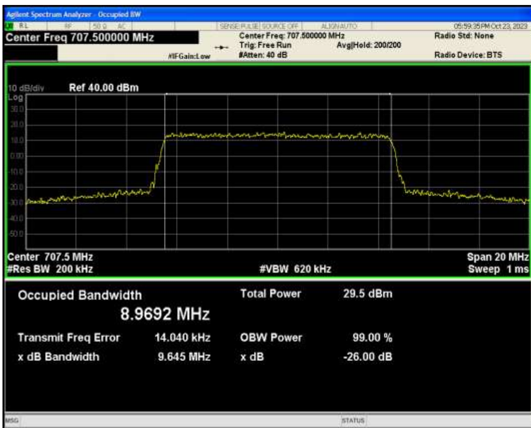
Band12 QAM16 BW=10MHz Channel=23095 RB Size=50 Position=#0
