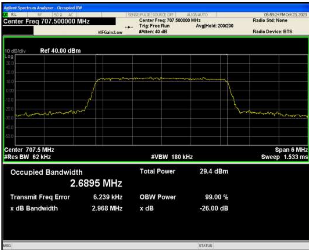
Band12 QPSK BW=5MHz Channel=23095 RB Size=25 Position=#0
