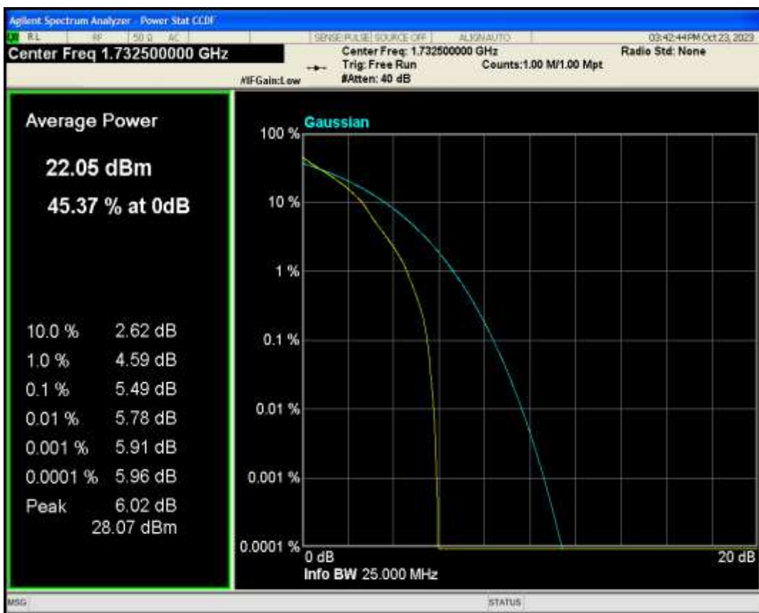
Band4 QAM16 BW=20MHz Channel=20175 RB Size=1 Position=#0
