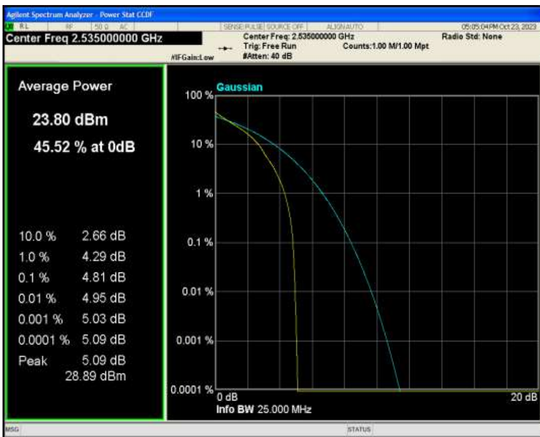
Band7 QAM16 BW=15MHz Channel=21100 RB Size=1 Position=#0
