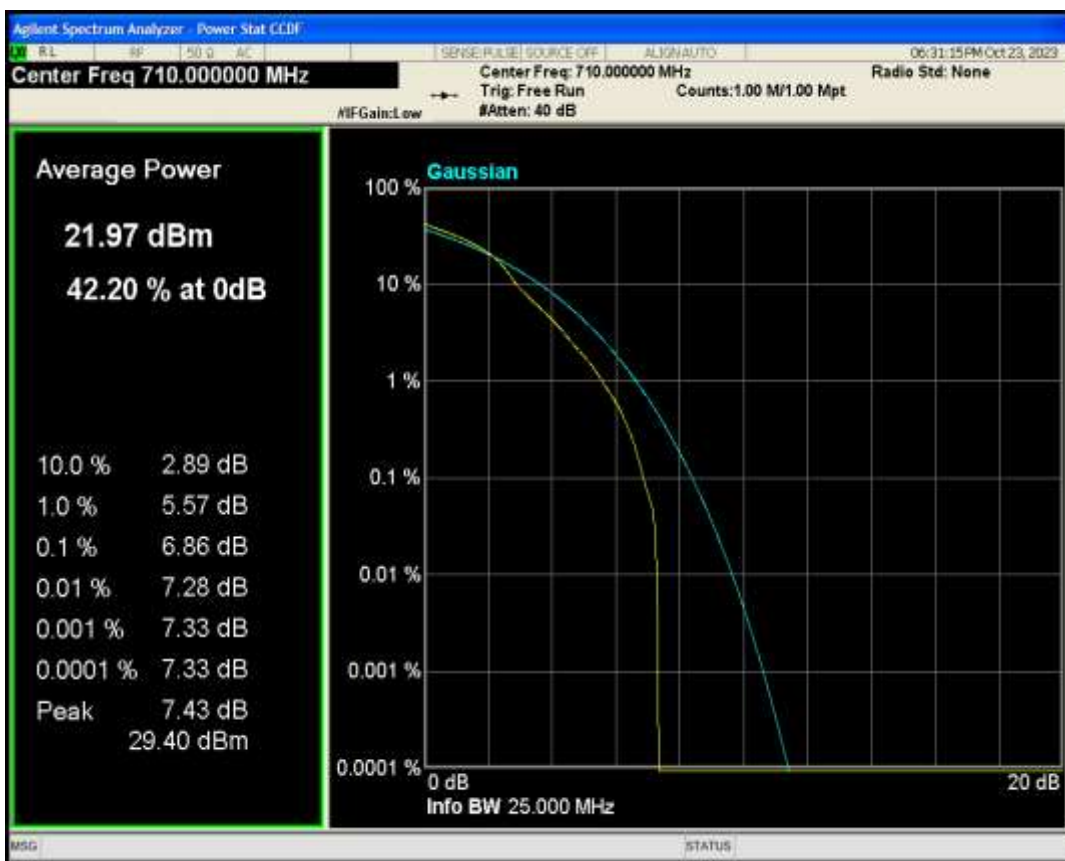
Band17 QPSK BW=10MHz Channel=23790 RB Size=1 Position=#0
