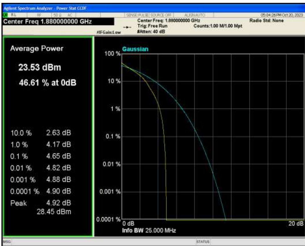
Band2 QAM16 BW=15MHz Channel=18900 RB Size=1 Position=#0
