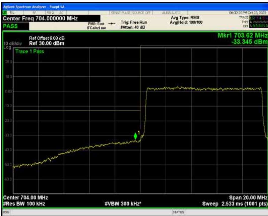
Band17 QPSK BW=10MHz Channel=23800 RB Size=50 Position=#0
