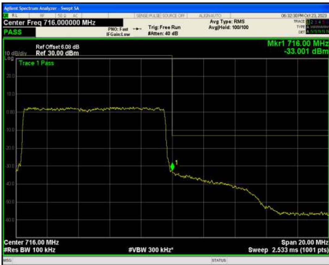
Band2 QPSK BW=1.4MHz Channel=18607 RB Size=6 Position=#0
