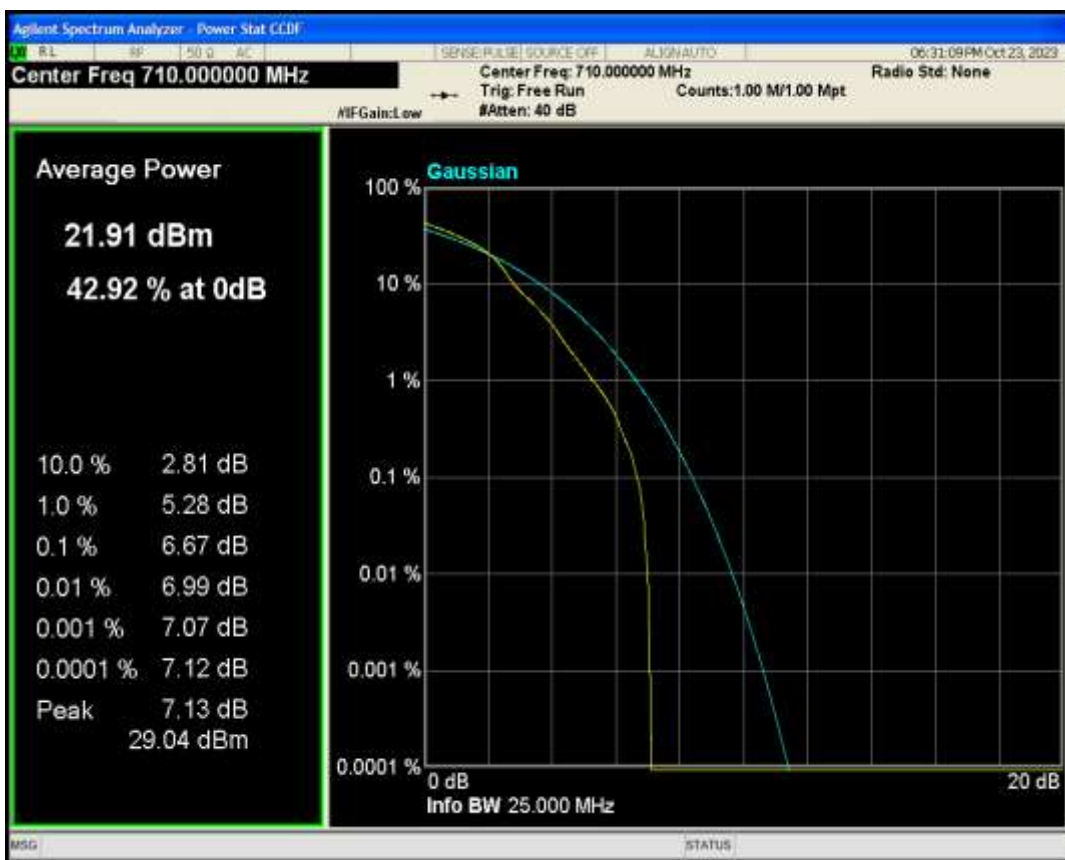
Band17 QAM16 BW=10MHz Channel=23790 RB Size=1 Position=#0
