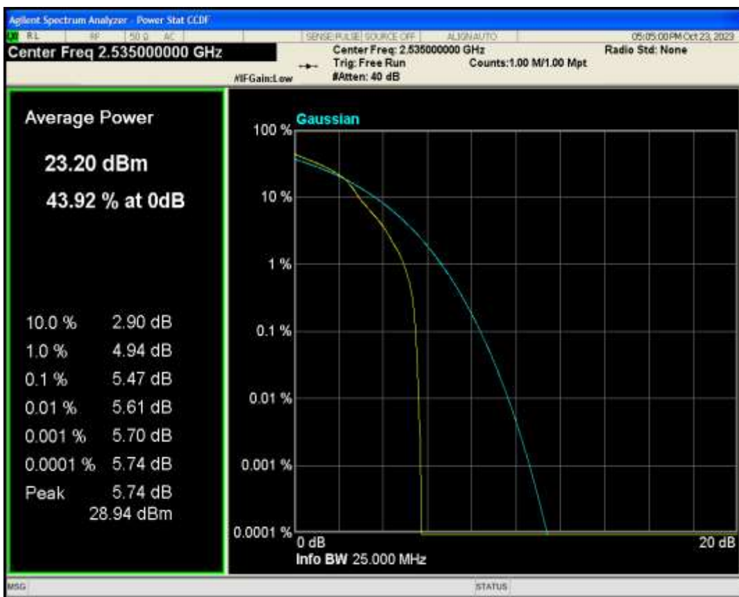
Band7 QPSK BW=15MHz Channel=21100 RB Size=1 Position=#0
