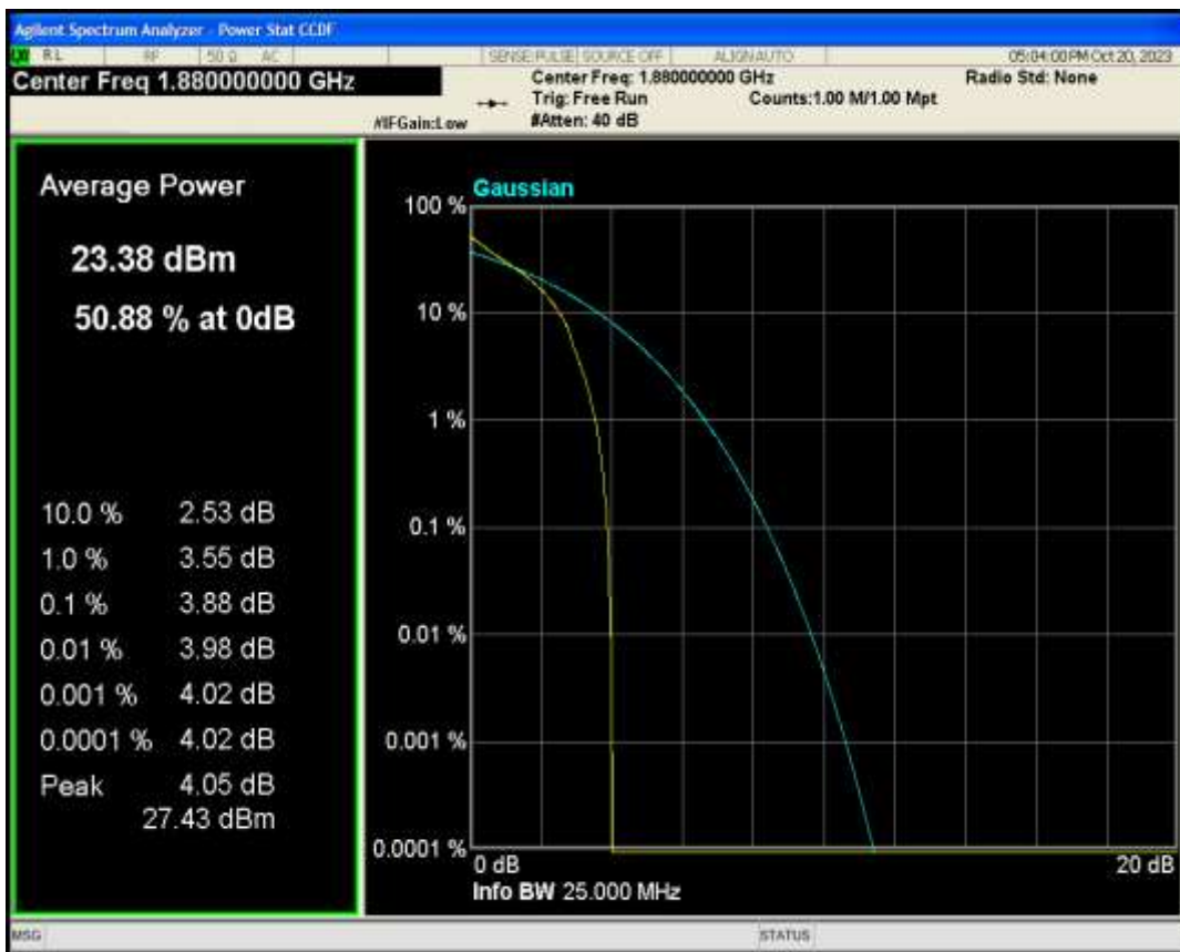
Band2 QAM16 BW=1.4MHz Channel=18900 RB Size=1 Position=#0
