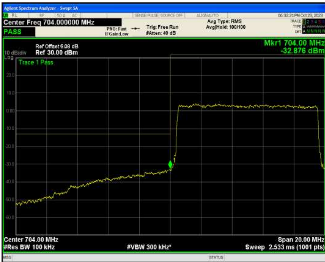
Band17 QAM16 BW=10MHz Channel=23780 RB Size=50 Position=#0
