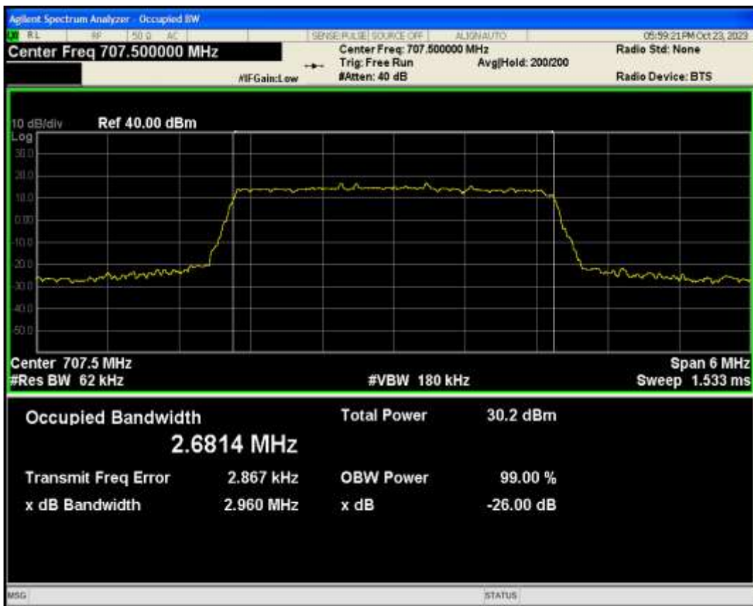
Band12 QAM16 BW=3MHz Channel=23095 RB Size=15 Position=#0
