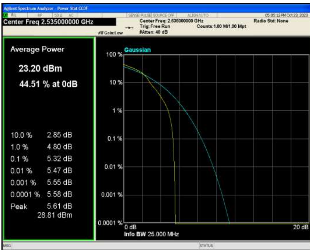
Band7 QAM16 BW=20MHz Channel=21100 RB Size=1 Position=#0
