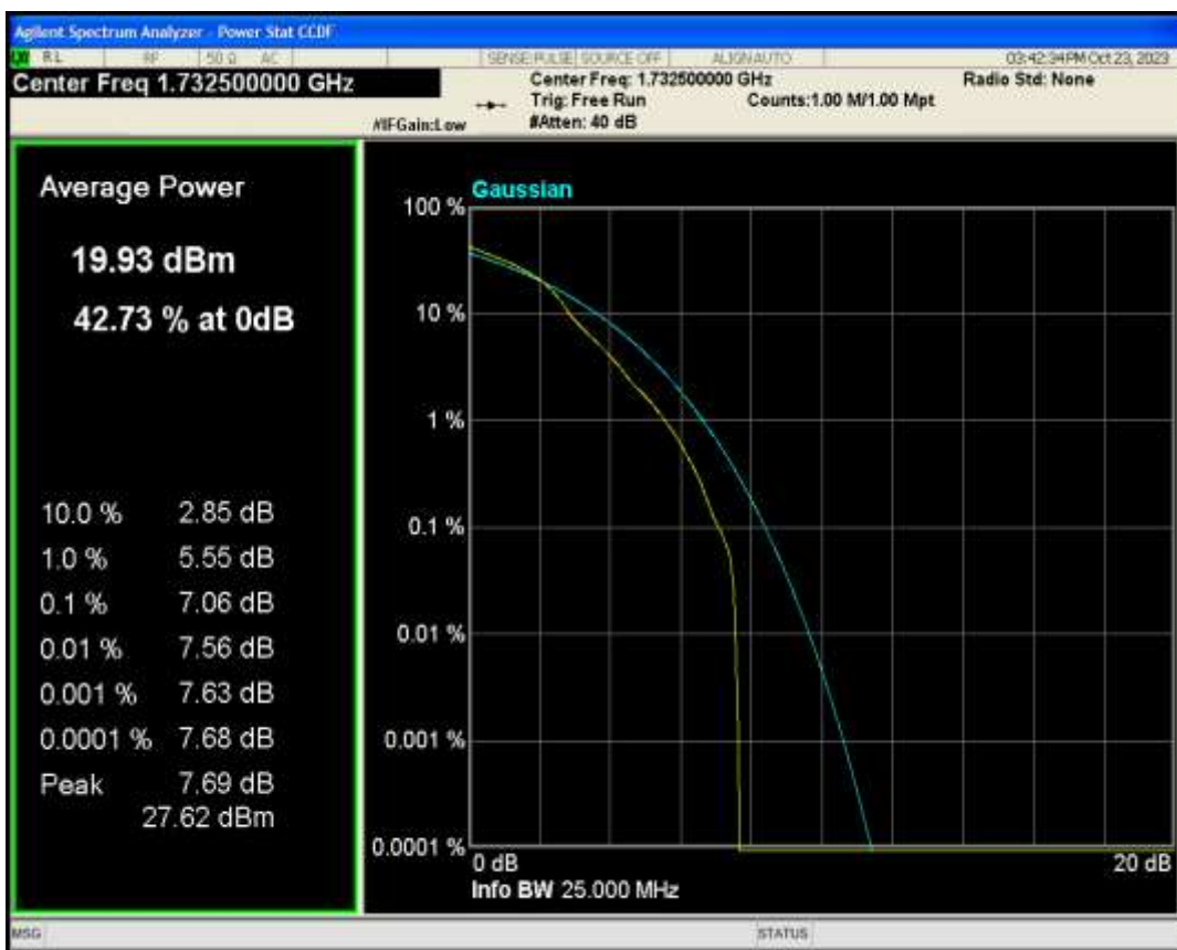
Band4 QPSK BW=15MHz Channel=20175 RB Size=1 Position=#0
