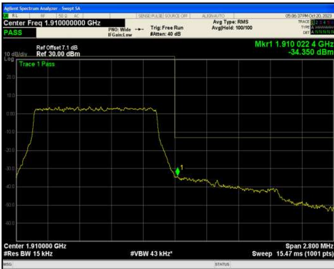
Band2 QAM16 BW=1.4MHz Channel=19193 RB Size=6 Position=#0
