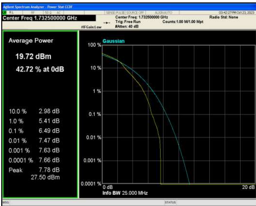
Band4 QPSK BW=10MHz Channel=20175 RB Size=1 Position=#0
