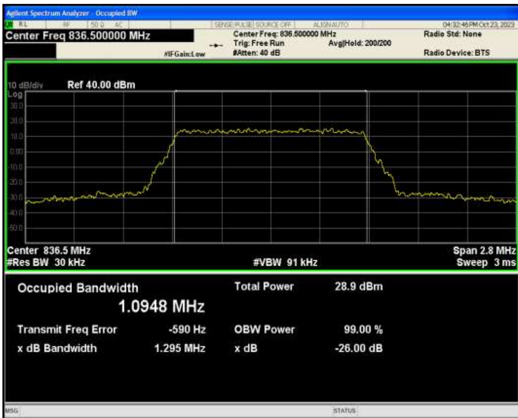
Band5 QPSK BW=3MHz Channel=20525 RB Size=15 Position=#0
