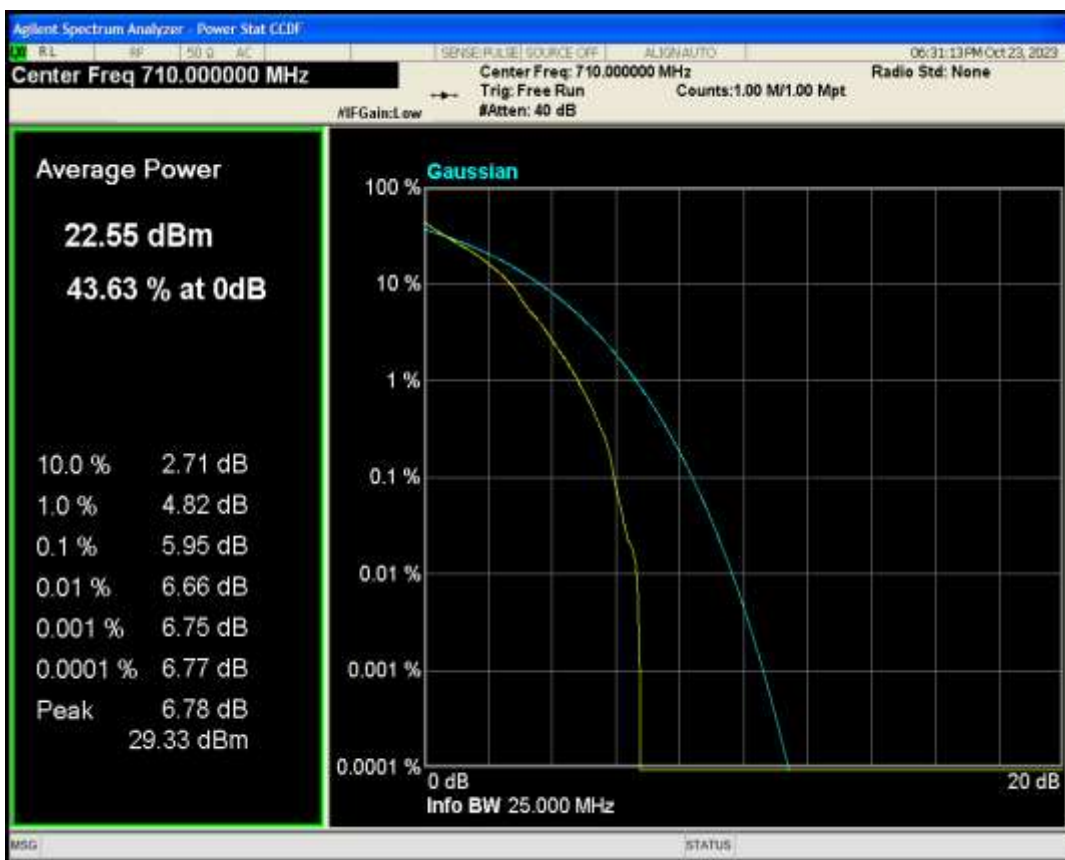
Band2 QPSK BW=1.4MHz Channel=18900 RB Size=1 Position=#0
