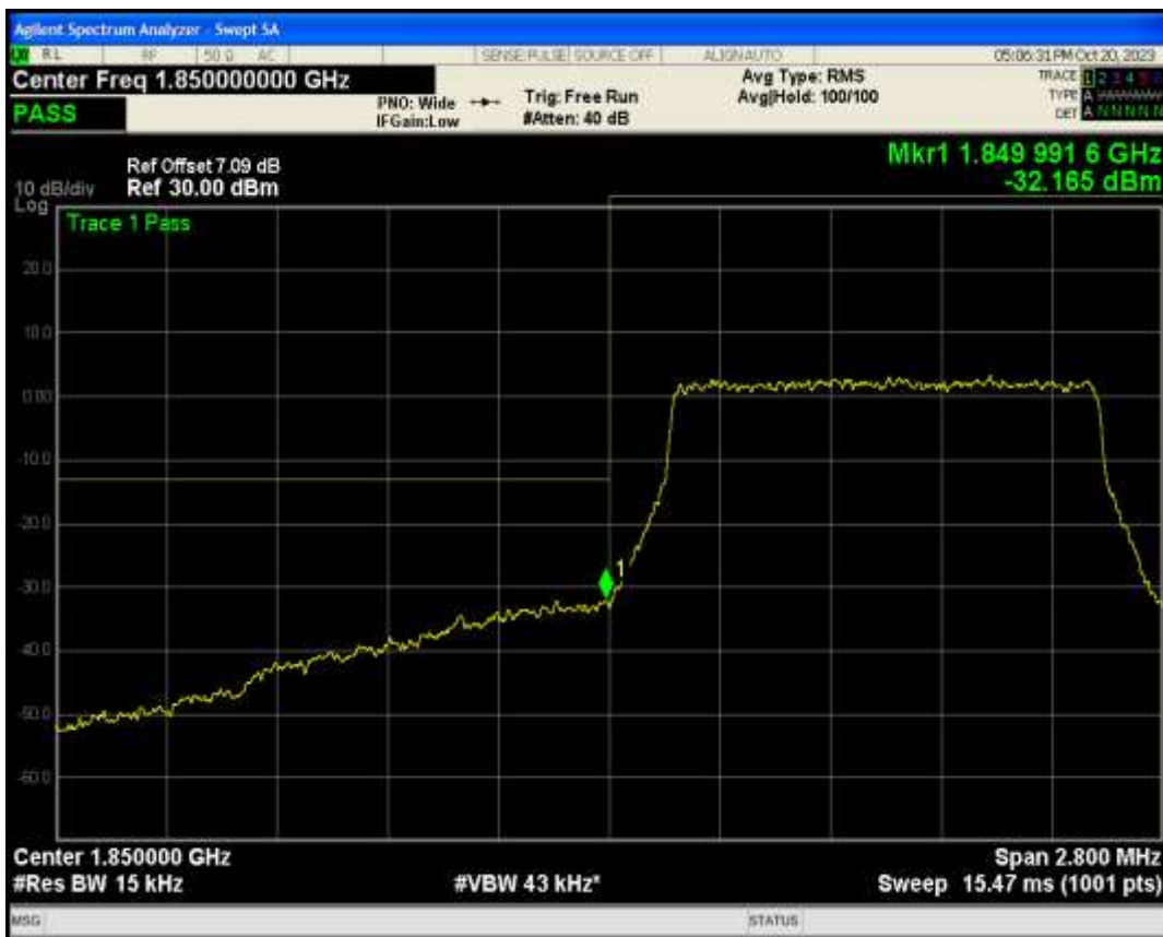
Band2 QPSK BW=1.4MHz Channel=19193 RB Size=6 Position=#0
