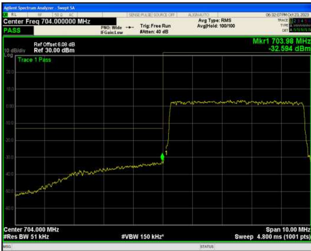
Band17 QPSK BW=5MHz Channel=23825 RB Size=25 Position=#0
