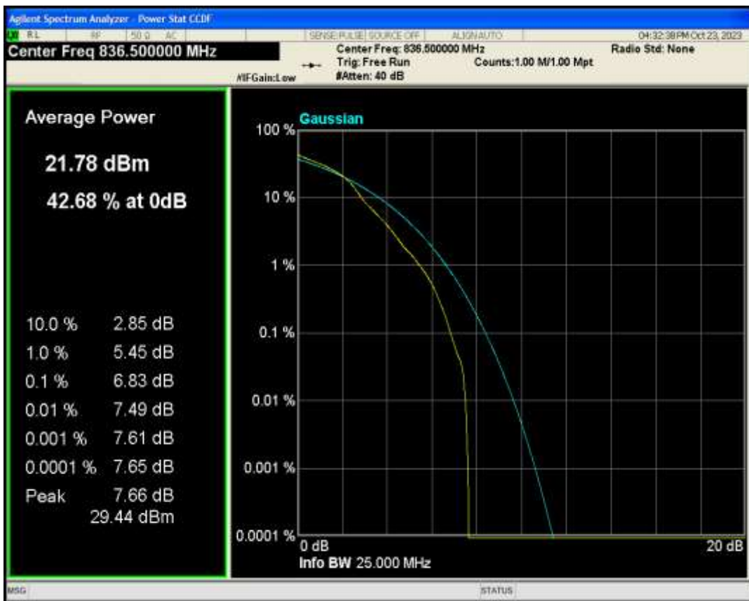
Band7 QPSK BW=5MHz Channel=21100 RB Size=1 Position=#0
