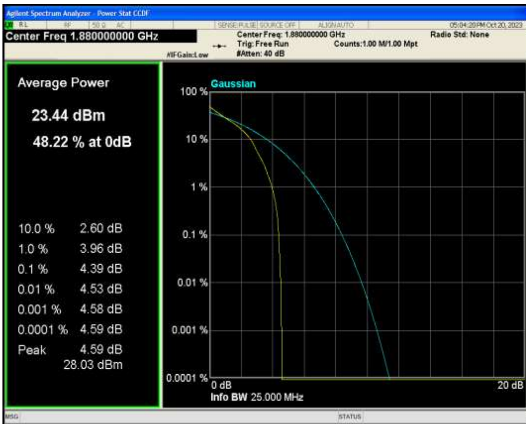
Band2 QAM16 BW=10MHz Channel=18900 RB Size=1 Position=#0
