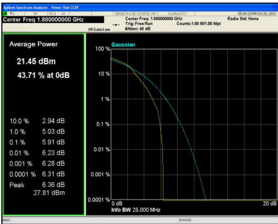
Band2 QPSK BW=15MHz Channel=18900 RB Size=1 Position=#0
