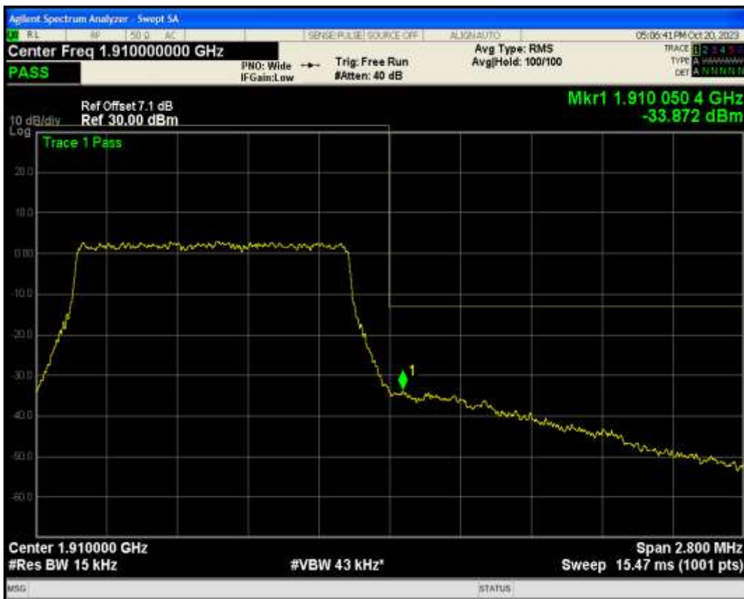
Band2 QPSK BW=3MHz Channel=18615 RB Size=15 Position=#0
