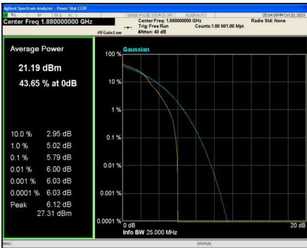
Band2 QPSK BW=5MHz Channel=18900 RB Size=1 Position=#0
