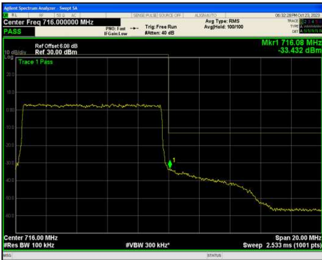
Band17 QAM16 BW=10MHz Channel=23800 RB Size=50 Position=#0
