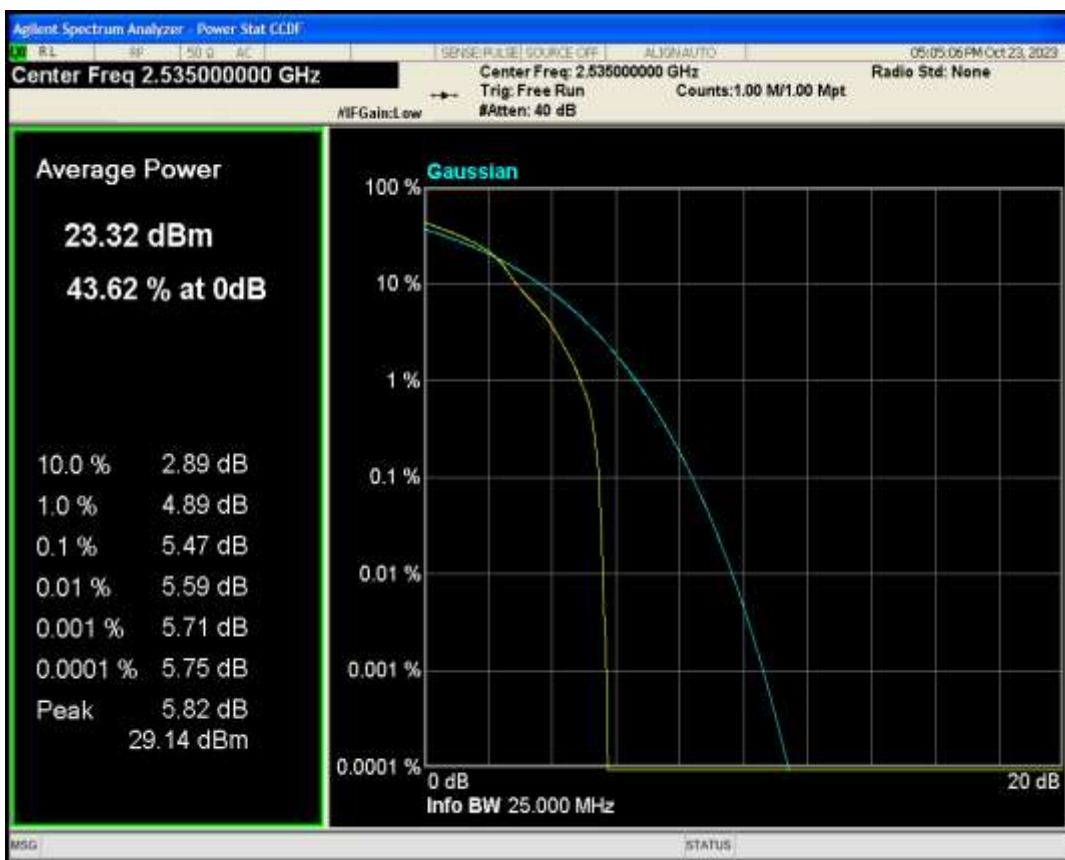
Band7 QPSK BW=20MHz Channel=21100 RB Size=1 Position=#0
