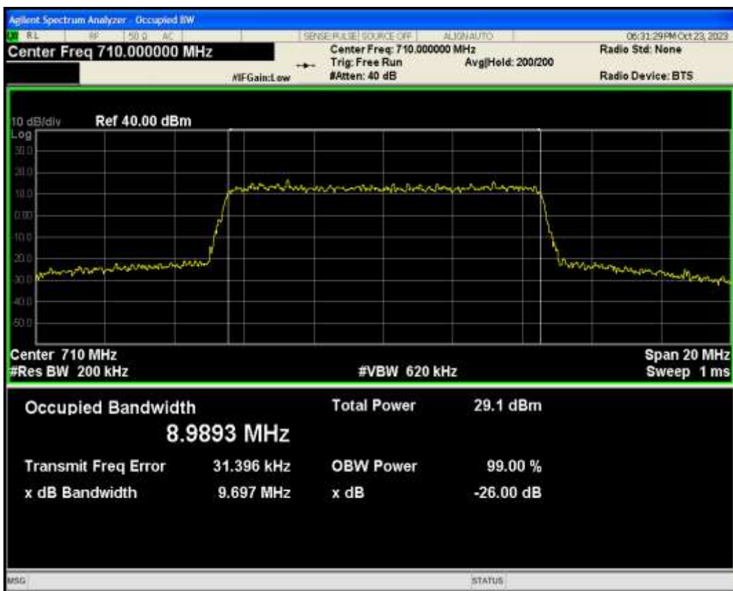
Band17 QPSK BW=10MHz Channel=23790 RB Size=50 Position=#0
