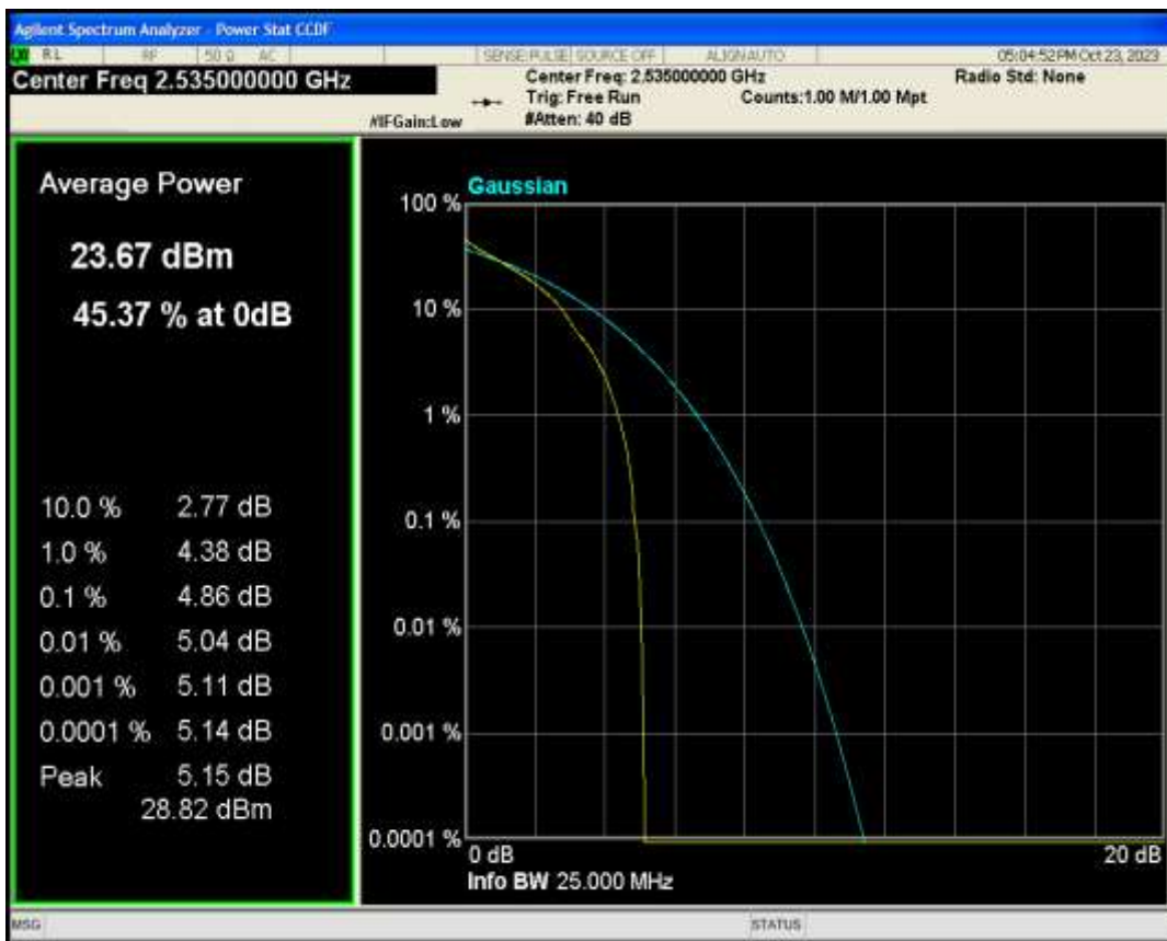
Band7 QAM16 BW=5MHz Channel=21100 RB Size=1 Position=#0
