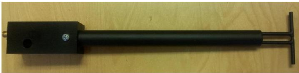
Figure 1 – MVG COMOSAR Validation Dipole
