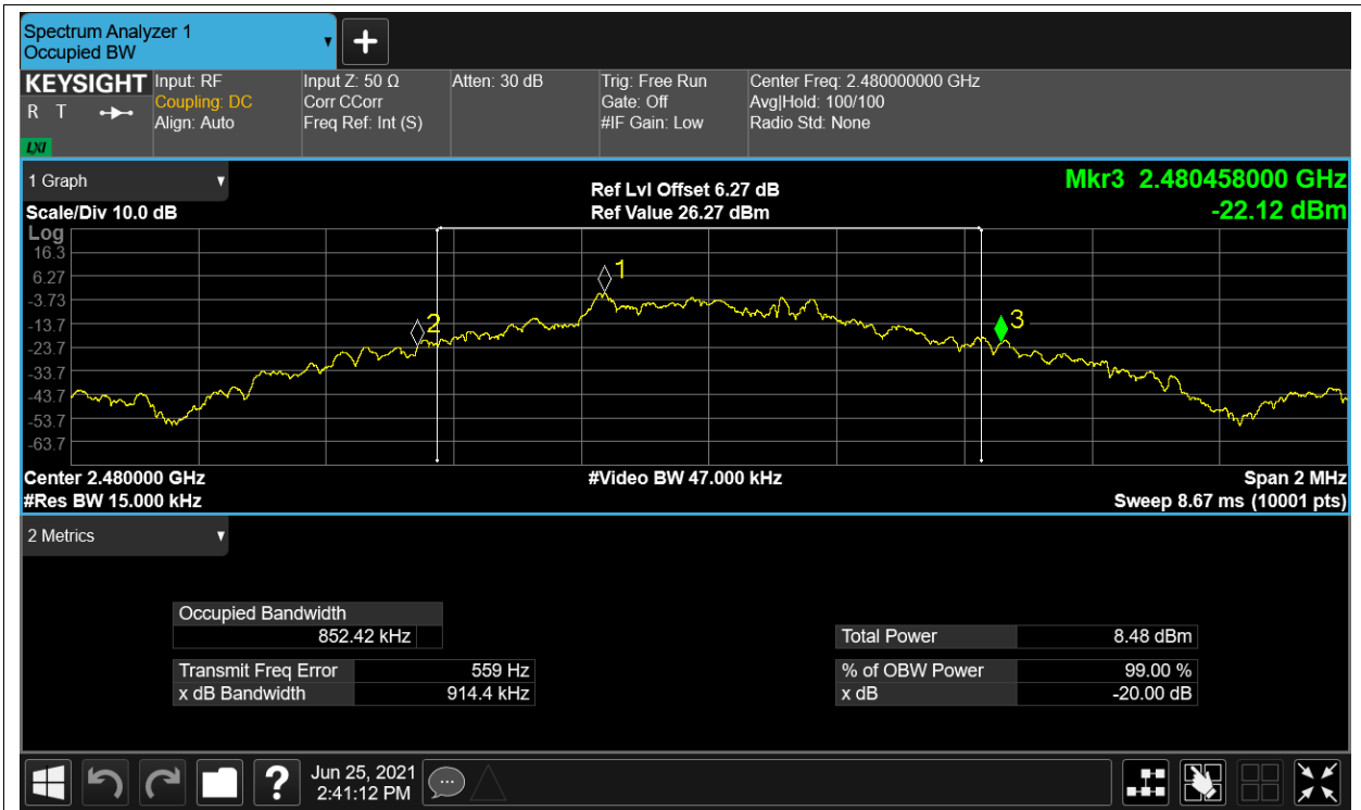
-20dB Bandwidth NVNT 2-DH1 2402MHz Ant1
