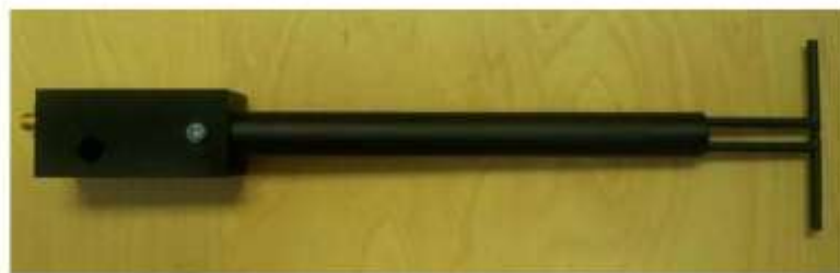
Figure 1 – MVG COMOSAR Validation Dipole
