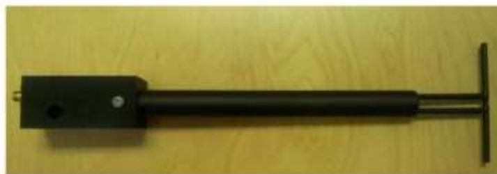
Figure 1 – MVG COMOSAR Validation Dipole
