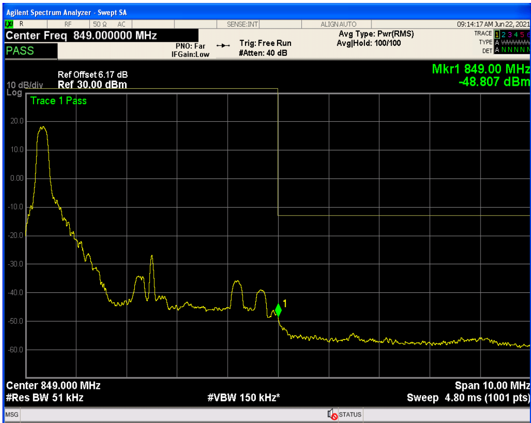
Band5 QPSK BW=5MHz Channel=20625 RB Size=1 Position=#Max
