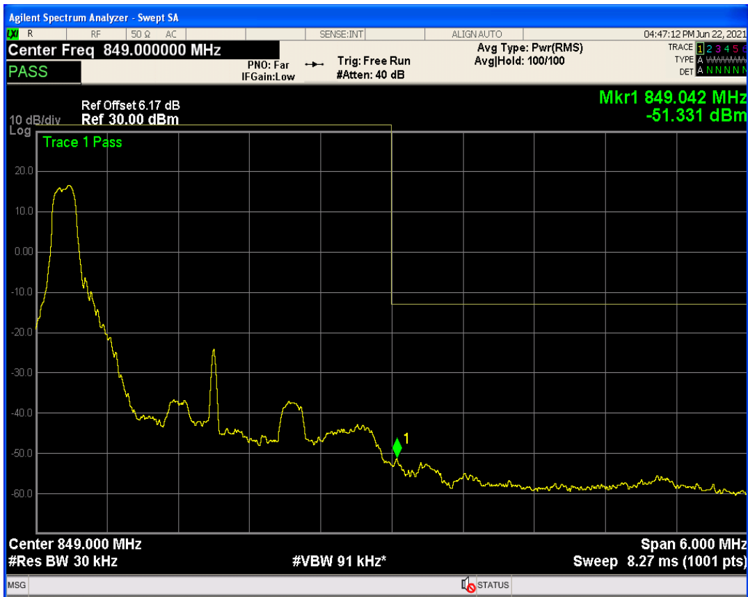
Band26b QPSK BW=3MHz Channel=27025 RB Size=15 Position=#0
