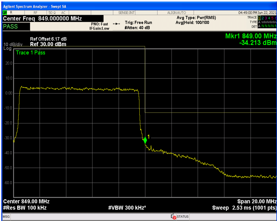
Band26b QAM16 BW=10MHz Channel=26990 RB Size=1 Position=#0
