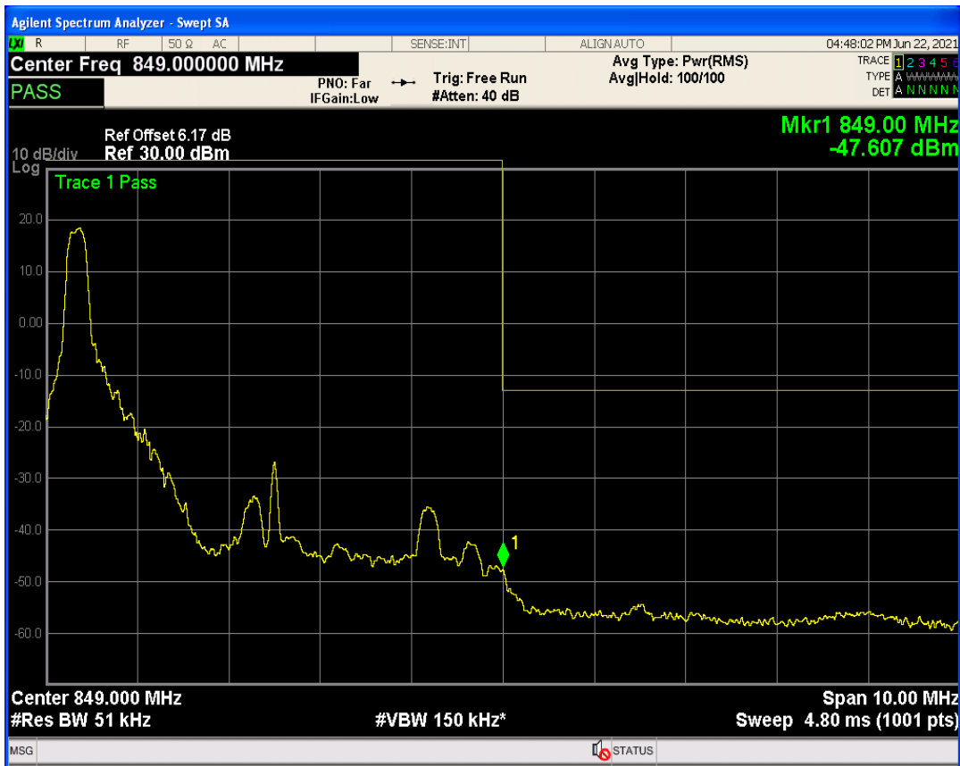
Band26b QPSK BW=5MHz Channel=27015 RB Size=1 Position=#Max
