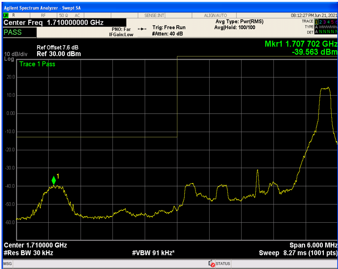
Band4 QPSK BW=3MHz Channel=20385 RB Size=1 Position=#0
