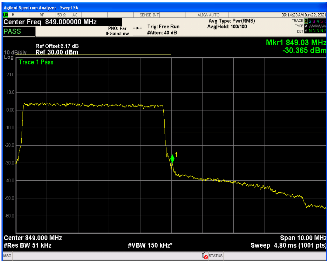
Band5 QAM16 BW=5MHz Channel=20625 RB Size=1 Position=#0
