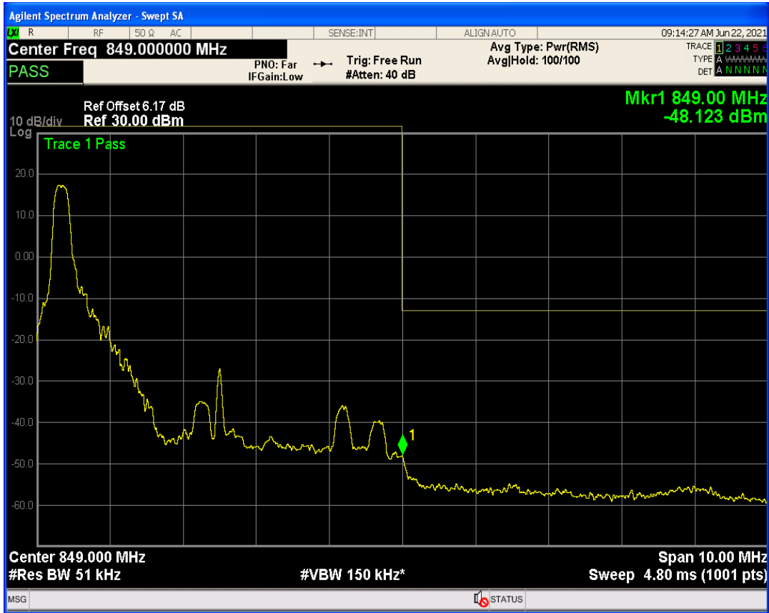
Band5 QAM16 BW=5MHz Channel=20625 RB Size=25 Position=#0
