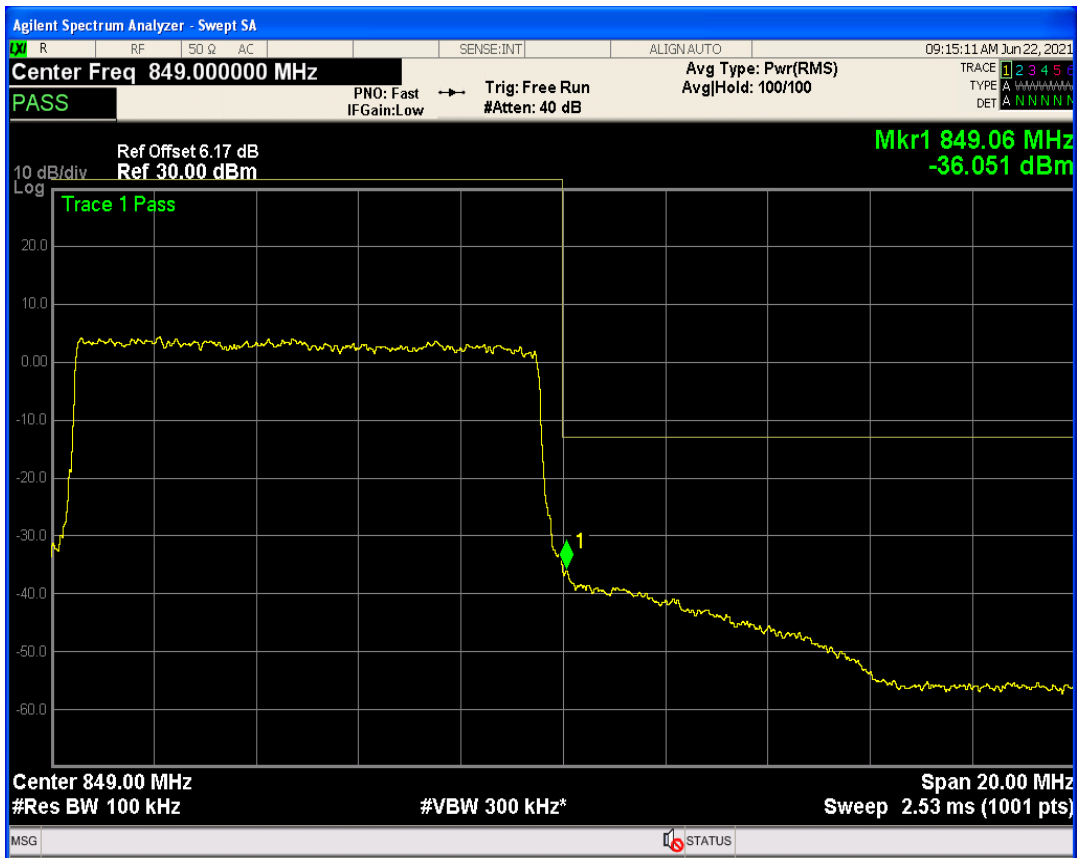
Band5 QAM16 BW=10MHz Channel=20600 RB Size=1 Position=#0
