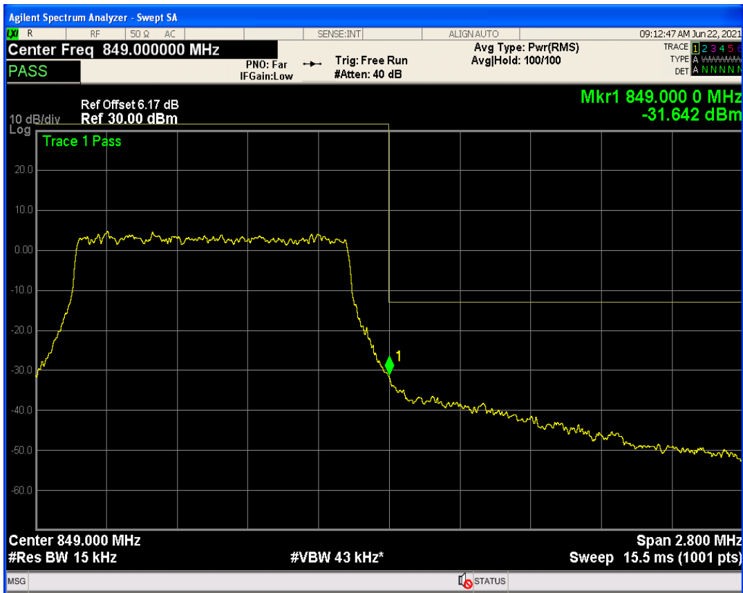
Band5 QPSK BW=3MHz Channel=20415 RB Size=1 Position=#Max
