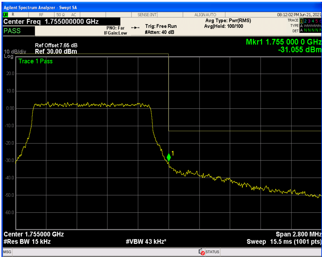
Band4 QPSK BW=3MHz Channel=19965 RB Size=1 Position=#Max
