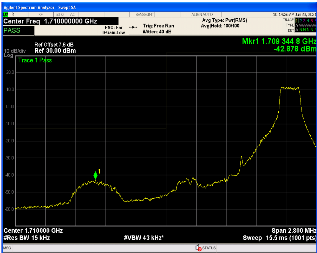
Band66 QPSK BW=1.4MHz Channel=132665 RB Size=1 Position=#0
