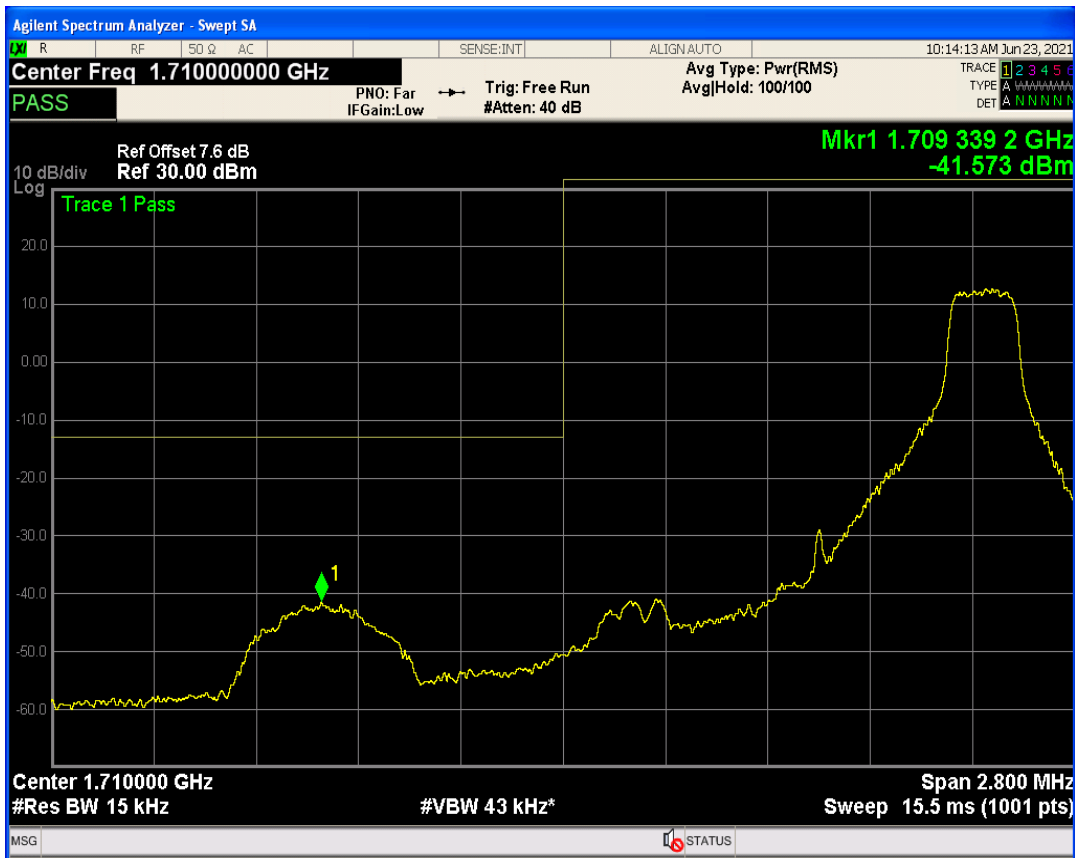
Band66 QPSK BW=1.4MHz Channel=131979 RB Size=1 Position=#0
