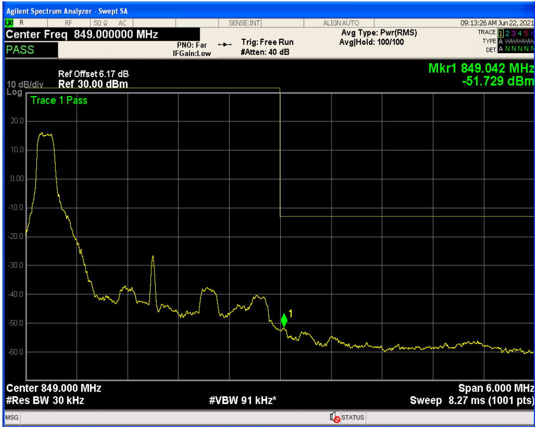
Band5 QAM16 BW=3MHz Channel=20415 RB Size=15 Position=#0
