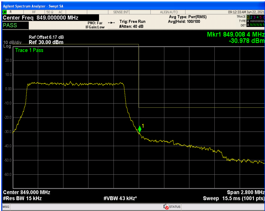
Band5 QAM16 BW=1.4MHz Channel=20643 RB Size=1 Position=#0
