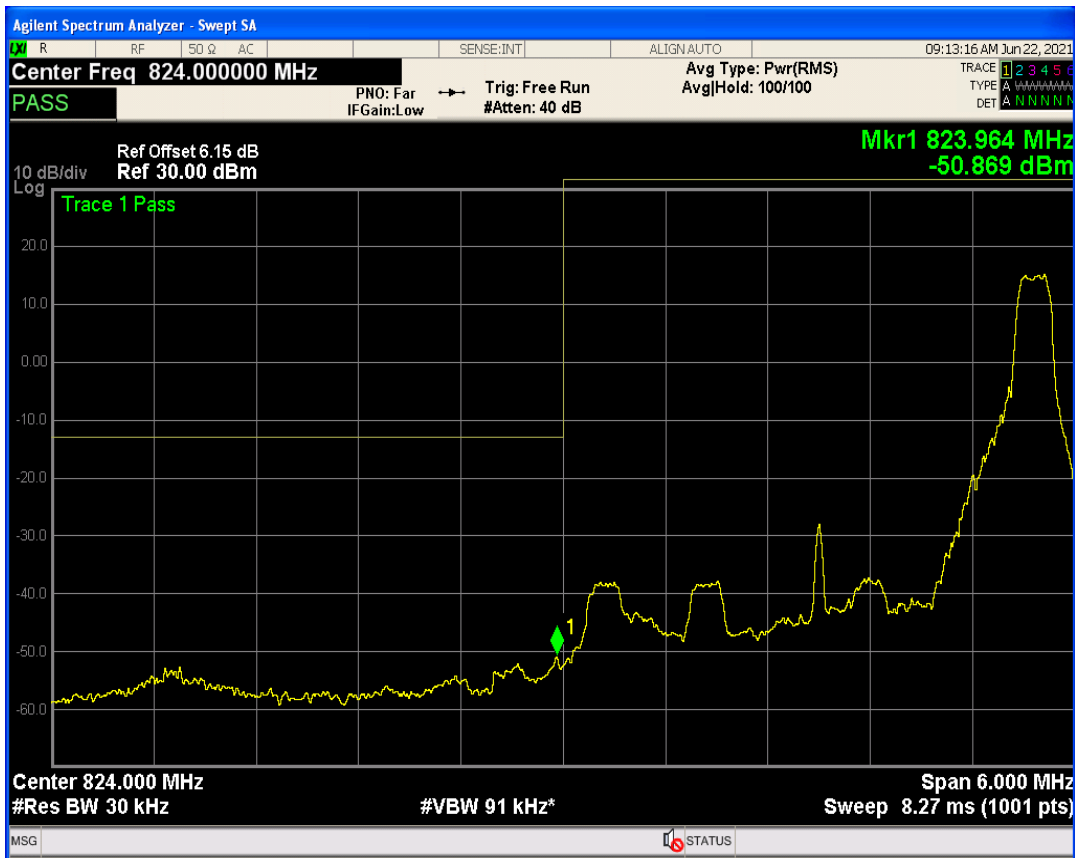
Band5 QPSK BW=3MHz Channel=20635 RB Size=1 Position=#0
