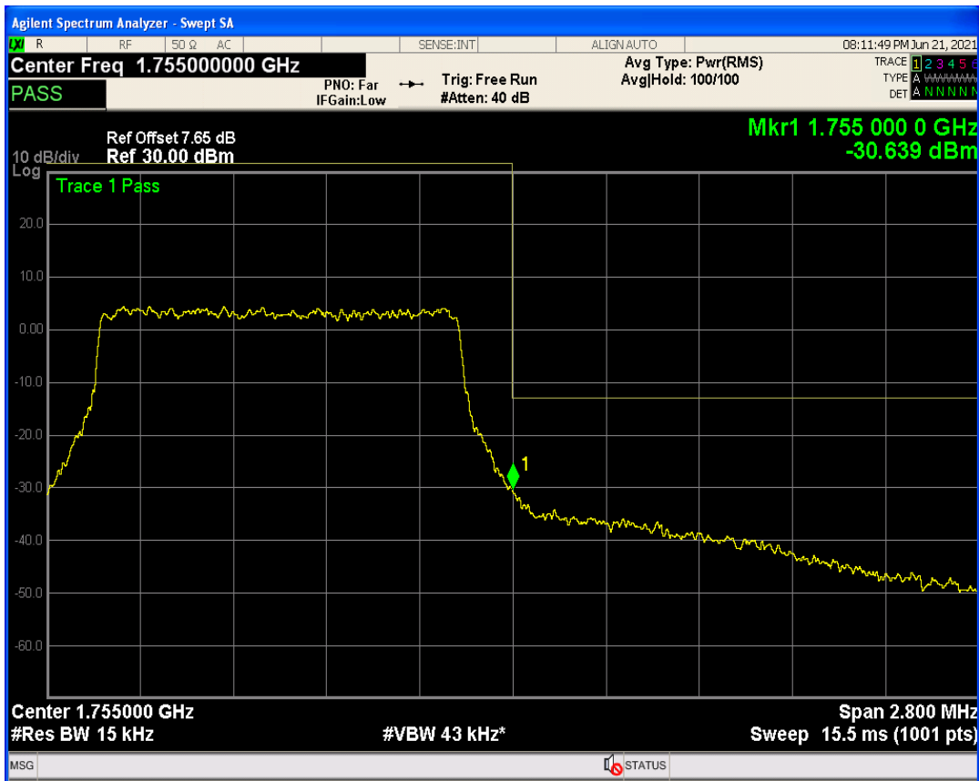
Band4 QAM16 BW=1.4MHz Channel=20393 RB Size=1 Position=#0
