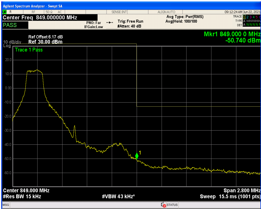
Band5 QPSK BW=1.4MHz Channel=20643 RB Size=1 Position=#Max
