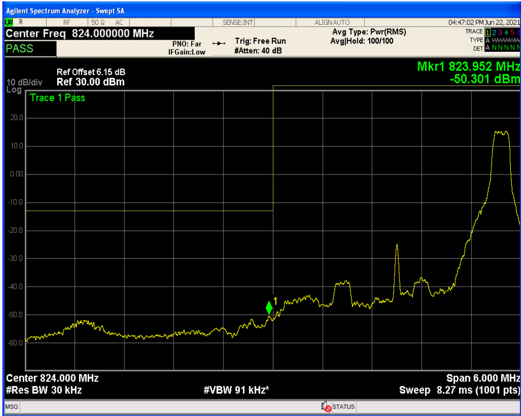
Band26b QPSK BW=3MHz Channel=27025 RB Size=1 Position=#0
