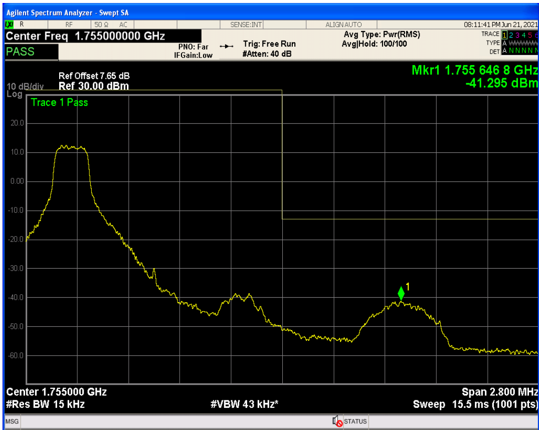
Band4 QPSK BW=1.4MHz Channel=20393 RB Size=1 Position=#Max
