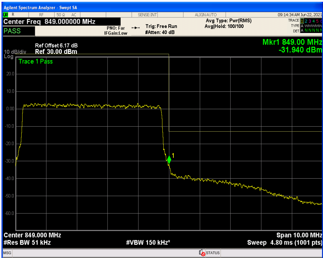
Band5 QAM16 BW=5MHz Channel=20625 RB Size=1 Position=#Max
