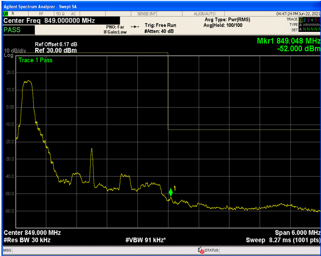
Band26b QAM16 BW=3MHz Channel=27025 RB Size=15 Position=#0
