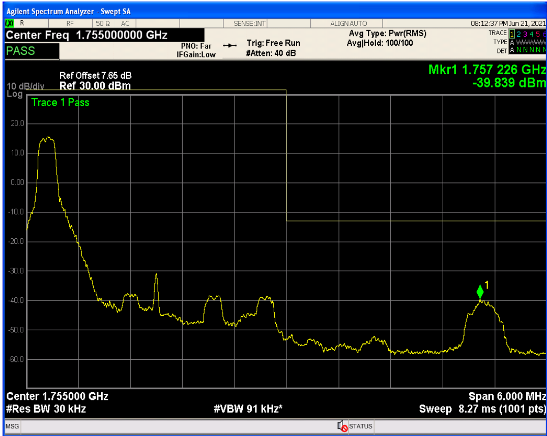
Band4 QAM16 BW=3MHz Channel=19965 RB Size=15 Position=#0
