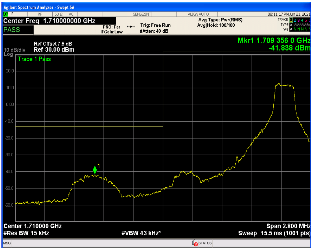
Band4 QPSK BW=1.4MHz Channel=19957 RB Size=1 Position=#0
