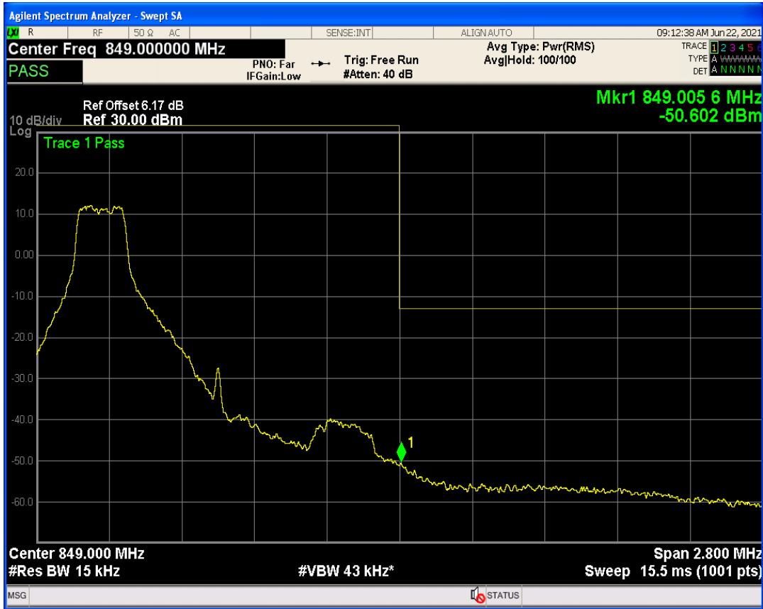
Band5 QAM16 BW=1.4MHz Channel=20643 RB Size=1 Position=#Max
