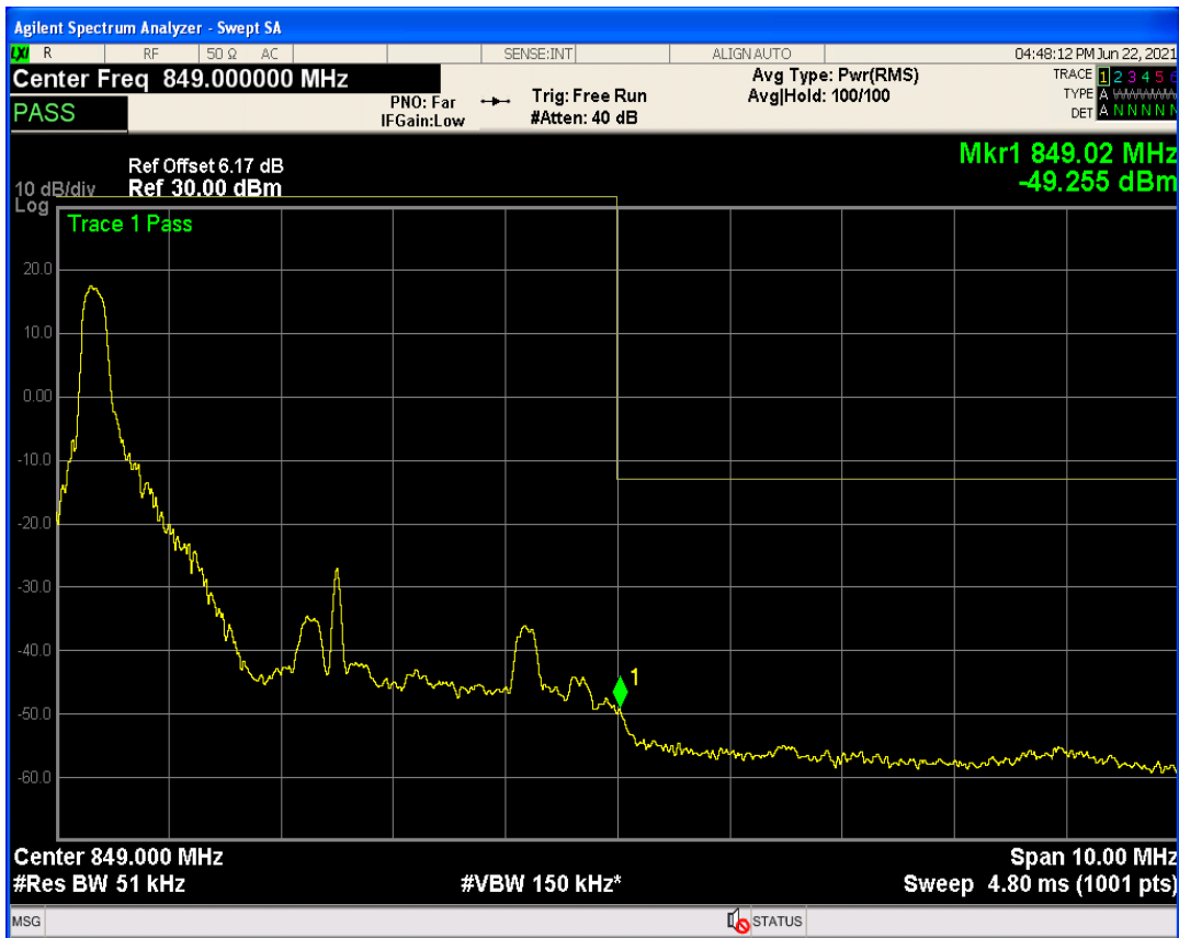
Band26b QPSK BW=5MHz Channel=27015 RB Size=25 Position=#0
