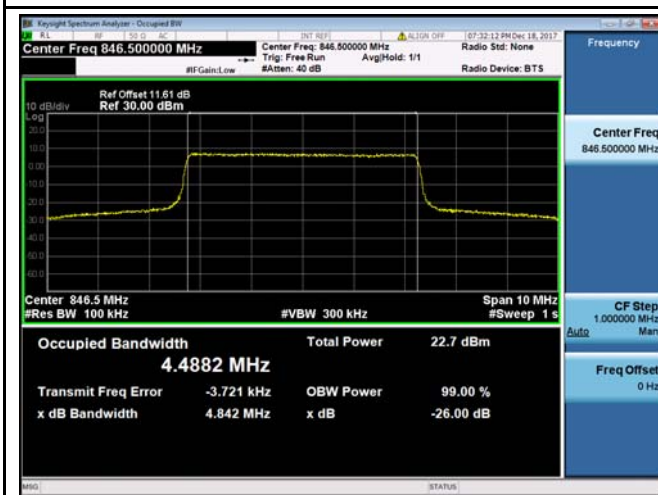
LTE band 5 - Middle CH QPSK-5
