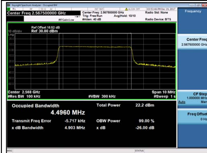
LTE band 7 - High CH QPSK-5
