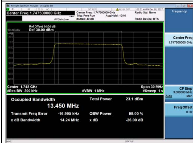
LTE band 4 - Middle CH QPSK-15
