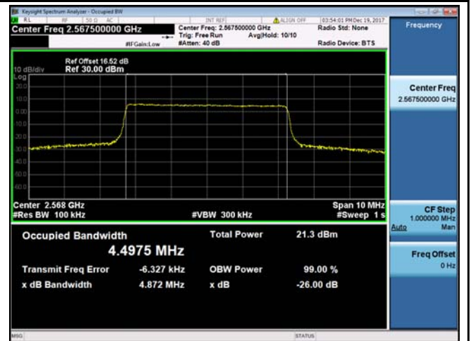
LTE band 7 - High CH 16QAM-5
