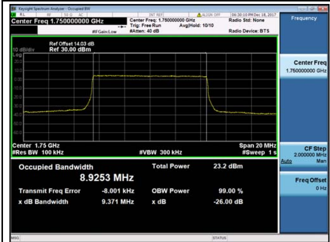
LTE band 4 - High CH QPSK-10
