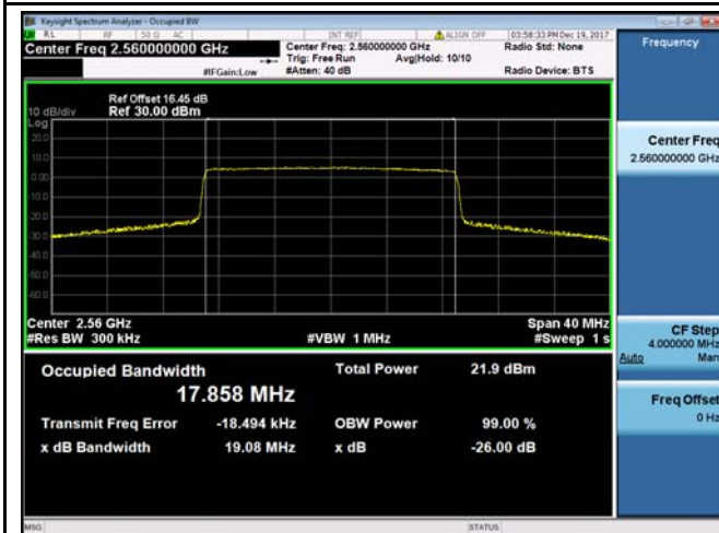
LTE band 7 - Middle CH QPSK-20
