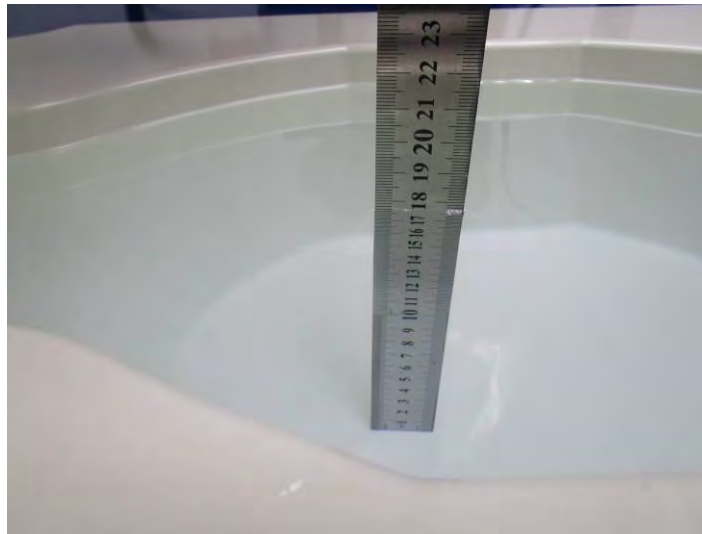
Liquid Height for Body SAR
