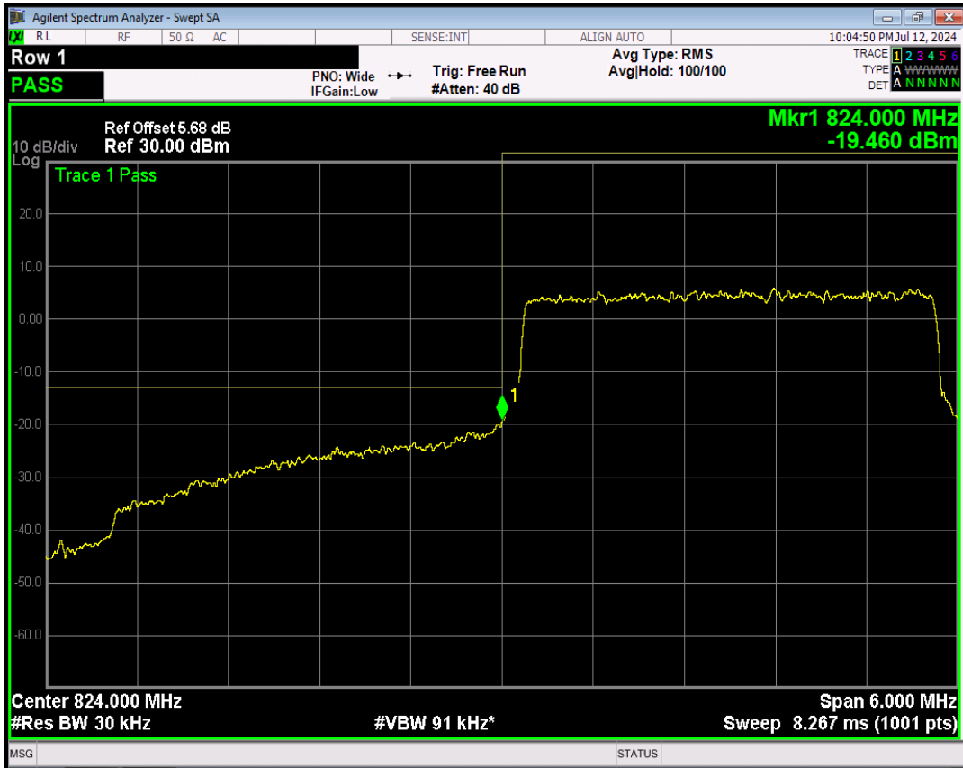
Band5 16QAM BW=3MHz Channel=20415 RB Size=15 Position=#0
