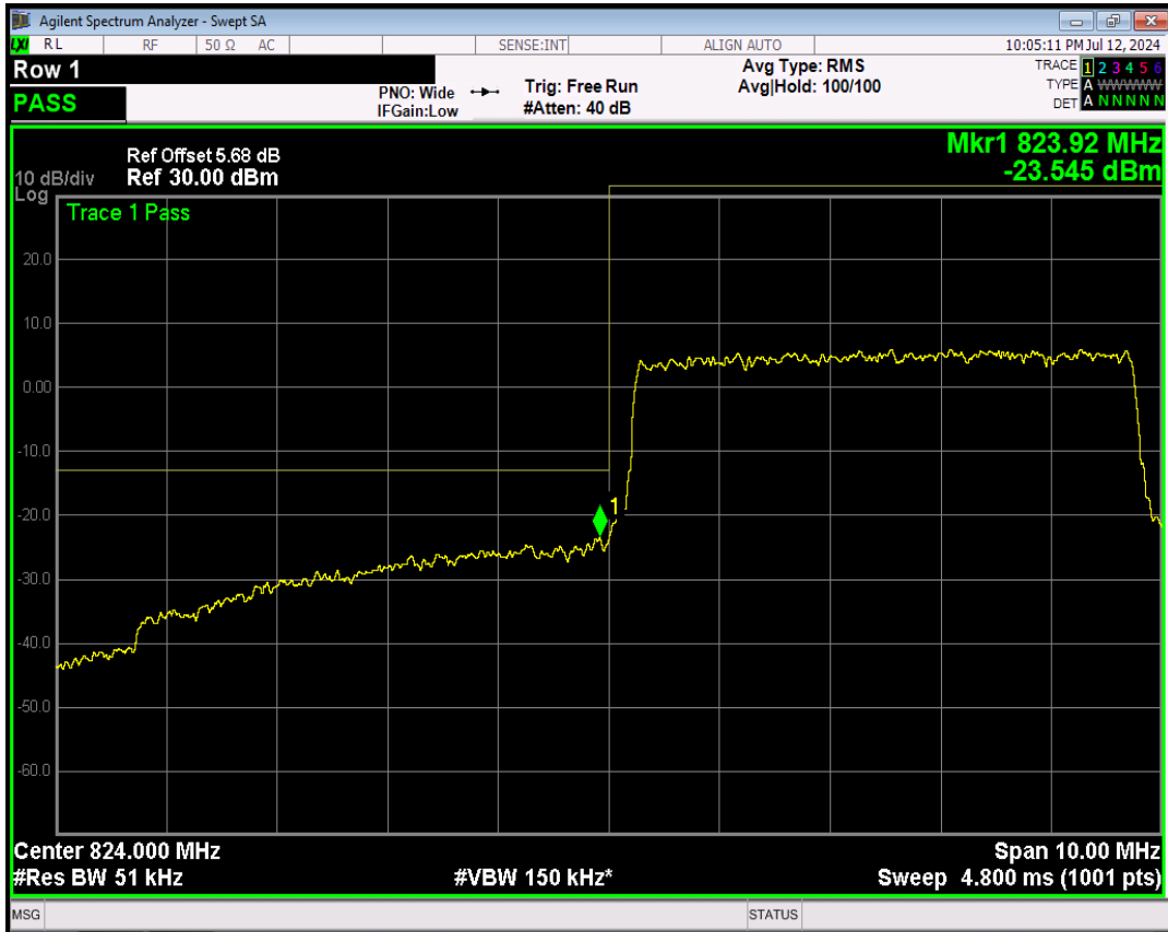
Band5 16QAM BW=5MHz Channel=20425 RB Size=25 Position=#0
