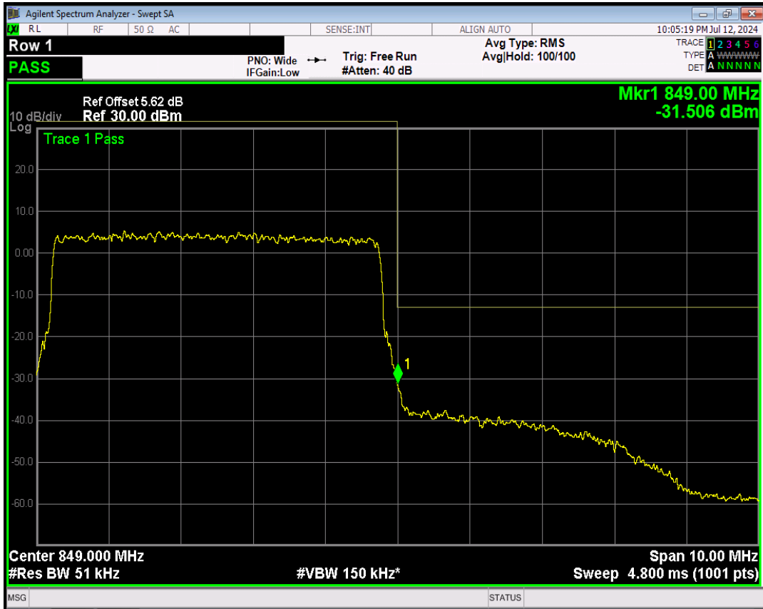
Band5 16QAM BW=5MHz Channel=20625 RB Size=25 Position=#0
