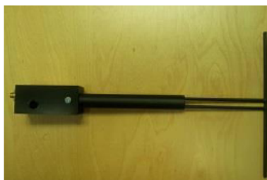
Figure 1 – MVG COMOSAR Validation Dipole
