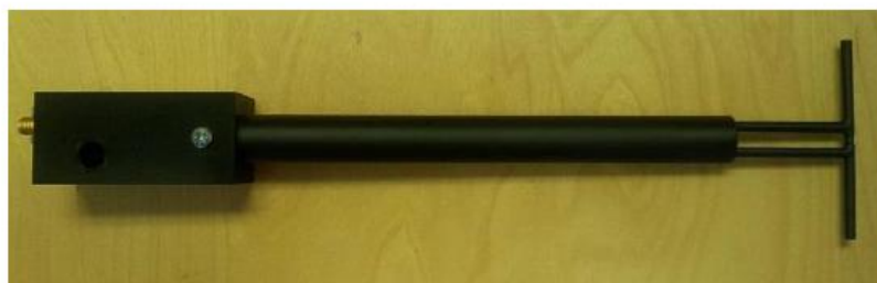
Figure 1 – MVG COMOSAR Validation Dipole
