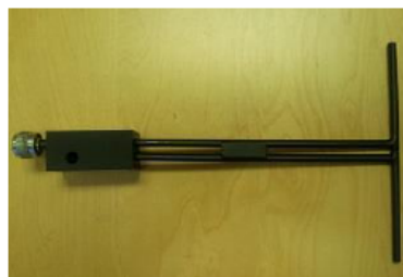
Figure 1 – MVG COMOSAR Validation Dipole
