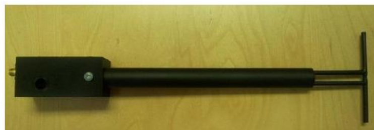
Figure 1 – MVG COMOSAR Validation Dipole
