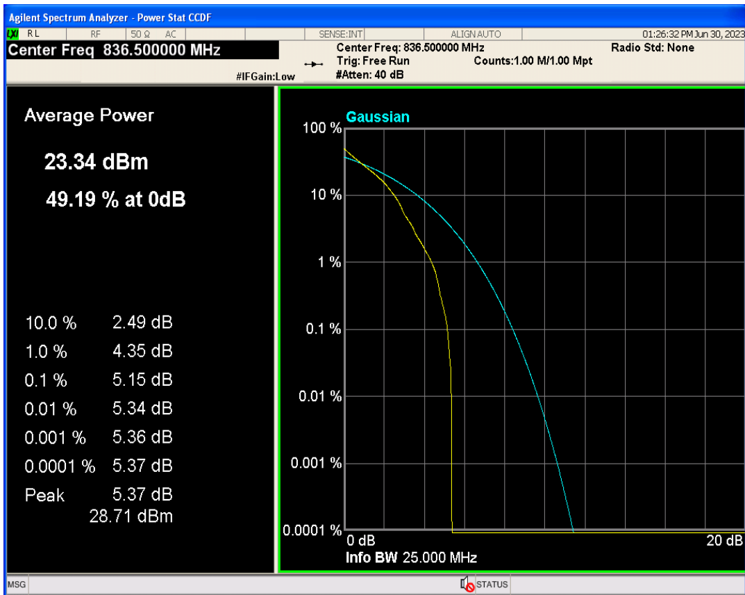
Band5 16QAM BW=1.4MHz Channel=20525 RB Size=1 Position=#0
