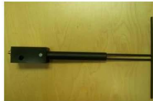
Figure 1 – MVG COMOSAR Validation Dipole
