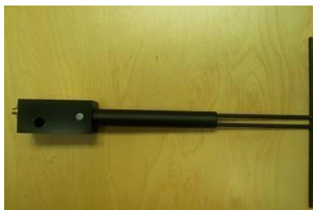
Figure 1 – MVG COMOSAR Validation Dipole
