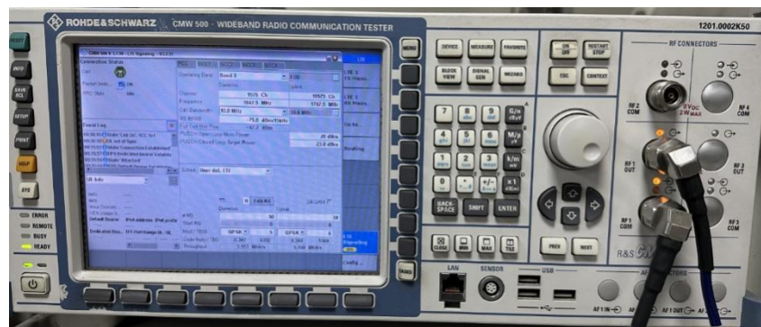
CMW 500 (2G/3G/4G Test Equipment)
