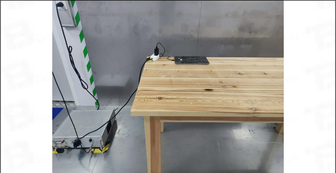
Conducted Emission at AC power line
