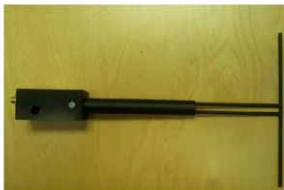
Figure 1 – MVG COMOSAR Validation Dipole
