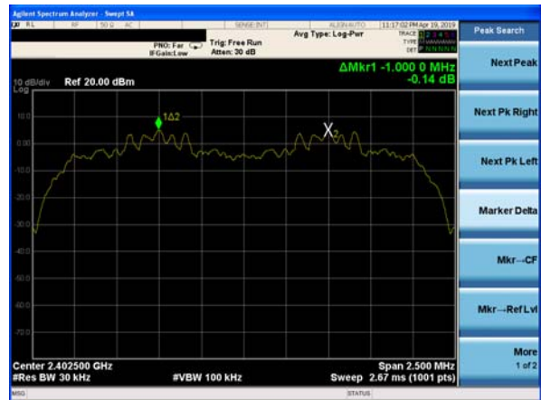
(2Mbps) Channel Separation plot on channel 39-40
