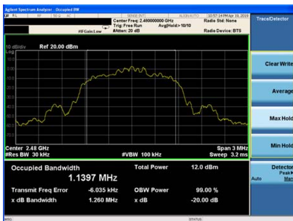
20dB Bandwidth plot on channel 78 (3Mbps)
