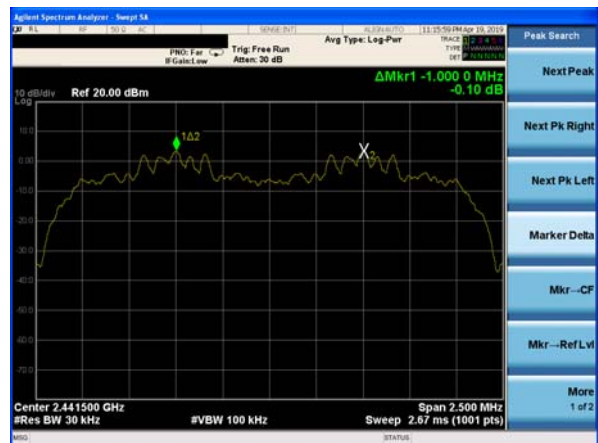
(2Mbps) Channel Separation plot on channel 77-78
