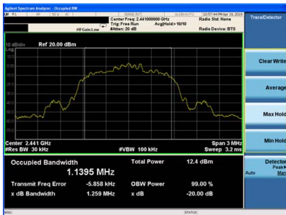
20dB Bandwidth plot on channel 78 (3Mbps)
