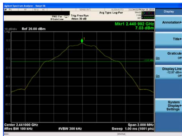
GFSK on channel 39
