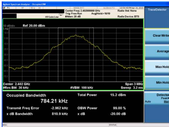
20dB Bandwidth plot on channel 39 (1Mbps)
