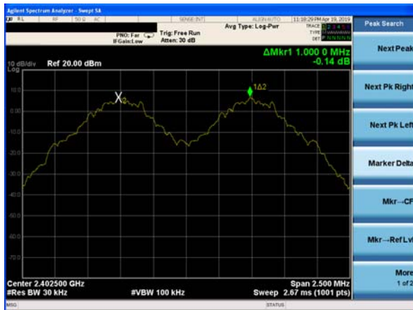
(1Mbps) Channel Separation plot on channel 39-40
