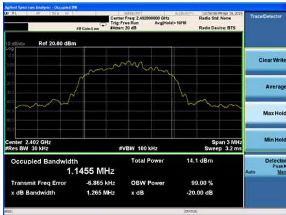
20dB Bandwidth plot on channel 39 (3Mbps)
