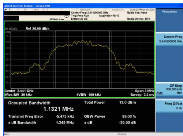
20dB Bandwidth plot on channel 78 (2Mbps)
