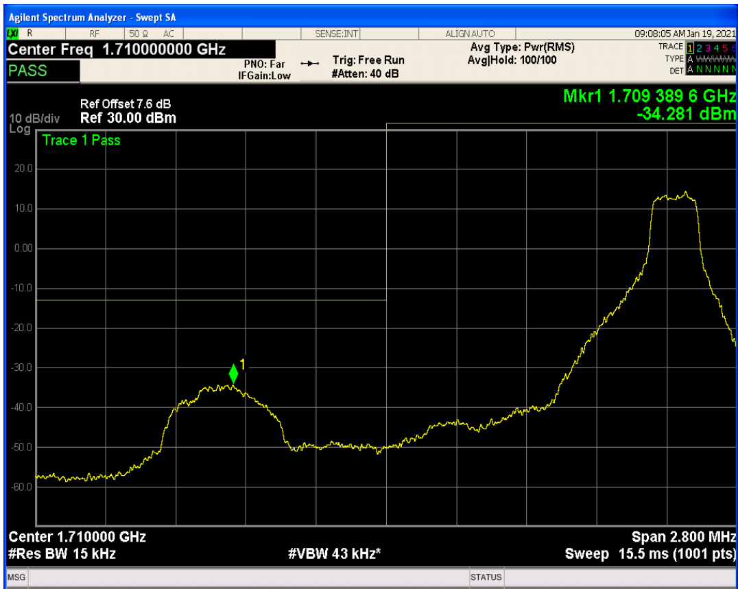
Band4 QPSK BW=1.4MHz Channel=19957 RB Size=6 Position=#0
