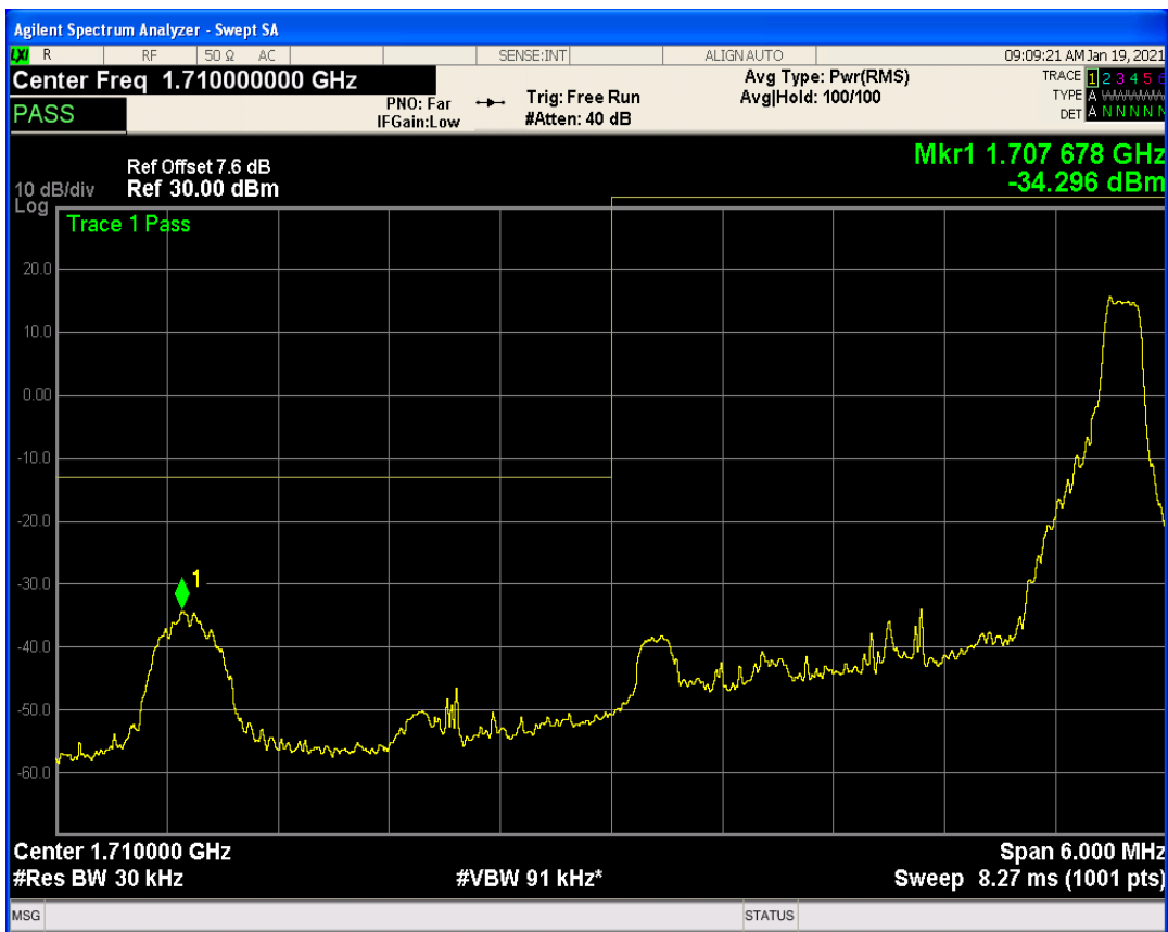
Band4 QAM16 BW=3MHz Channel=19965 RB Size=15 Position=#0
