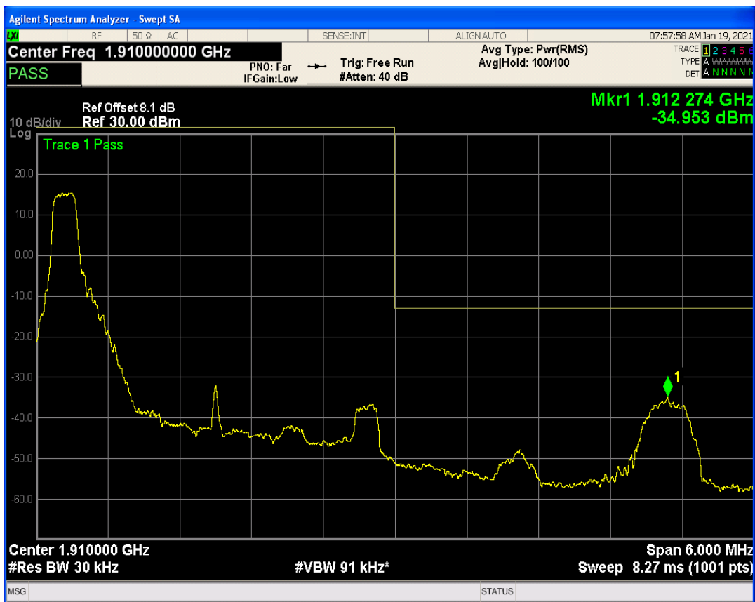
Band2 QPSK BW=3MHz Channel=19185 RB Size=15 Position=#0
