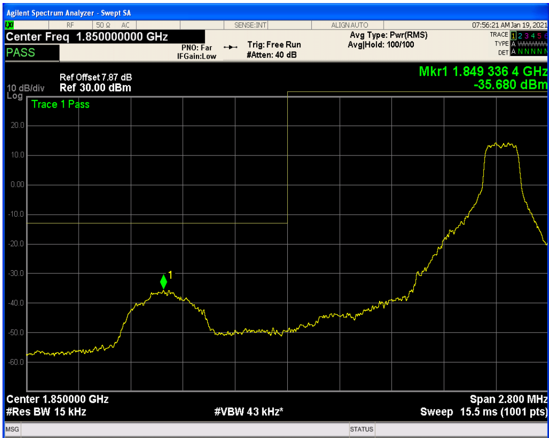
Band2 QAM16 BW=1.4MHz Channel=18607 RB Size=1 Position=#0
