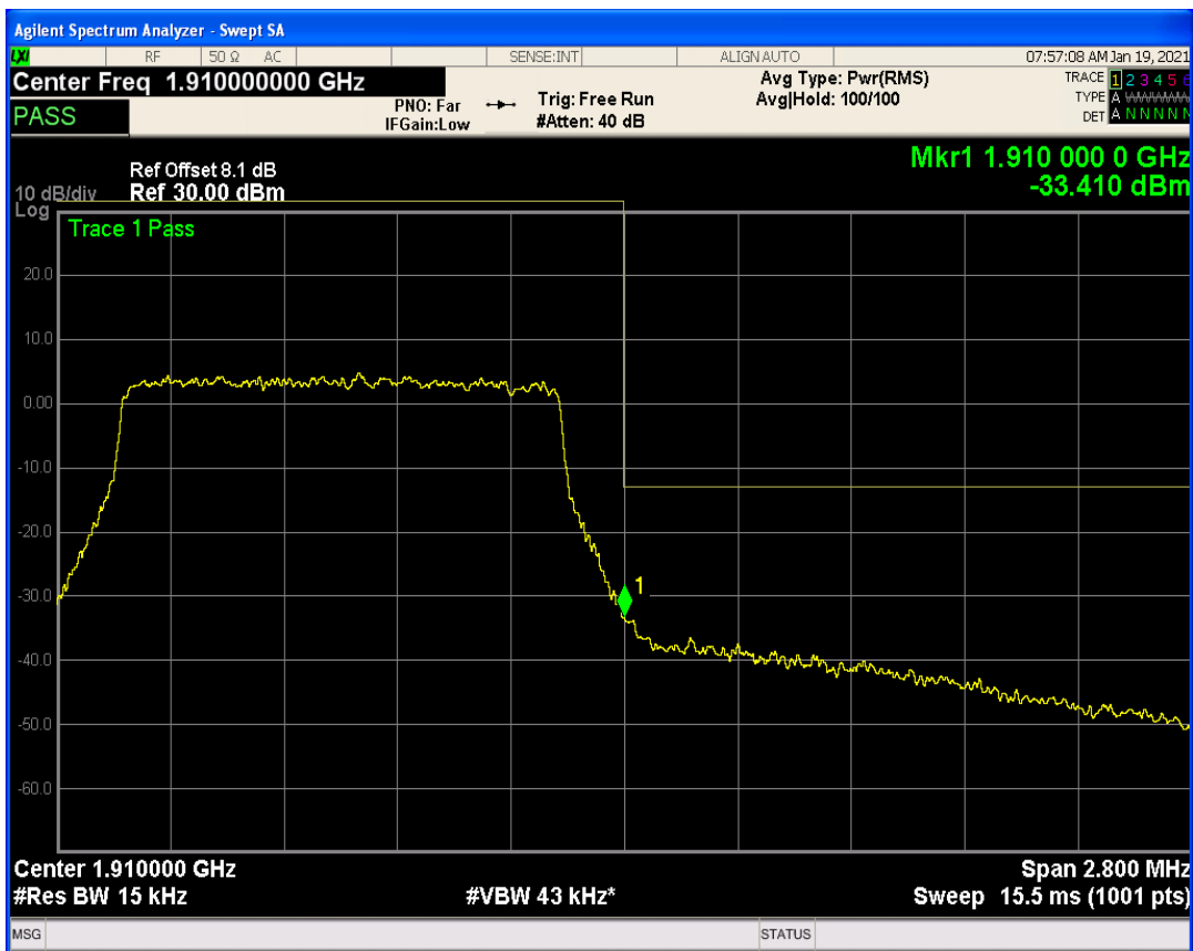
Band2 QPSK BW=3MHz Channel=18615 RB Size=1 Position=#Max
