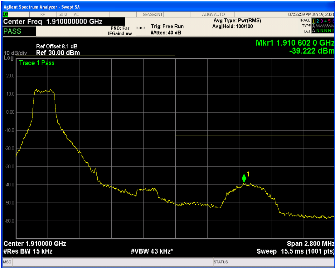
Band2 QAM16 BW=1.4MHz Channel=19193 RB Size=1 Position=#Max
