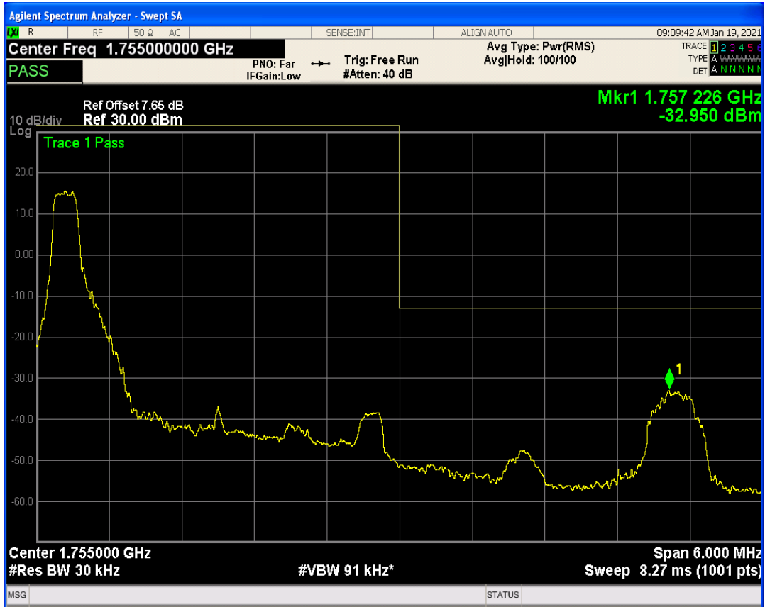
Band4 QAM16 BW=3MHz Channel=20385 RB Size=1 Position=#Max
