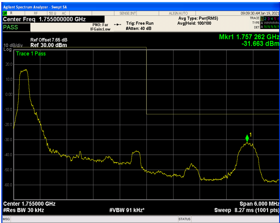
Band4 QPSK BW=3MHz Channel=20385 RB Size=1 Position=#Max
