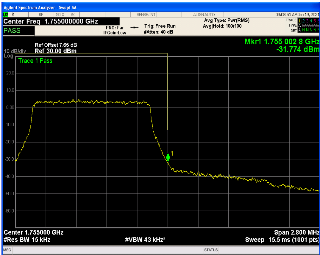
Band4 QPSK BW=3MHz Channel=19965 RB Size=1 Position=#Max
