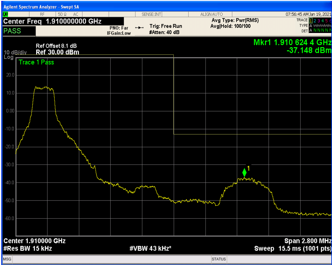
Band2 QAM16 BW=1.4MHz Channel=18607 RB Size=6 Position=#0
