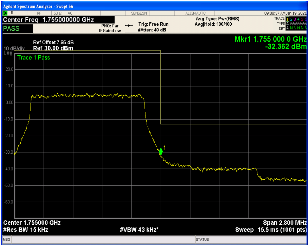
Band4 QAM16 BW=1.4MHz Channel=20393 RB Size=1 Position=#Max
