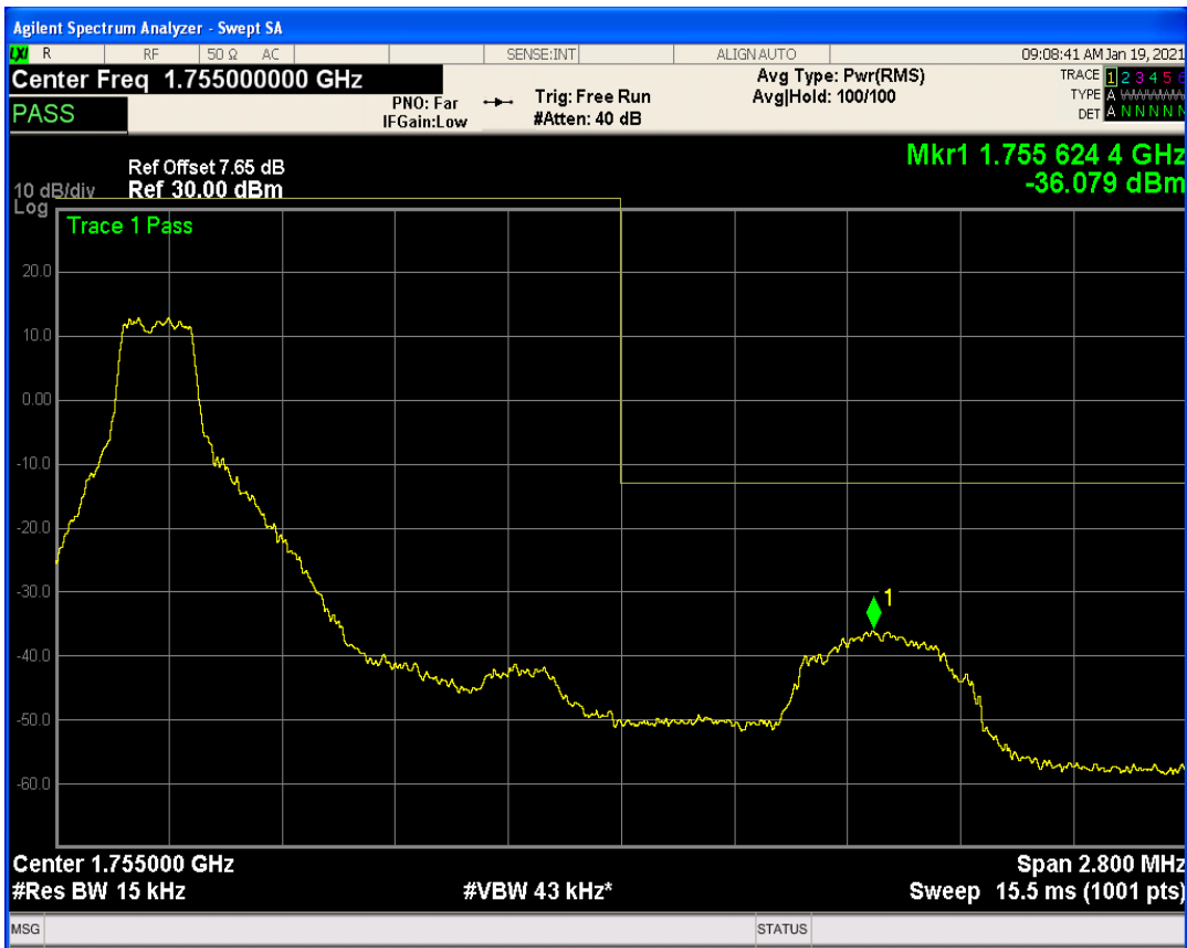
Band4 QPSK BW=1.4MHz Channel=20393 RB Size=6 Position=#0
