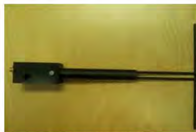
Figure 1 – MVG COMOSAR Validation Dipole
