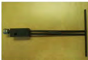
Figure 1 – MVG COMOSAR Validation Dipole
