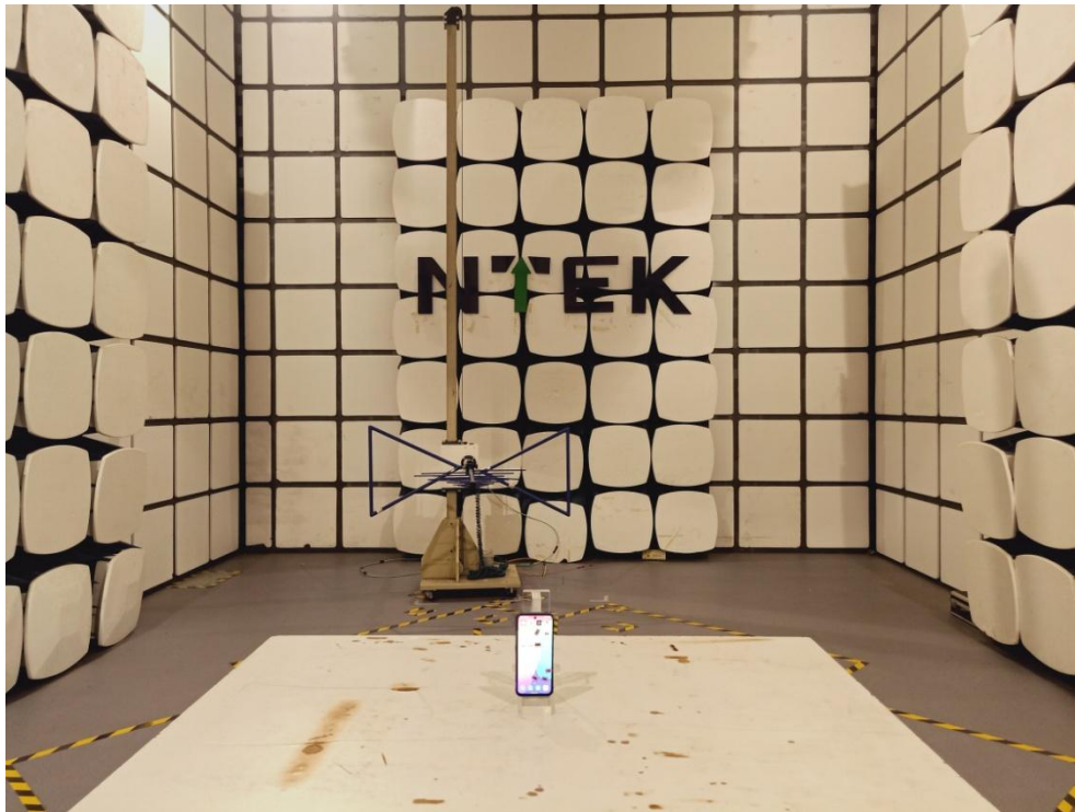
Radiated Measurement Photos(30MHz~1GHz )
