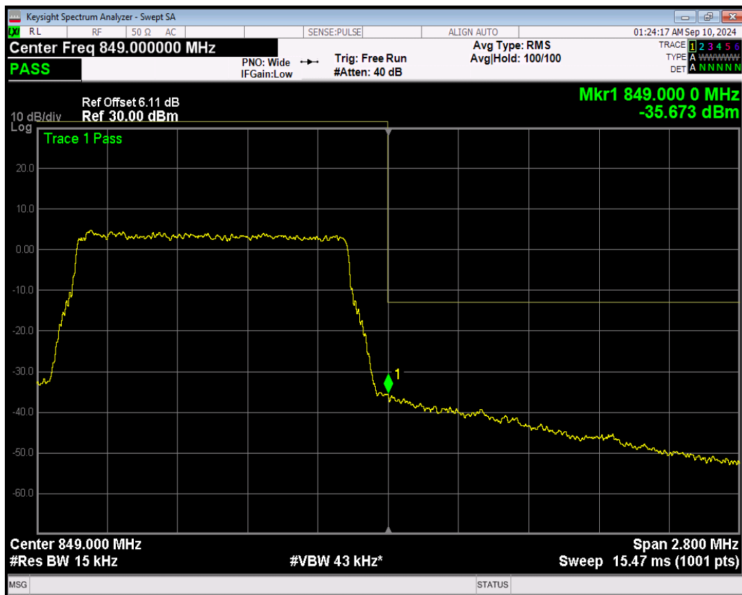
Band26(824-849) 16QAM BW=1.4MHz Channel=27033 RB Size=1 Position=#0
