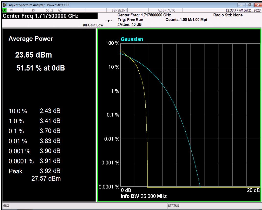
Band4 16QAM BW=15MHz Channel=20025 RB Size=1 Position=#0
