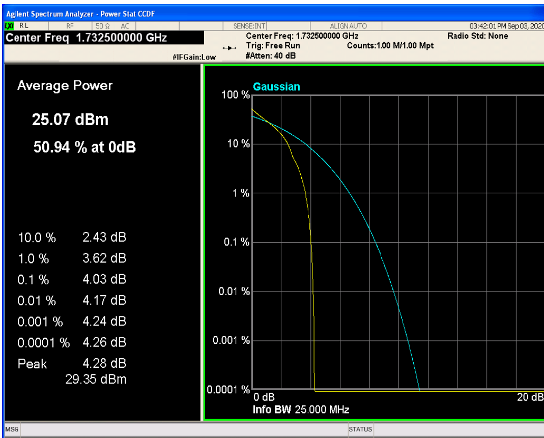
LTE Band5 QPSK BW=1.4MHz Channel=20525 RB Size=1 Position=#0
