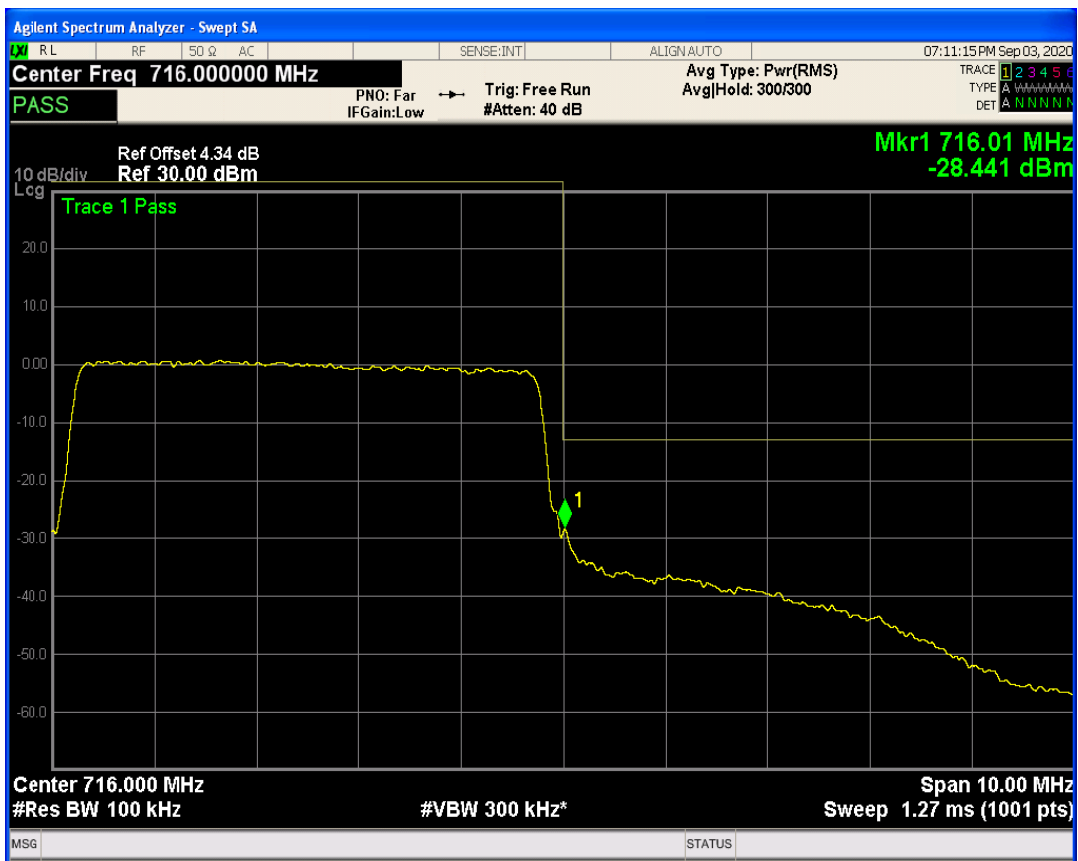
LTE Band12 QPSK BW=10MHz Channel=23060 RB Size=1 Position=#Max
