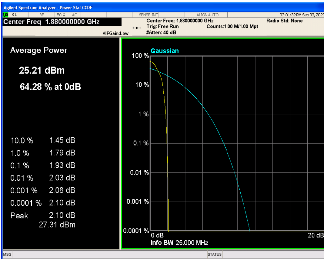
LTE Band2 QAM16 BW=15MHz Channel=18900 RB Size=1 Position=#0
