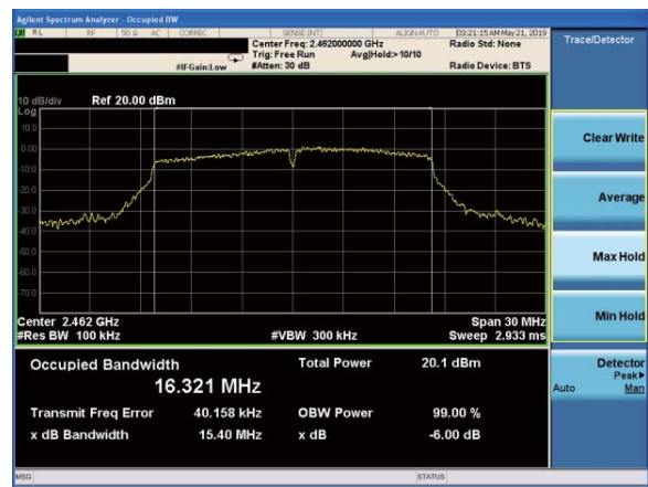
(802.11g) 6dB Bandwidth plot on channel 11
